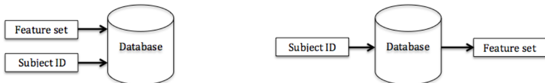
Figure 2.2: Enrolment (left) and lookup phases (right) of a database. Subject lookup can only be done after enrolment of that subject.
