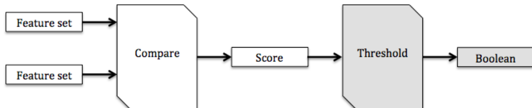
Figure 2.3: Comparing the feature sets of the target and query. The thresholding step is optional.
