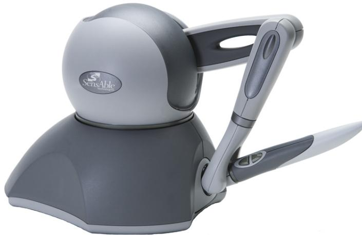
Figure 5.8: The Sensable Phantom Omni
