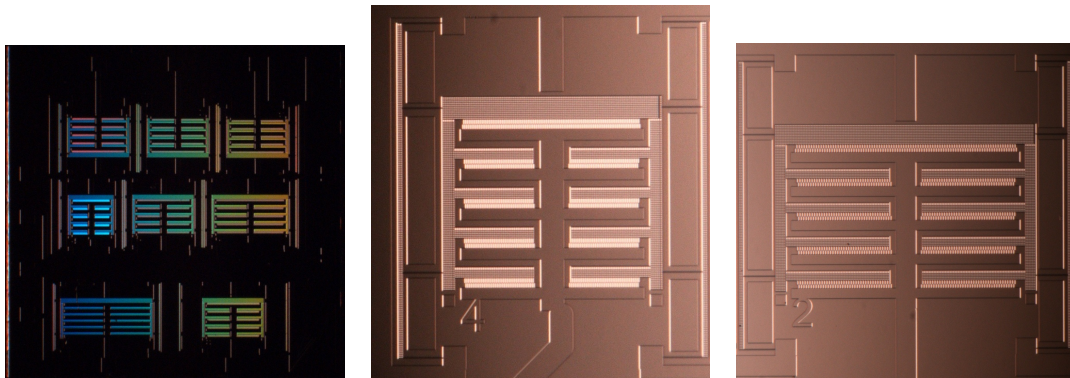
(a) Photo of the FF2 chip which was held under an angle under a microscope. The grids on the translators reflect different colours light differently. (b) Photo of the FF-SG-2 design. The photo was taken with a microscope. (c) Photo of the FF-LF2 design. The photo was taken with a microscope.
