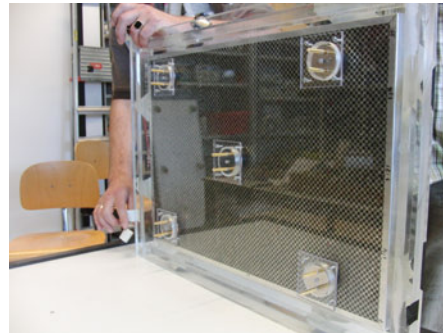
Figure 4.9: Back view of the panel, with the five magnets
