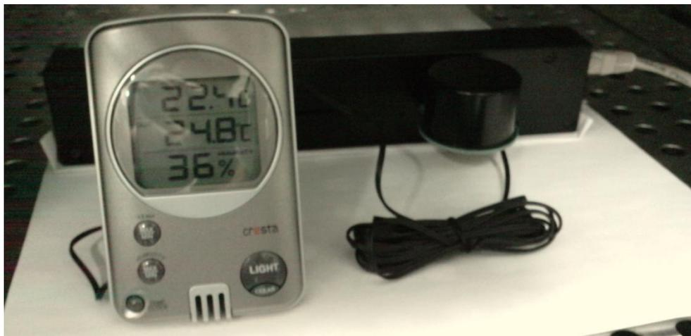
Figure A1. Measurement of the chip's temperature. A hood was used to cover the chips.
