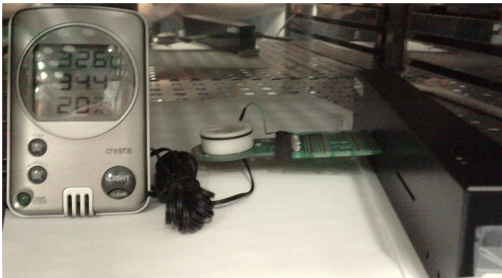
Figure A2. Measurement of the chip's temperature. No hood was used to cover the chips and the PCB extension cable was used to provide an external reference electrode.
