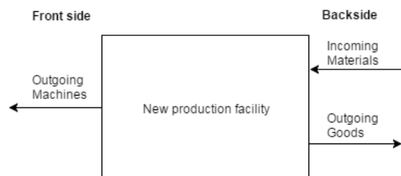
Figure 4.1: Formulated drop-off and pick-up points As there are no restrictions (e.g., route of transportation), this configuration offers the greatest flexibility for positioning the necessary resources.
