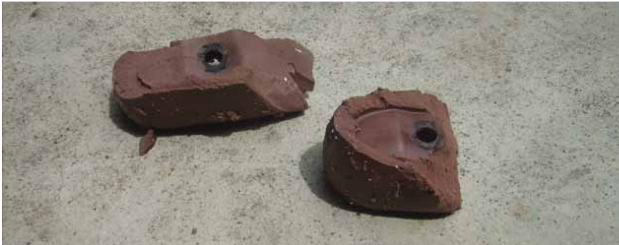
Figure 5: Two decaying ICRC feet.
