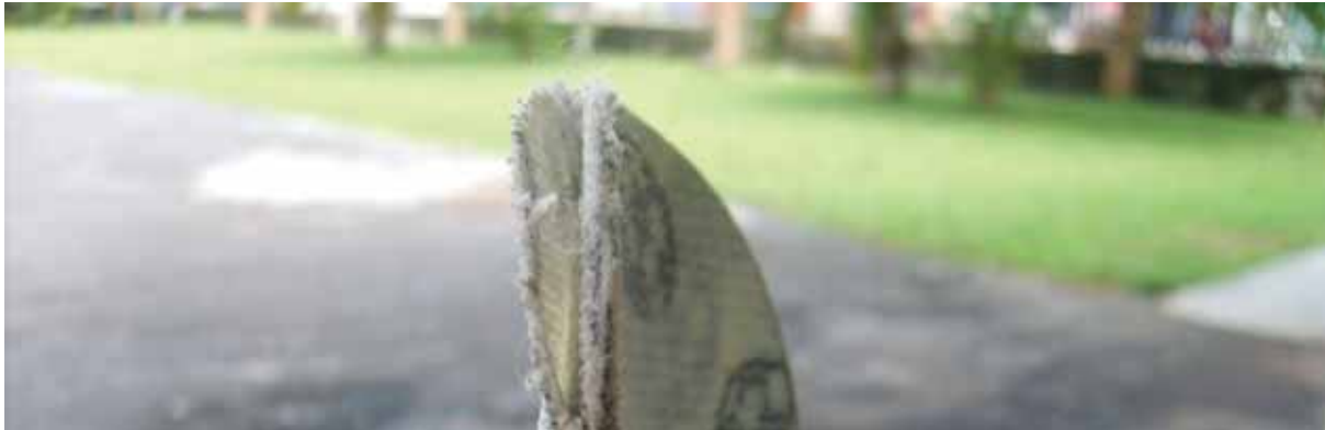
Figure 32: The lateral condyle of one socket split in half. Clearly the two different layers did not adhere properly to each other.
