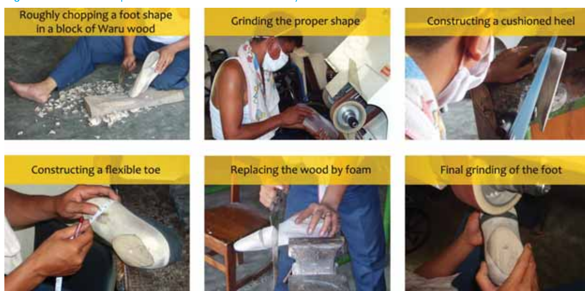
Figure 4: Production steps of the artificial foot constructed by Mr Tamba.
