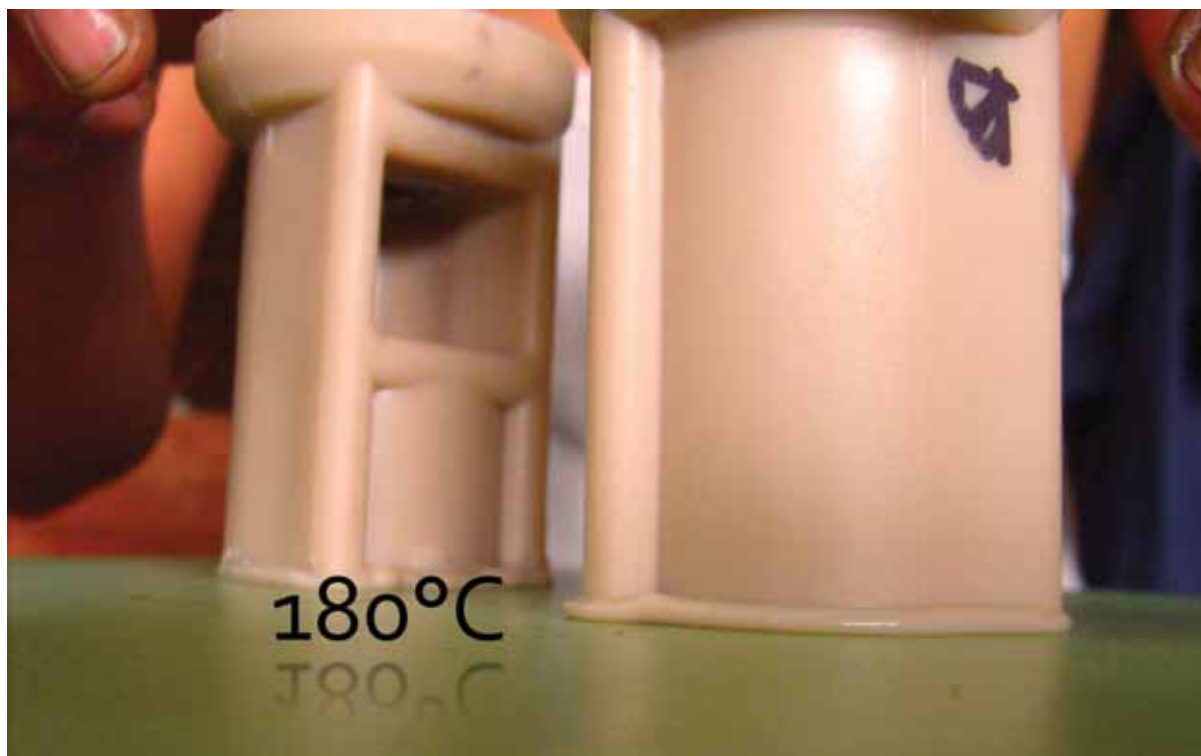
Figure 7: The two pipes of the ICRC system are cut at the right length and placed on a plate of 180°C. The polypropylene slightly melts and acts as glue when the pieces are pressed together.
