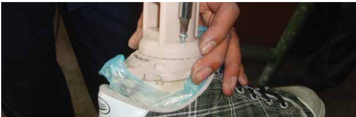
Figure 33: A screw through the convex and concave ICRC components is added for extra strength.
