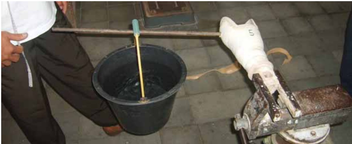
Figure 27: The torsion strength of the connection between the synthetic cast tape and the ICRC Cup is at least 60 Nm.
