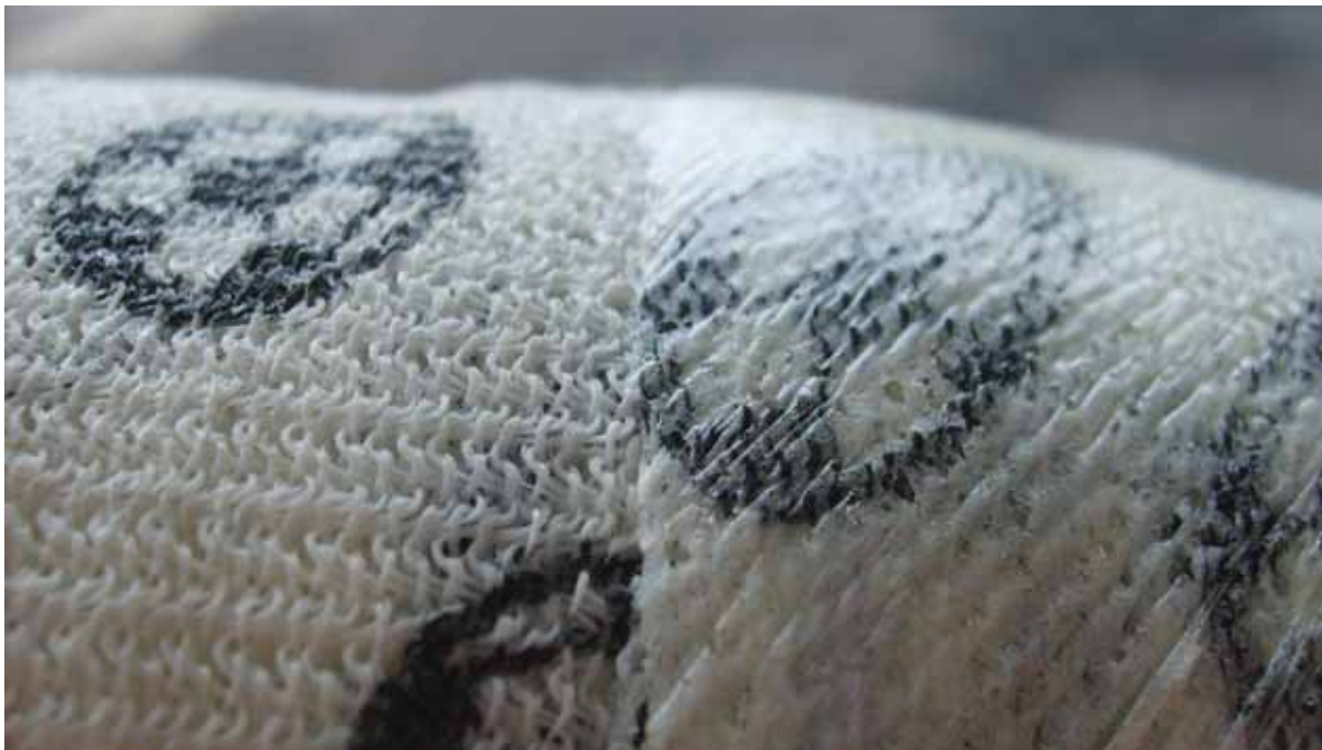
Figure 22: Close-up photo of a socket made with Delta Cast® Prints. First the socket was wrapped with low to moderate tension which resulted in a rather rough surface (left). Then this socket was wrapped with an extra layer, this time wrapped with high tension (right). Notice the stretched football print on the right and the smoother surface.
