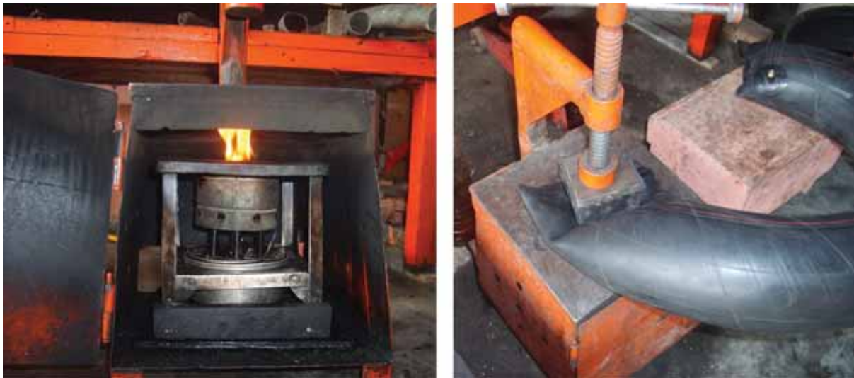
Figure 31: With the advanced technology of high temperature (left) and high pressure (right) a car tube can be 'glued' together.
