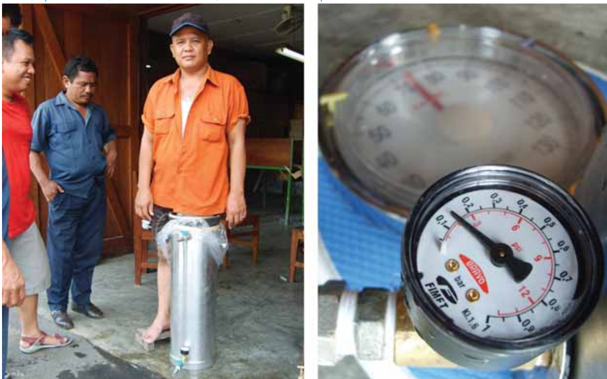
Figure 28: (left) Subject M standing in the PCAST. (right) With an added weight of 41,5 kg on a stump with a diameter of 13 cm, a pressure of 0,15 bar was measured, 105 % lower than expected.
