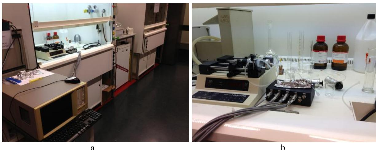
*Fig. 10 Photographs showing the measurement setup: a) the fume hood with cables coming in from the Keithley 4200 SCS, b) the pump on the left, and measurement box in the center with a sample.*
