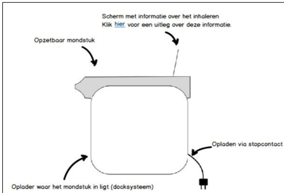
**Figure 25.** Screenshot: side view mouthpiece attached to the dock station
