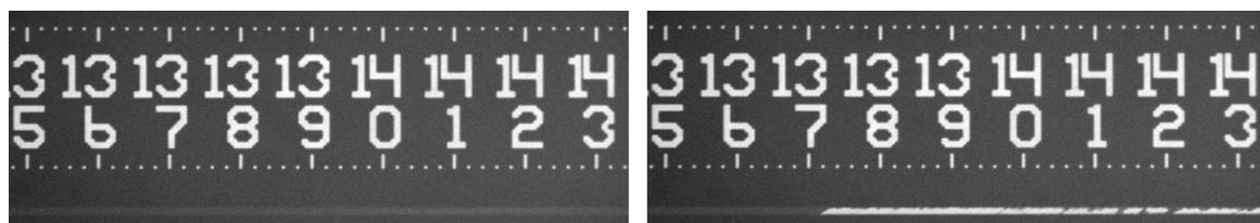
Figure 3.6: A cavitation event. In this case the low conductivity fluid is drained to the right. The difference between the two shots is one frame of 0.2s. The front remains intact at 13.72mm. The front may not be the same as the cavitation position; this has to be verified by checking the theoretical position of the front vs. the cavitation position and time.
