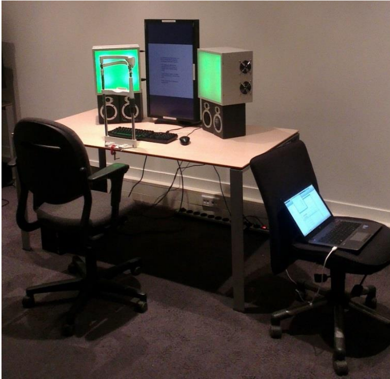
Figure 14. Experimental setup for experiment 3. The task was carried out on the vertically oriented screen on the table, while the led cubes were run using the laptop computer on the right. In this photo, luminance levels were increased to improve the visibility of the setup. During the experiment, the light was set to an illuminance of 7 lx.
