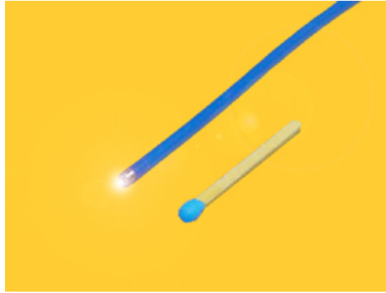
Figure 4.10: The O2C probe, microprobe with a diameter of 2.6 mm compared with the size of a match. [18]
