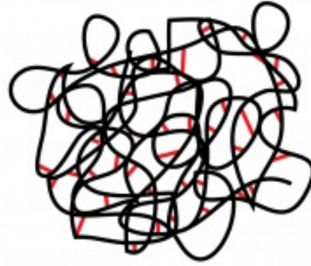
Figure 6.6.: Artists' conception of a cross-linked polymer. The black line represents the polymer chain, and the red bars the points where the cross linkages are made [13]
