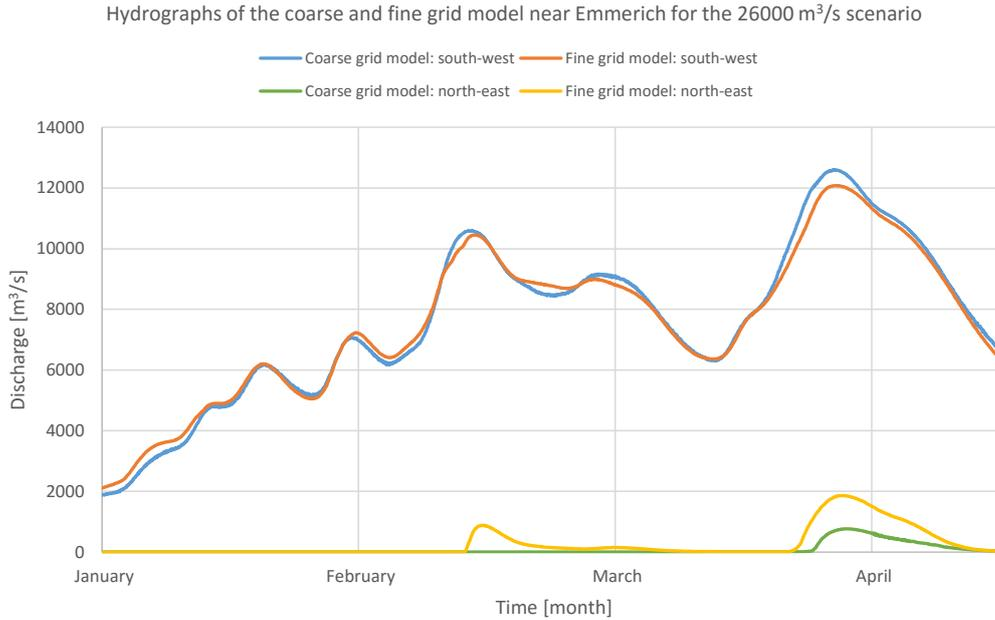
Figure 18: hydrographs of the coarse and fine grid model at the south-western and north-eastern side of the high-lying grounds near Emmerich for the 26000 m<sup>3</sup>/s scenario. The locations are shown in figure 17.
