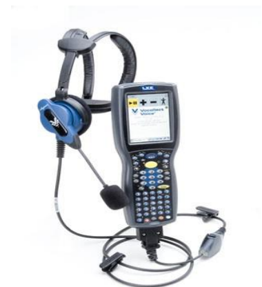
Picture 7.9 - Voice picking device Adapted from Inther, Retrieved May 3, 2016, from http://www.inther.nl/order-picking/voice-picking/ Copyright 2016.
