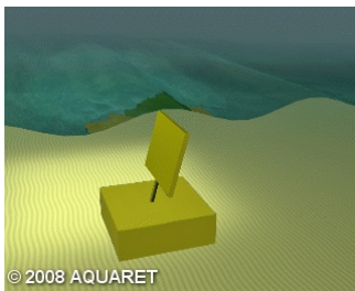
Figure 8.3: Oscillating wave surge device
