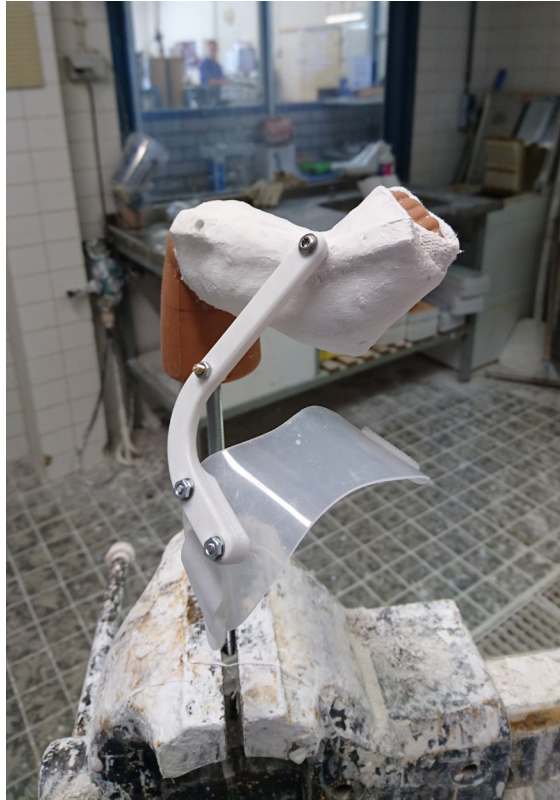
Figure 8.4 Photograph of the first prototype with the top part detached
