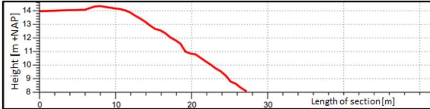
Figure 7: Current geometry of foreland on location west (Actueel Hoogtebestand Nederland, 2014)
