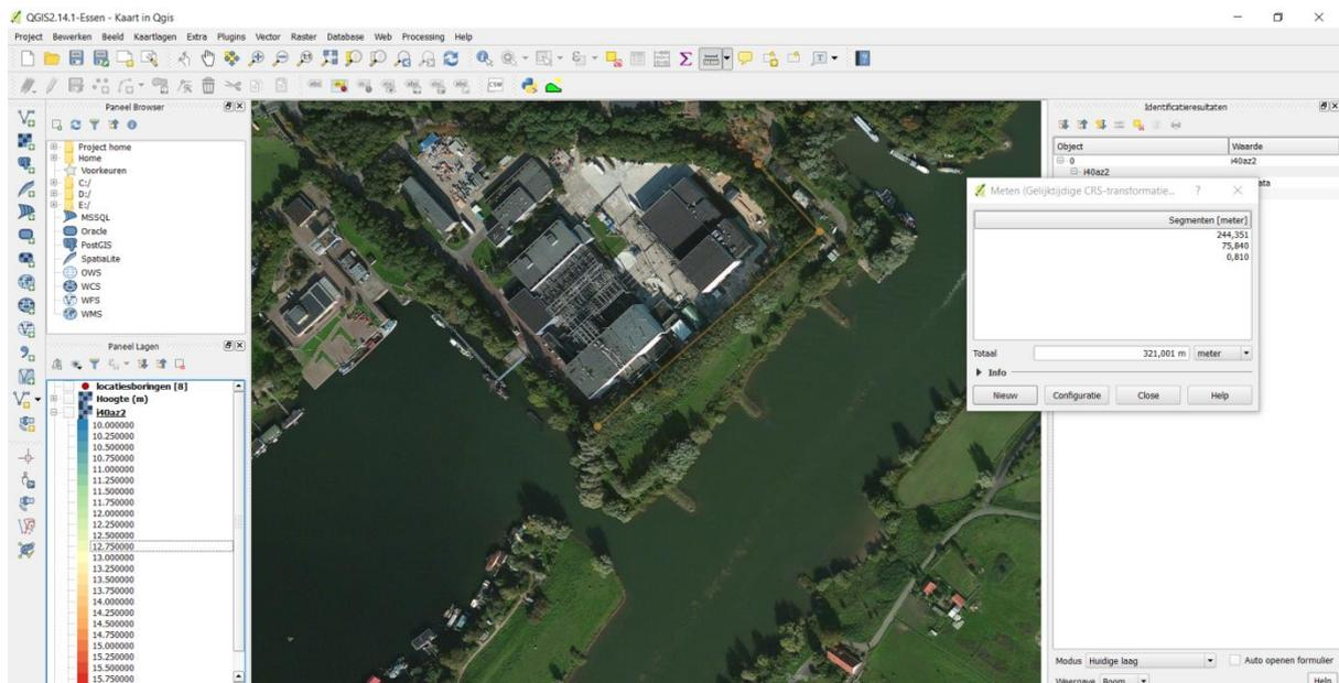
Figure 39: Determining lengths dike paths for dike on terrain of KEMA Laboratories
