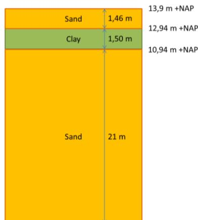
Figure 16: Soil structure for calculations for uplifting on terrain of KEMA Laboratories
