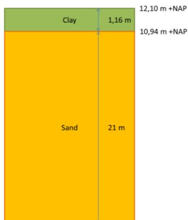
Figure 15: Soil structure for calculations for uplifting on the foreland
