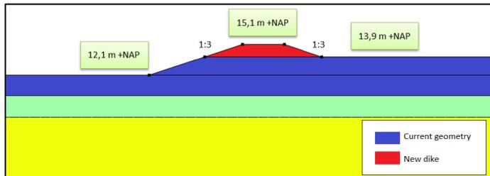
Figure 21: Dike on the terrain of KEMA Laboratories at location south
