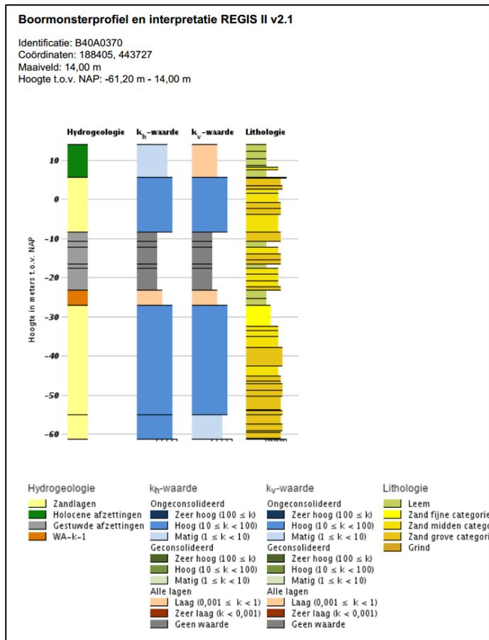
Figure 34: Deeper boring at location of KEMA Laboratories
