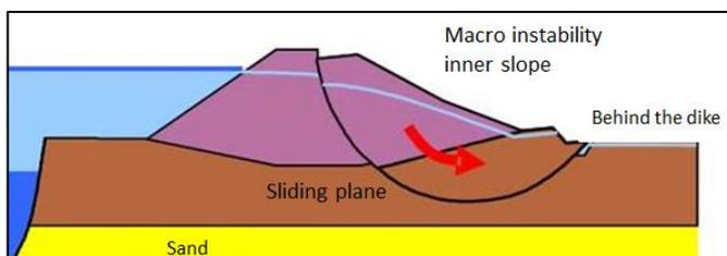
Figure 17: Macro instability of the inner slope
