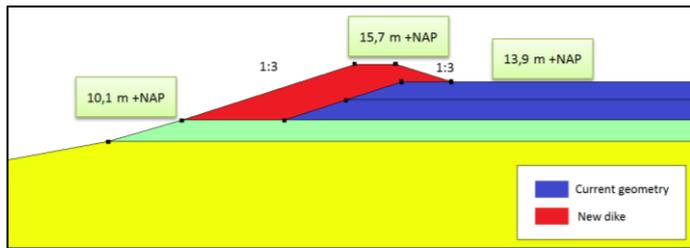
Figure 19: Dike partly on terrain of KEMA Laboratories at location west
