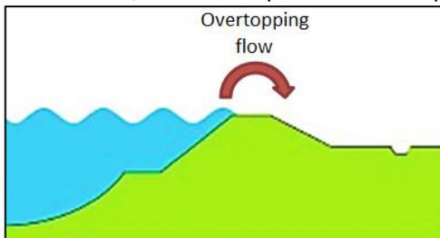
Figure 13: Overtopping flow over the dike
