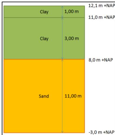
**Figure 18: Soil structure used for calculations of macro stability**
