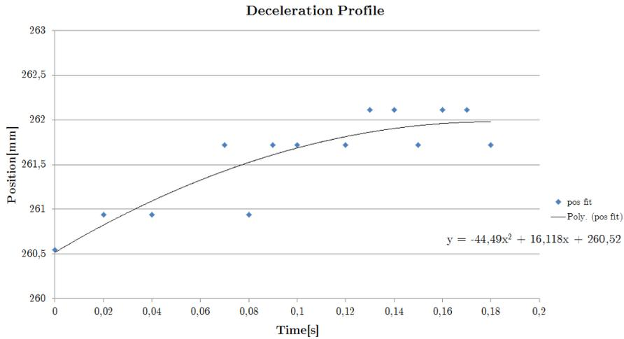
Figure 57: Maximum deceleration data of the Y-direction. The polynomial fit line is for the position. This fit line needs to be integrated twice to get the deceleration. Measurement without load in the cart.
