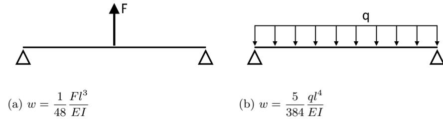
Figure 36: Two types of bending that are used to calculate the deformation of the spindle and also the linear guidance. (a) shows the deflection due to the force of the magnet and the weight of the magnet assembly. This is applicable for both the spindle and linear guidance as for the Y-table deflection calculations. (b) shows the deflection caused by the spindle's own weight. The sum of the deflections is the total deflection of the spindle.
