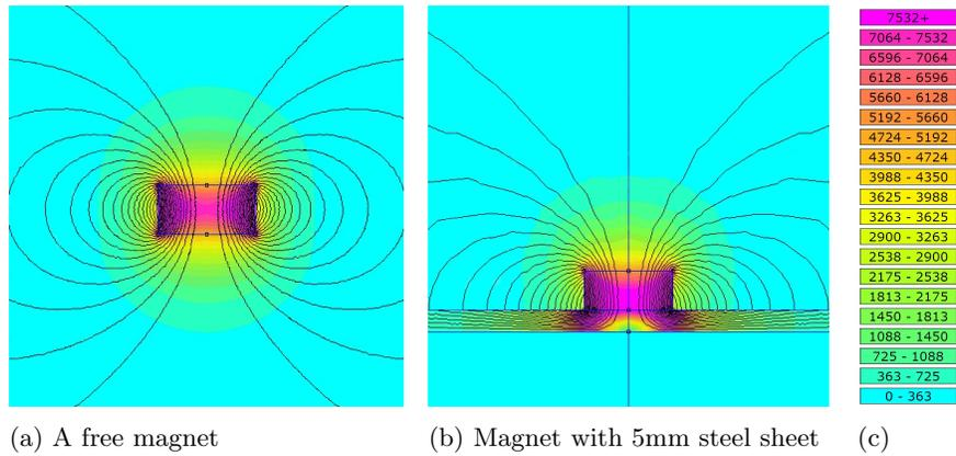
Figure 31: The difference in field strength and shape of the field between a) a free magnet and b) a magnet attached to a steel sheet that is thick enough to redirect all of the field through the sheet material. The colors in a) and b) correspond to the colors and field strengths in c). Pictures are made with K&J Magnetics' FEM calculator
