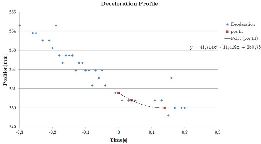
Figure 58: Maximum deceleration data of the Y-direction. The polynomial fit line is for the position. This fit line needs to be integrated twice to get the deceleration. Measurement with a load of 2kg in the cart.
