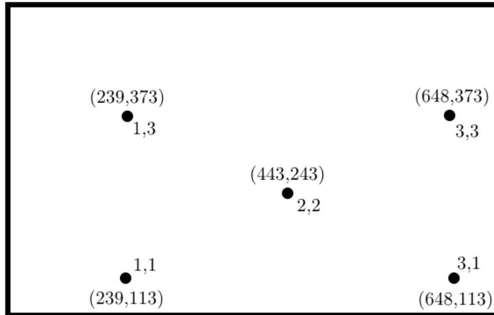
Figure 50: Positions of the measurement named '1,1', '1,3', '2,2', '3,1', '3,3' with the representing position in mm, i.e. (x[mm],y[mm]). Left bottom is the origin (0,0) and the top right (800,610).
