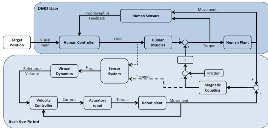
Figure 45: The control schematic of the final controller used for the XY-table.
