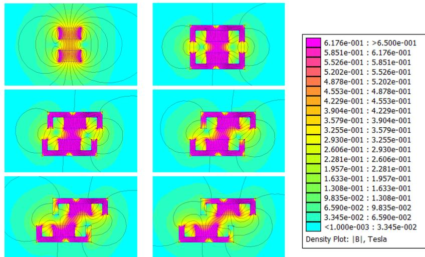
Figure 33: The difference in field between two magnets without and with magnetic shield (a & b), and the attractor field shapes of the magnets with shielding at center distances of 5mm (c), 10mm (d), 15mm (e), and 20mm (f). Colors are representing the field strengths in Tesla (g). The pictures are generated using Femm4.2 [55].
