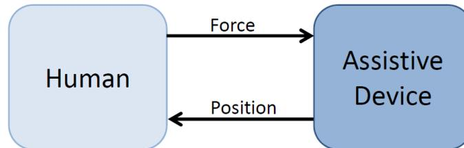
Figure 16: The interface of admittance control between the human and the controlled device. The device measures a force given by the user with it's sensors and the actuators make a movement according to this force.
