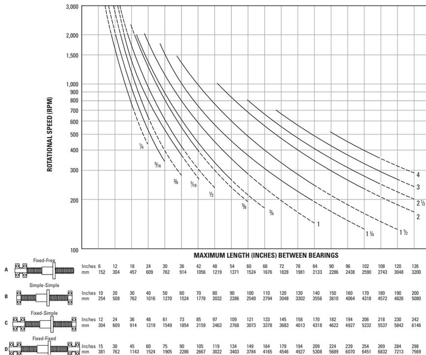
Figure 26: A typical critical spindle speed chart. The x-axis shows the unsupported length for different types of spindle support. A, B, C, and D represent the different types of support. The y-axis shows the rotational speed in revolutions per minute. The different root diameter are shown inside the graph underneath the lines and is given in inches.[40]
