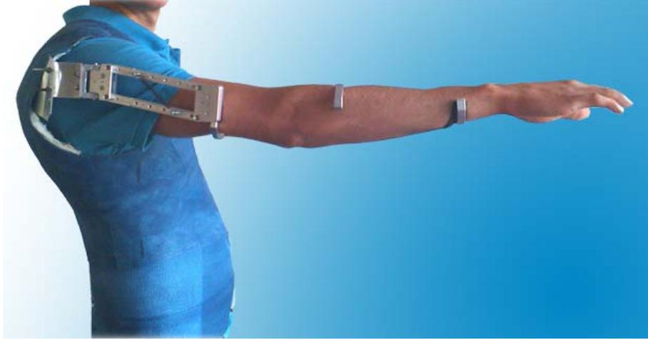
Figure 10: Prototype of the Flextension orthosis [24].
