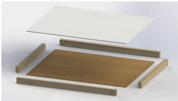
Figure 21: An exploded view of the table
