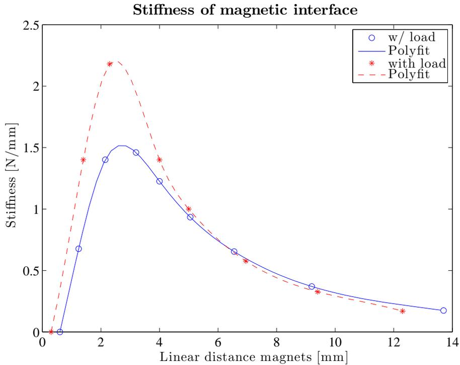
Figure 52: Lines of the stiffness with and without a load in the cart
