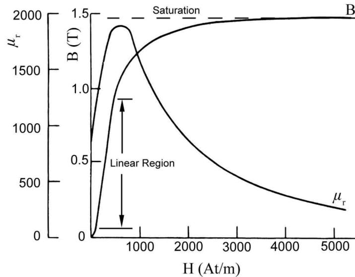
Figure 30: A typical relation between the relative permeability  $\mu_r$  and the magnetisation of ferromagnetic material [52].
