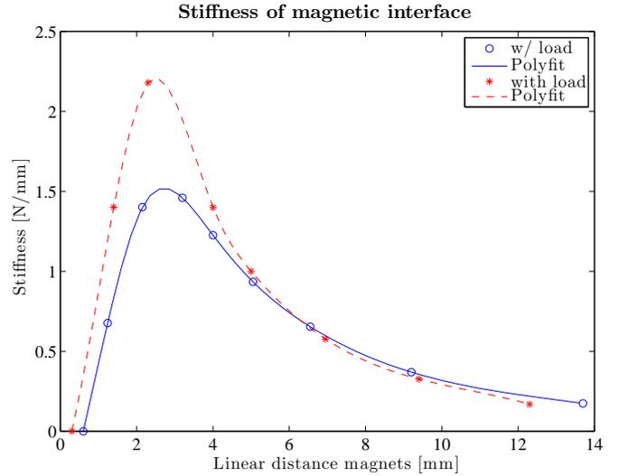
Fig. 7: The measured stiffnesses of the magnetic interface with (dashed red line) and without (solid blue line) a load of 2kg in the arm cart. The distance, is the horizontal distance between the two magnets.
