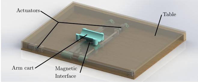
Fig. 5: A 3D CAD impression of the ActInArm concept. The table top and two wooden frame parts have been made transparent to make the actuators below the table top visible.
