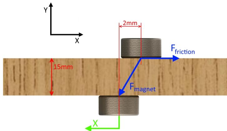
Figure 28: Relevant dimensions and forces acting on the magnets. The distance between the magnets in the y-direction is 15mm, the allowed dead-band is 2mm. The bottom magnet is moved in the x-direction and at the the maximum dead-band distance the x-component of the magnet force should be larger than the friction.
