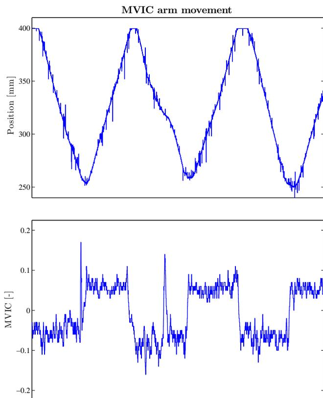
Fig. 8: The result of the validation. Plotted are the position of the end effector (top) and the normalized EMG signal, MVIC (bottom). Targets were positioned at 250mm and 400mm.
