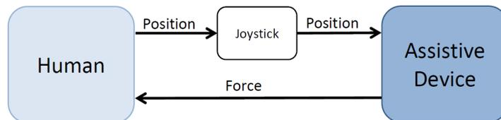
Figure 19: The user gives the input by moving a joystick. The joystick signal is then used to give a force back to the user.
