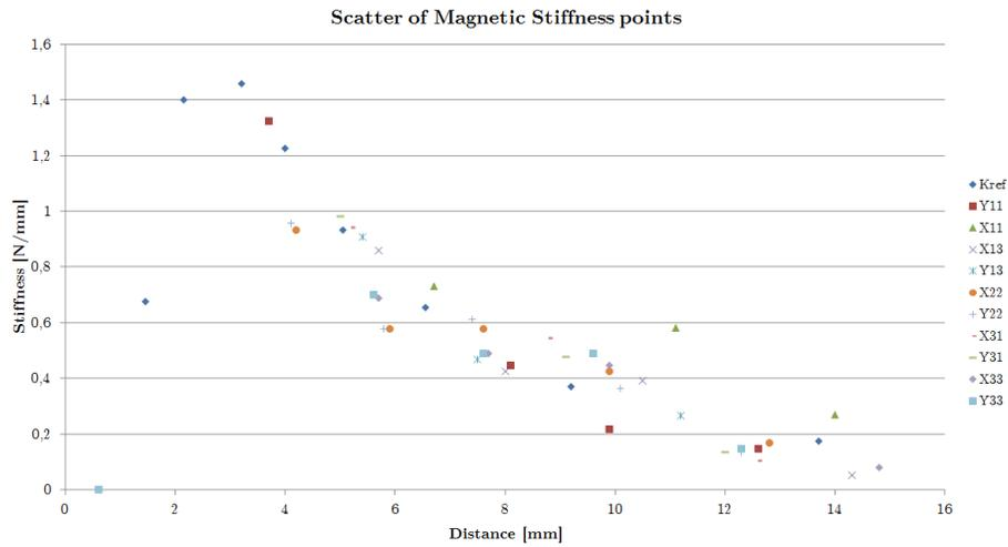
Figure 51: Scatter plot of all the stiffness at the different positions in the X and Y direction. Measured without a load in the cart
