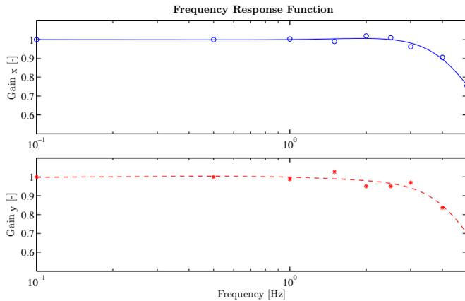
Fig. 9: The frequency response functions (FRF) of the assistive device in the X- and Y-direction ( $Gain_x$  &  $Gain_y$ ). The FRFs are the open loop functions from the desired velocity to the measured velocity and are measured without a load in the arm cart.
