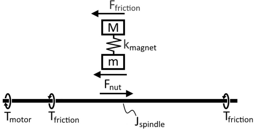
Figure 27: The forces the stepper motor needs to overcome. The spindle and the Y-table and arm with cart are decoupled, with  $F_{nut}$  being the interaction force between the two. The forces at the spindle include friction forces at the ball bearings of the spindle, acceleration of the spindle, and the nut force. The nut force includes acceleration of the Y-table and the arm with cart, and friction forces of the ball transfer units of the cart.
