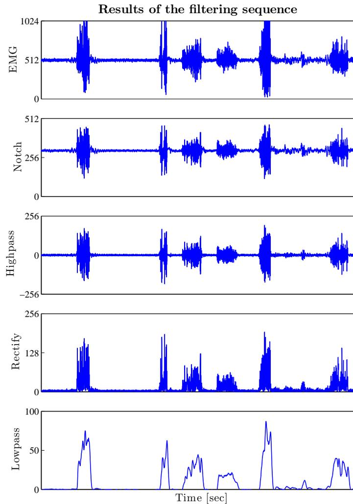
Figure 46: A typical result of EMG filtering. The peaks in the EMG graph are caused by muscle contractions.
