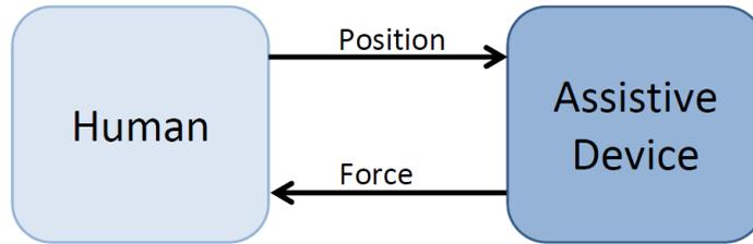
Figure 18: The interface of impedance control between the human and the controlled device. The device measures a position change with it's sensors and gives a force back to the user.
