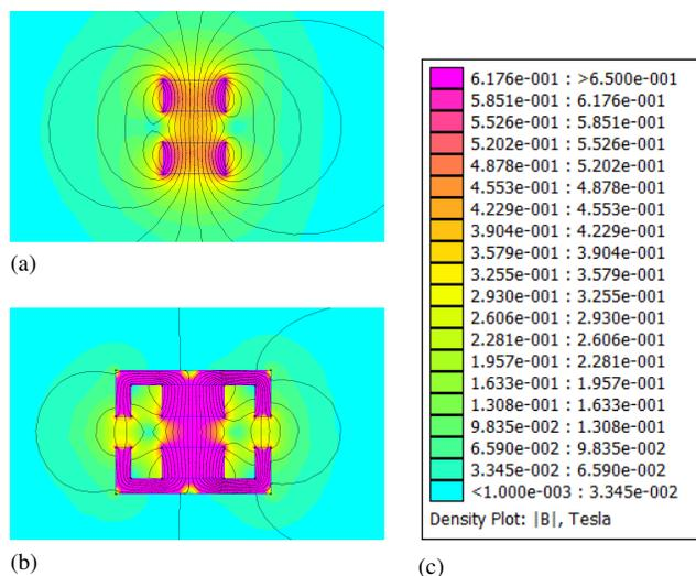
Fig. 4: An example of the difference in field shape and strength between two magnets without and with cups of high permeability material (a & b). Colors (c) are representing the field strengths [T]. The pictures are generated using Femm4.2 [16].
