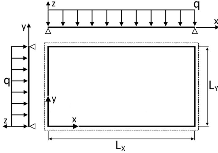
Figure 38: The situation of bending under own weight. All four edges are simply supported. 'q' represents the own weight of the HPL plate.
