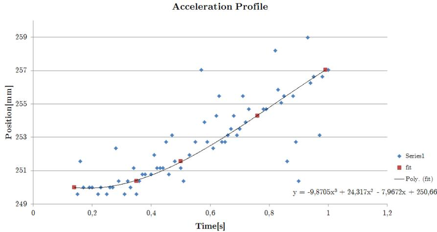
Figure 55: Maximum acceleration data of the Y-direction. The polynomial fit line is for the position. This fit line needs to be integrated twice to get the acceleration. Measurement with a load of 2kg in the cart.
