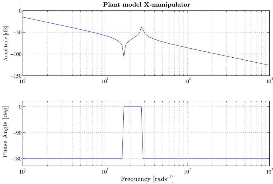
Figure 44: The Bode diagram of the reduced plant model of the XY-table. Both the rigid body mode and the mode of vibration can be seen clearly. In the magnitude plot the rigid body mode is the downward peak at 16.9 rad/s, the vibration mode the upward peak at 28 rad/s.
