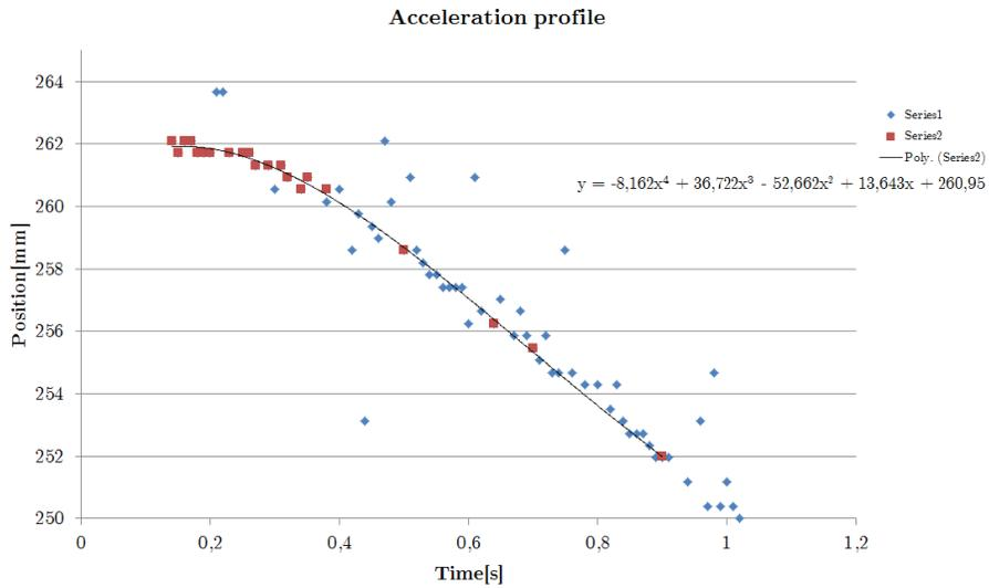
Figure 54: Maximum acceleration data of the Y-direction. The polynomial fit line is for the position. This fit line needs to be integrated twice to get the acceleration. Measurement without load in the cart.
