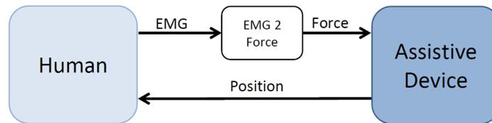
Figure 17: The interface of admittance control between the human and the controlled device. The device measures an EMG signal of the user's muscles. The EMG signal of the user's muscles is translated into a force and used to determine the desired movement of the actuators.
