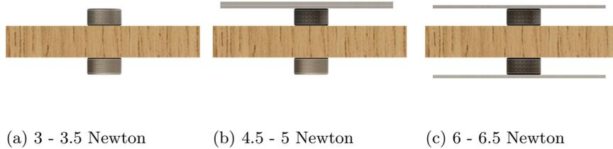
Figure 29: The three scenarios that were tested during the magnetic pull test. In subfigure a) the magnets were free. In subfigure b) both magnets have a 2mm steel sheet attached to them. In subfigure c) one magnet is free and the other has a 4mm steel sheet attached to it. The maximum horizontal forces up to the point where the two magnets still had interaction with eachother are stated underneath each subfigure.
