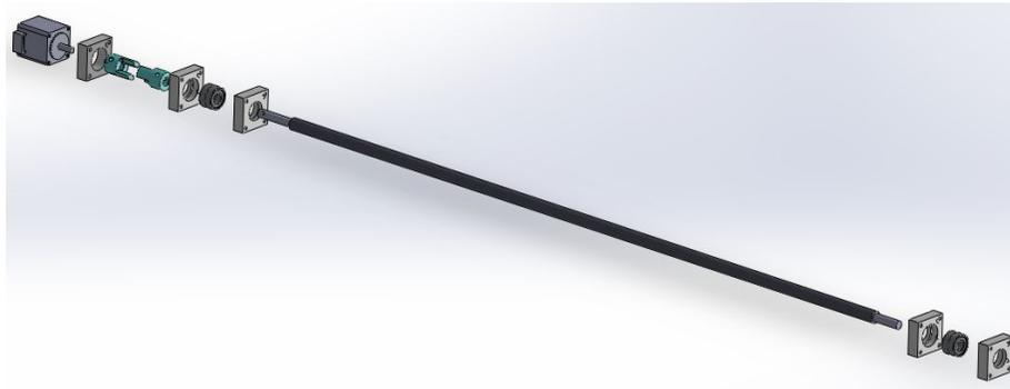
Figure 22: An exploded view of the manipulator for the x-direction
