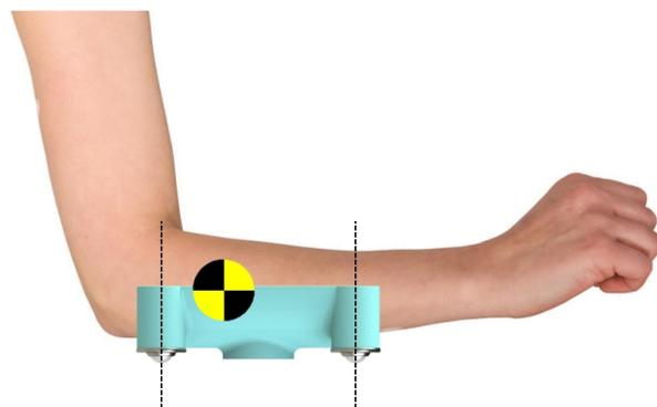
Fig. 3: The center of mass of the arm should be between the wheels of the arm cart (depicted by the striped lines).
