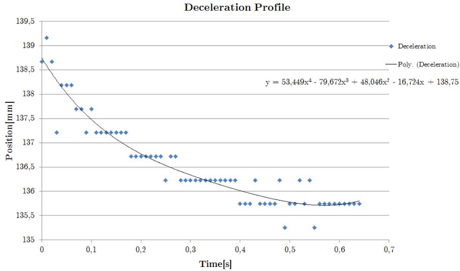
Figure 56: Maximum deceleration data of the X-direction. The polynomial fit line is for the position. This fit line needs to be integrated twice to get the deceleration. Measurement without load in the cart.
