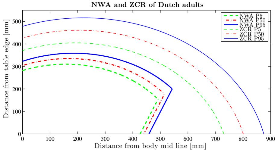
Figure 7: The normal working area (NWA) and zone of convenient reach (ZCR) over the table surface of the 5<sup>th</sup>, 50<sup>th</sup>, and 95<sup>th</sup> percentile of Dutch adult males.
