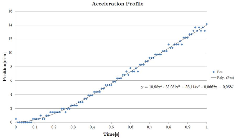
Figure 53: Maximum acceleration data of the X-direction. The polynomial fit line is for the position. This fit line needs to be integrated twice to get the acceleration. Measurement without load in the cart.
