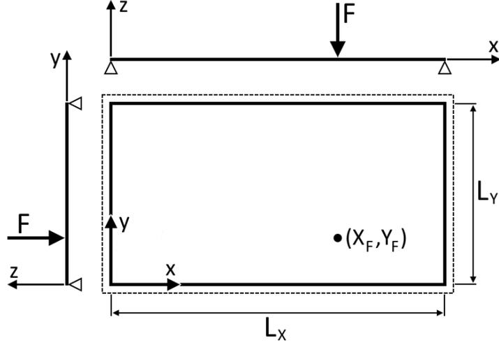
Figure 37: The situation of bending under the weight of the arm plus cart and the magnet force. 'F' represents the total force of the previous stated components. All four edges are simply supported.
