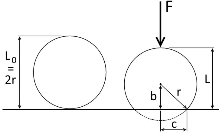
Figure 40: All the different parameters that are used in the derivation of the contact area formula.
