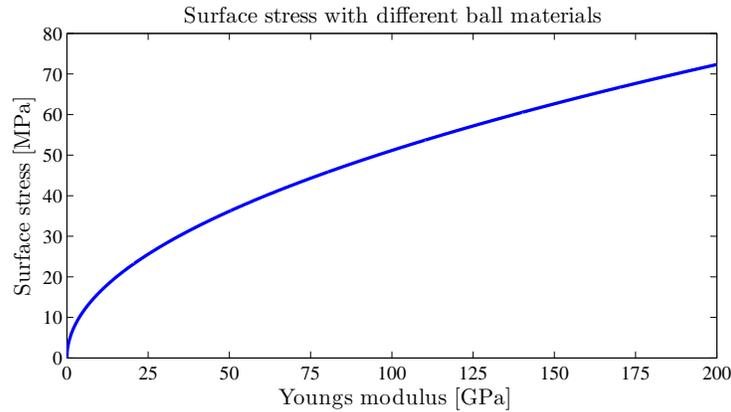
Figure 41: The stress at the table top surface for different materials
