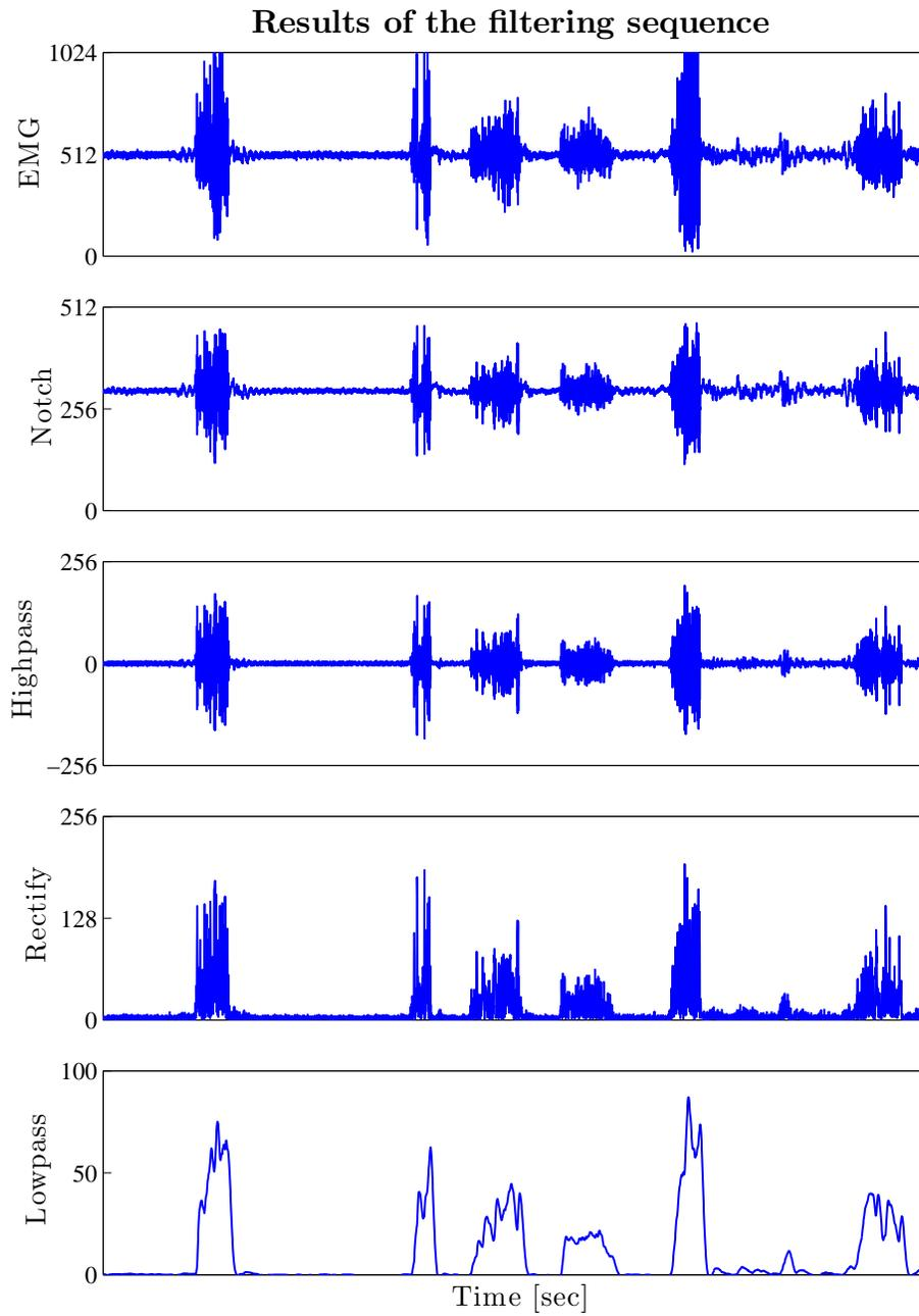
Figure 47: The filtered EMG signal from the raw input to the smoothed control signal.
