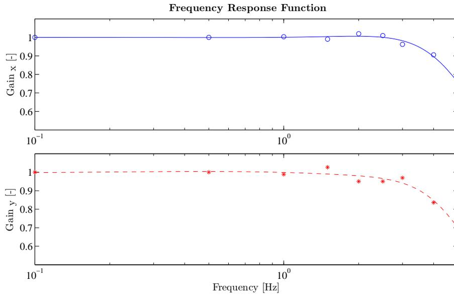
Figure 59: The frequency responses of the manipulator in the X- and Y-direction
