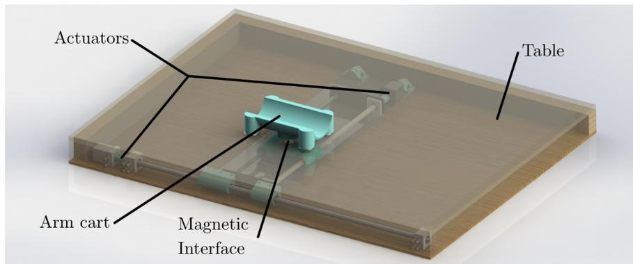
Figure 20: A 3D CAD impression of the final design of the XY-table concept. The table surface and two wooden frame parts have been made transparent to make the manipulator below the table surface visible. The parts are 1. The Table, 2. The Actuators, 3. The magnet assembly, and 4. The arm cart
