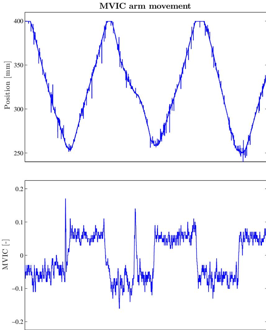
Figure 48: The result of the validation. Plotted are the position of the end effector (top) and the normalized EMG signal, MVIC (bottom). Targets were at 250mm and 400mm.
