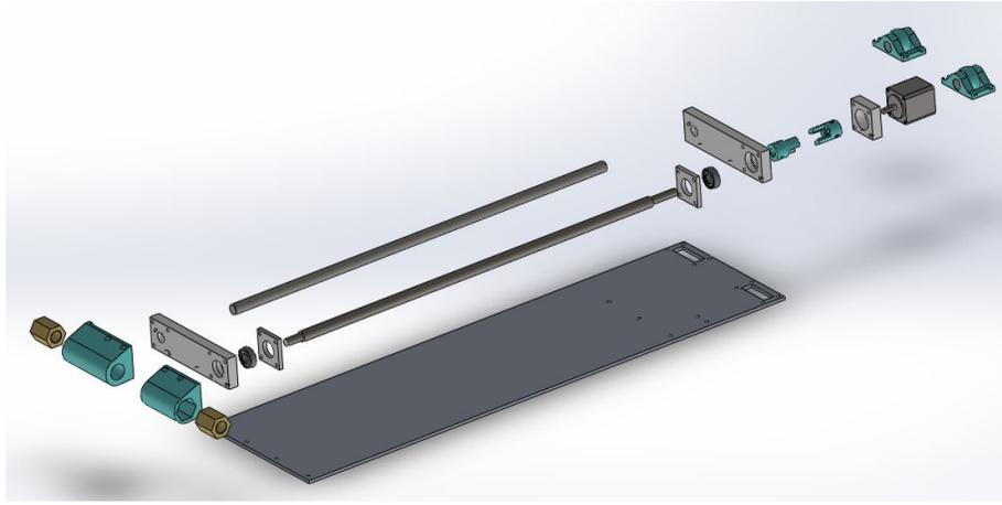
Figure 23: An exploded view of the manipulator for the y-direction
