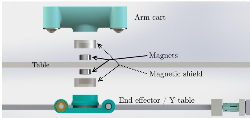
Figure 32: An exploded view of the magnetic interface. At both sides of the table top - the Arm cart and the Y-table side - there is a magnet with magnetic shield. With this interface movement of both parts is connected.
