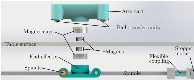
Fig. 6: A 3D CAD impression of the drivetrain of the ActIn-Arm prototype.
