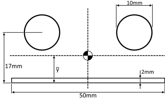
Figure 35: Cross-section of the Y-table, with the spindle and the guidance shaft being both  $\phi 10\text{mm}$  and the mounting plate below that has dimensions  $50\text{mm} \times 2\text{mm}$ .  $\bar{y}$  represents the distance between the neutral line and the bottom of the mounting plate.
