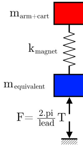
Figure 43: A simplified ideal model of the plant. The final model complies with the 'flexible transmission' model.
