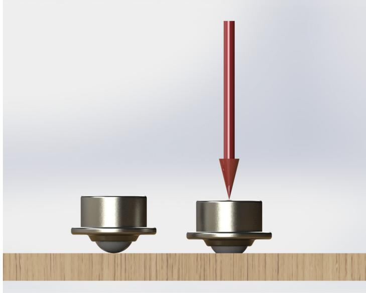
Figure 39: The left ball transfer unit represents the non-deformed situation. The right ball transfer unit the deformed state when a force (depicted by a red arrow) is applied. The deformation of the ball is exaggerated with respect to the real deformation to make the deformation visible. It can be seen that when a force is applied the contact point becomes a contact area.
