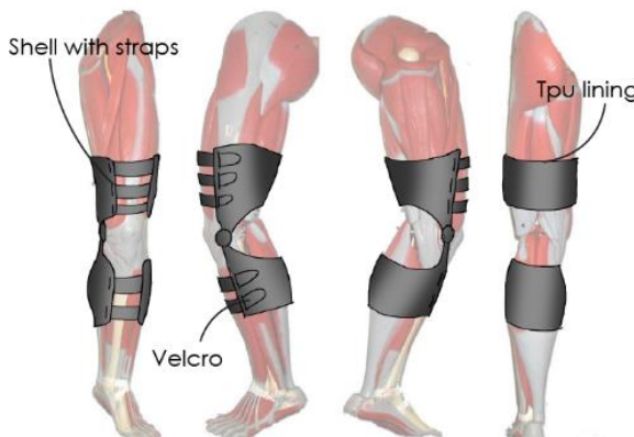
Fig. 3.2: concept 2, body fitting part
