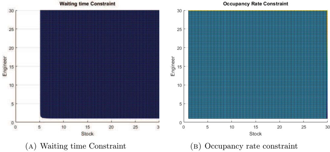
FIGURE 4.4: Feasible region of the case with  $\lambda = 0.5$ ,  $\nu = 0.4$ ,  $\nu^{em} = 10$ ,  $\mu = 3$ ,  $W^{max} = 0.002$ . The feasible region is indicated by the dark blue color on figure 4.4a.
