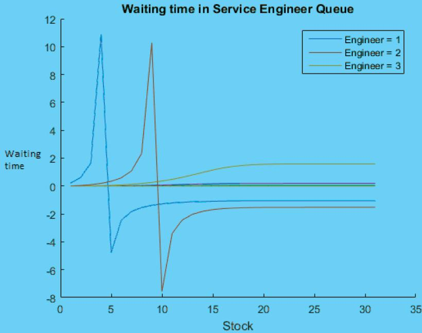
FIGURE 4.6: Average waiting time for service engineer queue with  $\lambda = 4$ ,  $\nu = 0.4$ ,  $\nu^{em} = 4$ ,  $\mu = 1.5$ ,  $W^{max} = 0.4$
