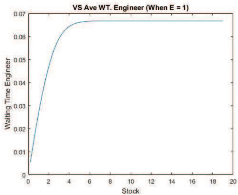
FIGURE 4.3: Average waiting time for service engineers queue with service engineer = 1
