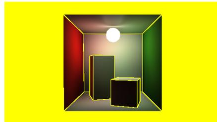
(c) Visualisation of identified edges in the Cornell box scene. Yellow areas are those for which the down-sampling scheme is deemed to be inappropriate and for which the radiance estimate is thus recomputed.
