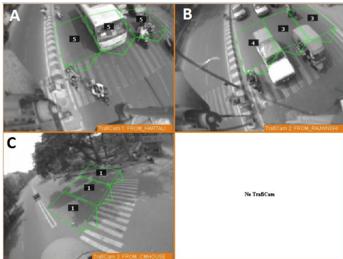
Figure 2.11 Traffic detector camera with virtual loops
