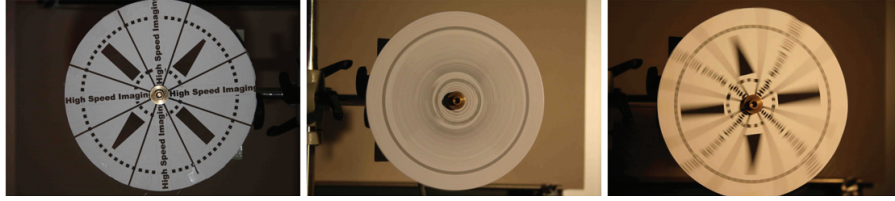
Figure 6: Talbot's high speed photography experiment. A paper disc is captured at standstill (left), spinning and captured with an exposure time of 10 ms (middle), and with an exposure time of 1 ms (right). Images courtesy of [VM11].
