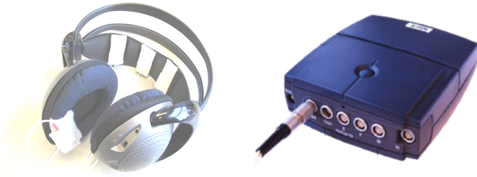
Figure 4. The left picture represents the audio headset and the EEG water electrodes; the right picture is showing the Nexus-10 acquisition device.
