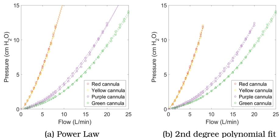
Figure 5.1: Laboratory results comparing the pressure measured in the pressure port with the atmospheric pressure for all four types of nasal cannulae. Each color indicates another nasal cannula size and the dots indicate the measured pressure at a specific flow rate. The dotted line indicates a fit through these measured point in which the left figure shows a power law fit and the right figure shows a 2nd order polynomial fit.
