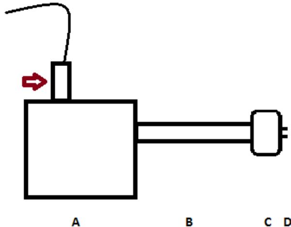
Figure 3.2: Schematic representation of the HFNC device. A is the humidifier in which the air is coming from above where the flow rate was set. *The red arrow points to the pressure port already present in the device*, B is a large heated tube, C is the connected nasal cannula and D are the nasal prongs.
