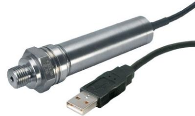
**Strain-gage** There are various types of pressure transducers, one of the most common, and the type this study uses, is the strain-gage base transducer. Pressure applied to the pressure transducer will produce a deflection of a diaphragm. This diaphragm is bonded to strain gages, in which the strain of the deflection of the diaphragm will cause a physical deformation of the strain gages. This strain will produce an electrical resistance change proportional to the applied pressure.
