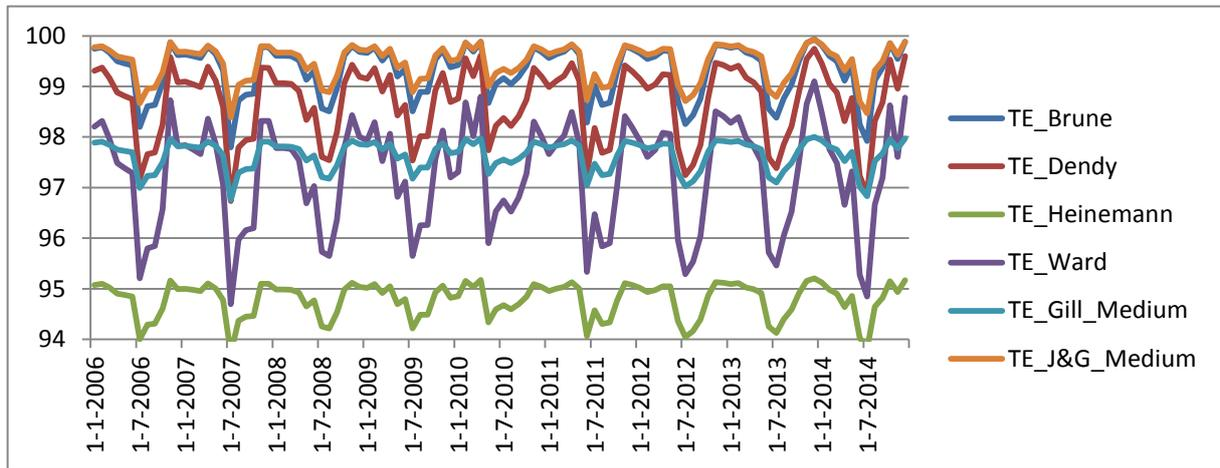
Figure 19: Trap efficiencies resulting from different empirical equations
