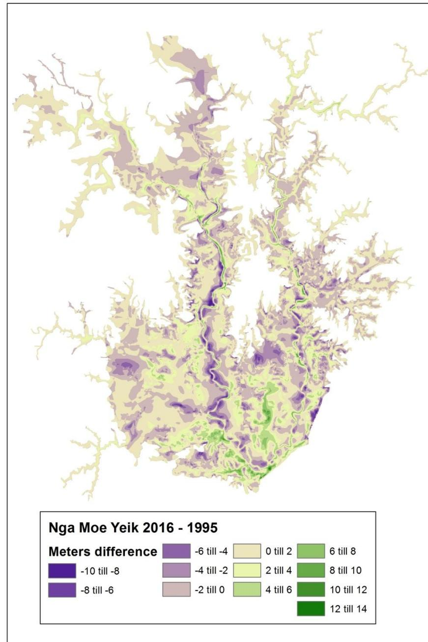
Figure 23: comparison of bed elevation levels, 2016 minus 1995
