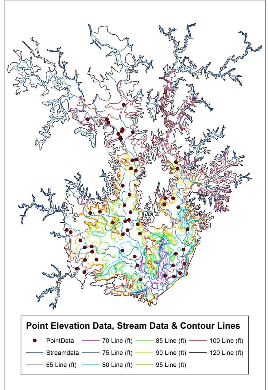
Figure 10: Digitized Point Elevation Data, Stream Data & Contour Lines
