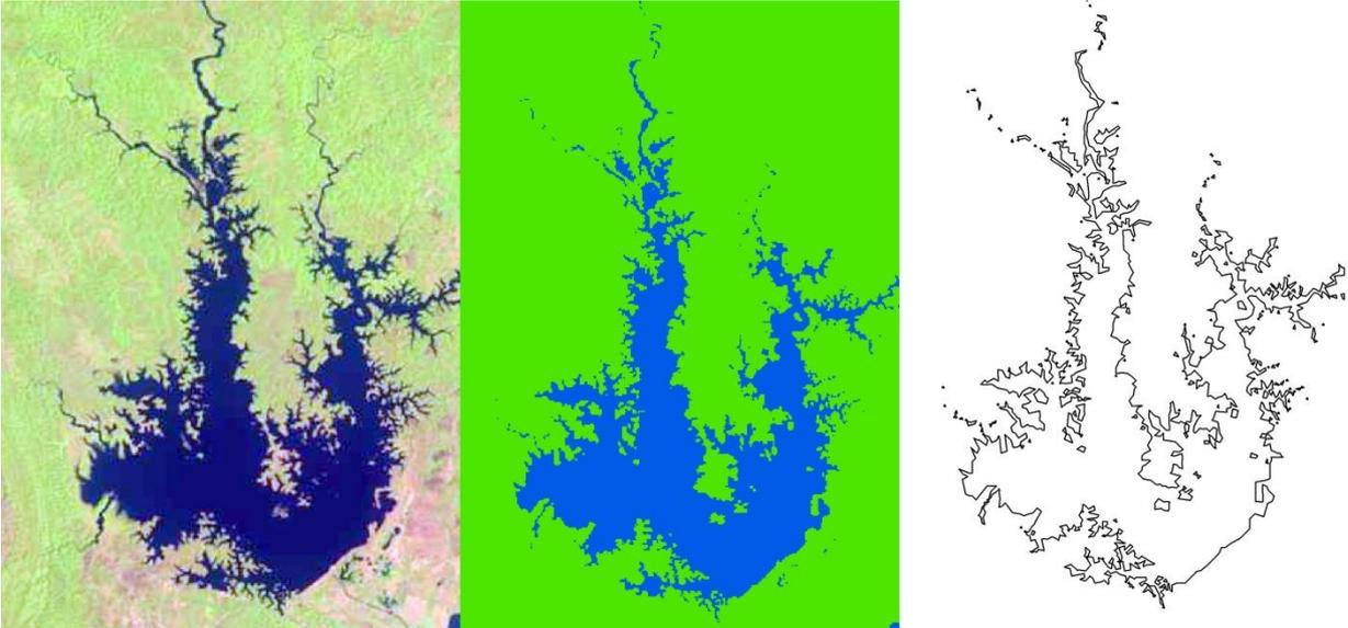
Figure 14: Left, Landsat 7 image from 29-02-2016, middle, output raster from ‘Maximum Likelihood Classification’ – tool, right, Polylines of water surface
