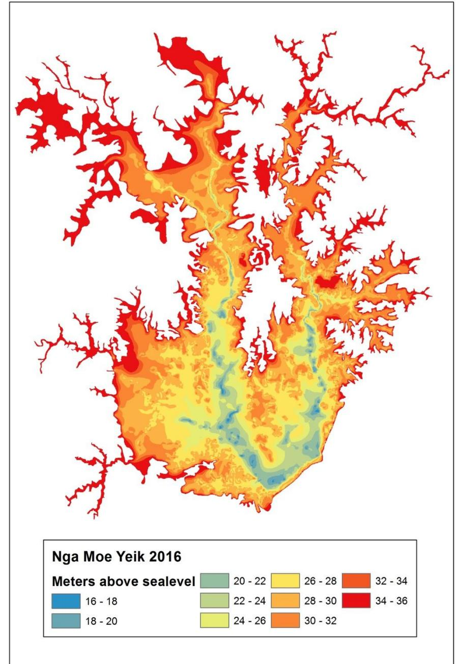
Figure 21: the elevation of the reservoirs bed as it is present in 2016
