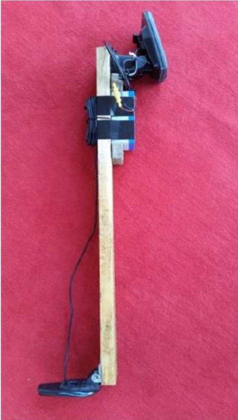
*Figure 31: the echo sounder setup*
