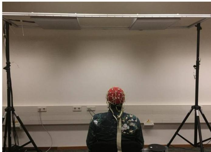
**Figure 3.3.** A participant wearing an EEG cap and the experimental setup. The picture depicts the two LED panels are above and the white wall in front of the participant.
