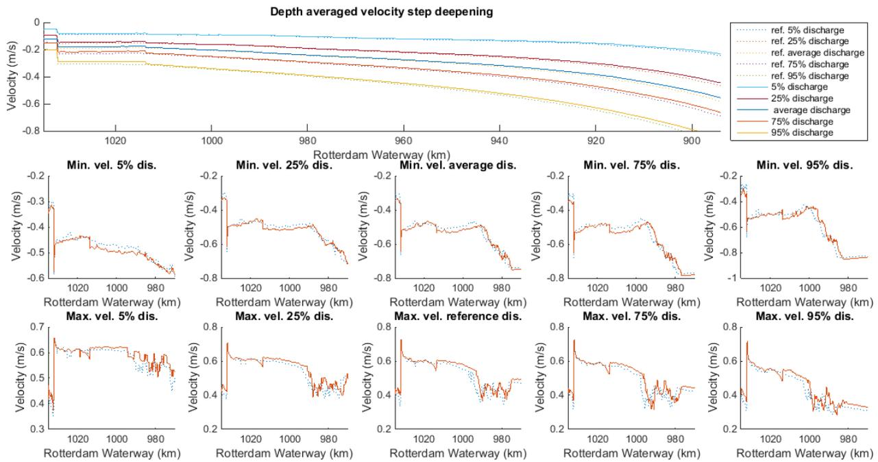
Figure 68 Depth average velocity for discharge sensitivity (upper panel); Flood (maximum) and ebb (minimum) velocity due compared (orange line) with reference depth (dashed line) for discharge sensitivity
