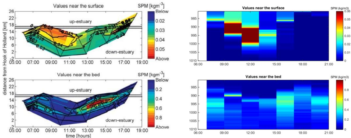
Figure 21 Left panel: SPM concentration measured by De Nijs et al. (2010). Right panel: calculated SPM with 4 weeks run up time
