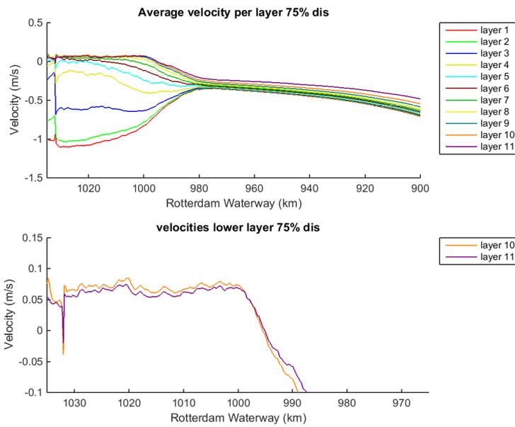
Figure 119 Average velocity per layer for 75% discharge (upper panel) and lowest two layers (lower panel)
