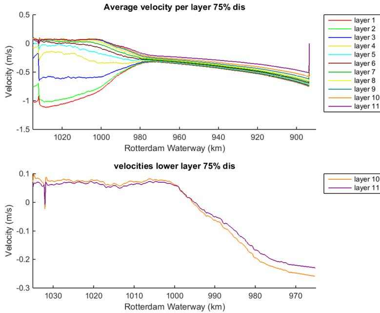
Figure 159 Average velocity for all layers (upper panel) and for the lowest two layers for the 75% discharge
