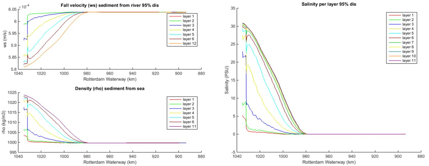
Figure 160 Fall velocity and density (left) and salinity (right) for the ETM deepening scenario 95% discharge
