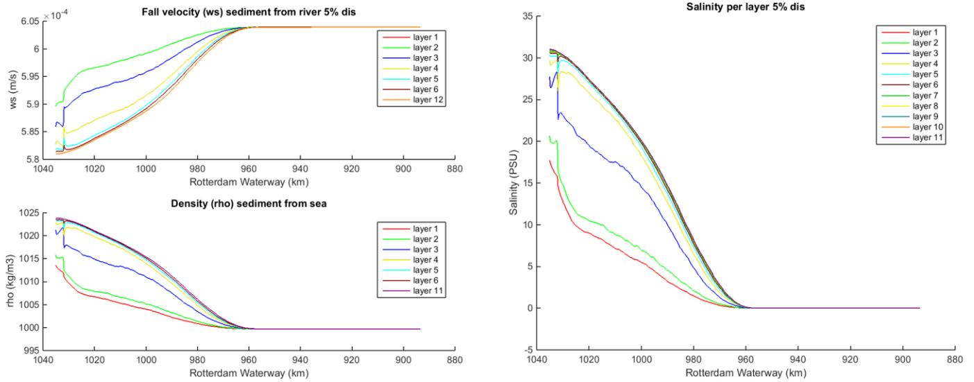
Figure 111 Fall velocity and density (left panels) and salinity for 5% discharge (right)
