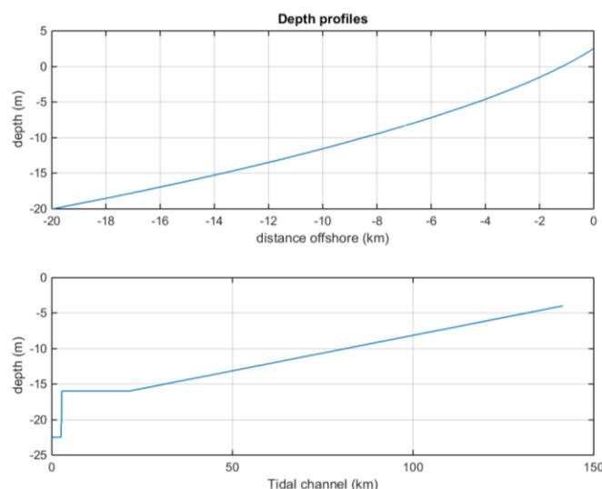
Figure 16 Bathymetry of a) the foreshore of the North Sea; b) the depth of the Rotterdam Waterway including the navigational channel
