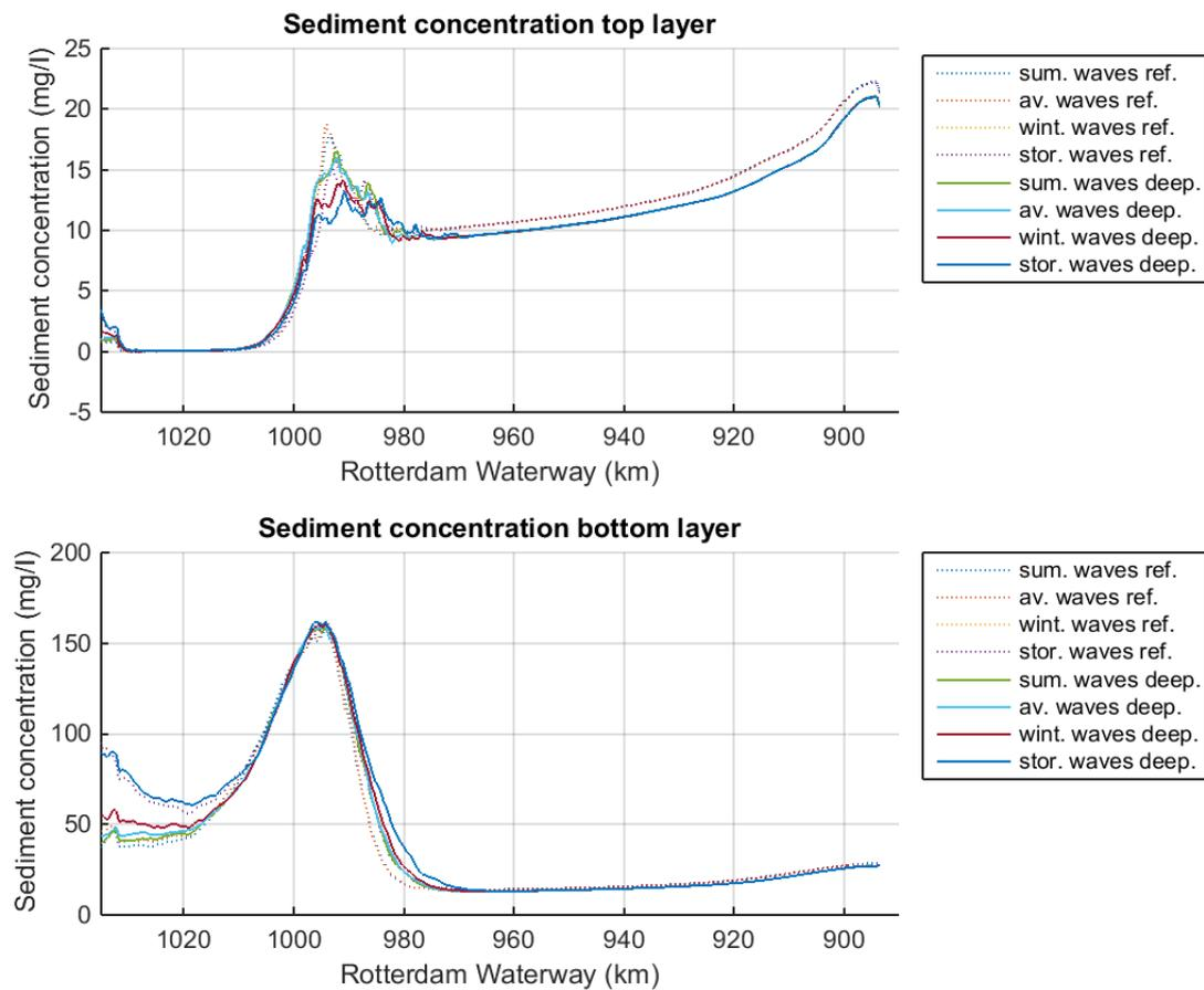
Figure 72 Concentration suspended sediment for the top layer (upper panel) and the bottom layer (lower panel) due to changing discharge for the reference scenario (dashed line) and the step deepening scenario
