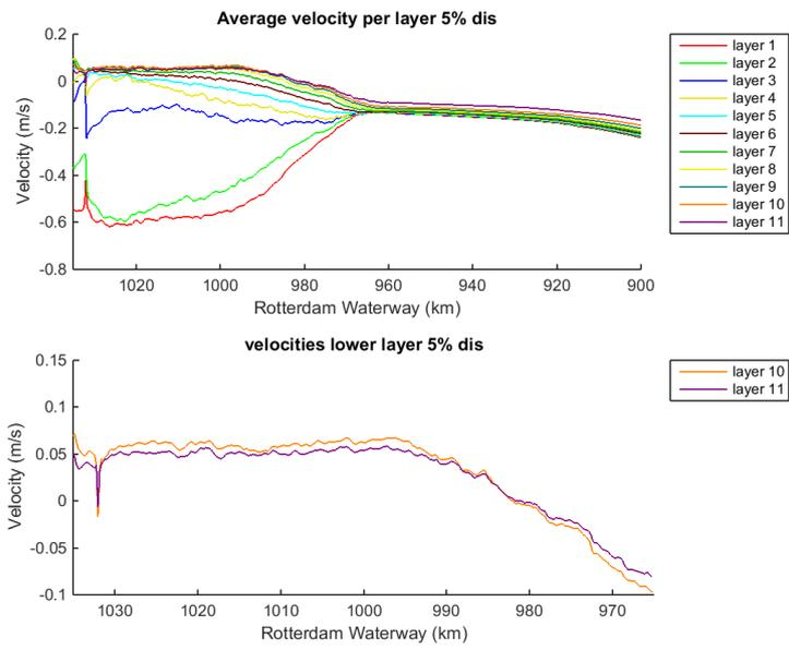
Figure 113 Average velocity per layer for 5% discharge (upper panel) and lowest two layers (lower panel)
