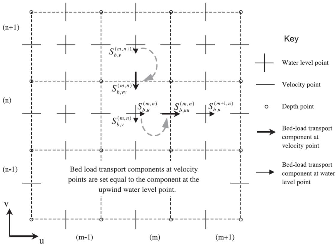
Figure 89 Solution procedure Delft3d (Lesser et al., 2004)
