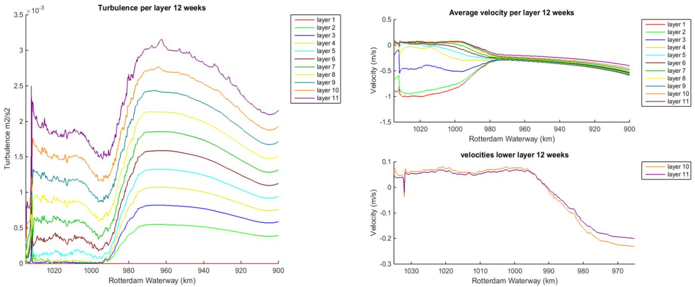
Figure 108 Turbulence in the Rotterdam Waterway on the left; Velocity per layer in the upper right figure; velocity profile of the nearbed layers in the lower right panel. Positive velocity indicates flood, a negative velocity indicates ebb
