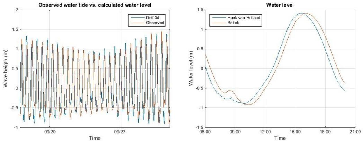
Figure 17 Left panel: Observed (orange) vs. calculated water level (blue). Right panel: water level of Hook of Holland (blue) and Botlek (orange)
