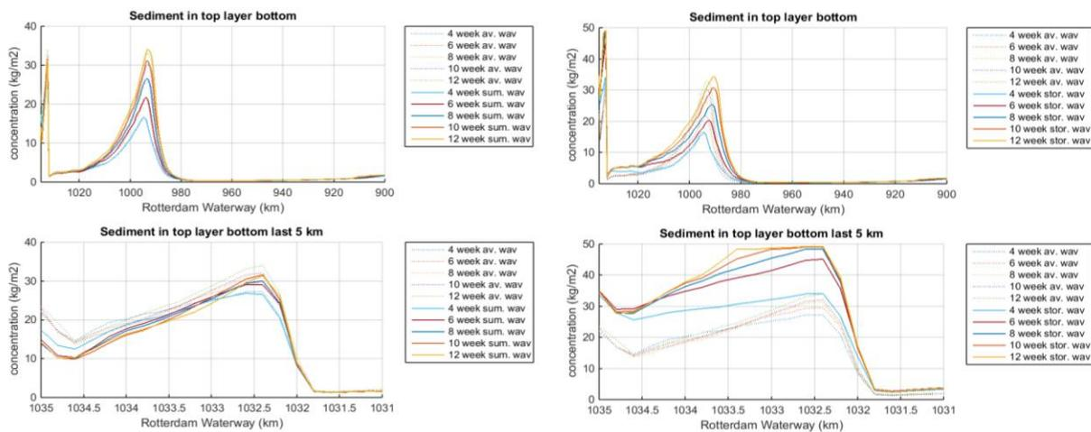
Figure 44 Available sediment in top layer for summer waves (left) and storm waves (right)
