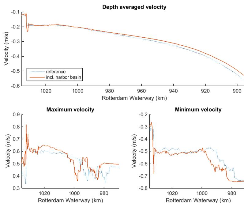
Figure 46 Depth average velocity (upper panel) of the reference scenario and the scenario including the harbor basins. Average flood velocity (lower left panel); Average ebb velocity (lower right panel)
