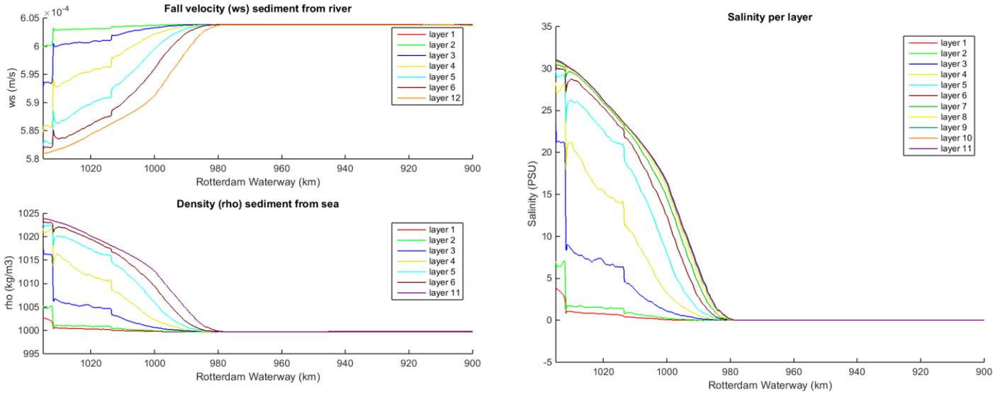
Figure 146 Fall velocity, density and salinity per layer for the deepened scenario
