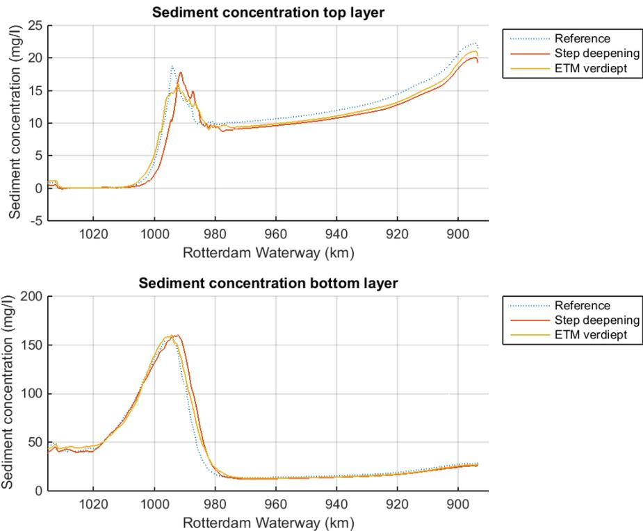
Figure 60 Suspended sediment concentration for the top and bottom layer for the different scenarios
