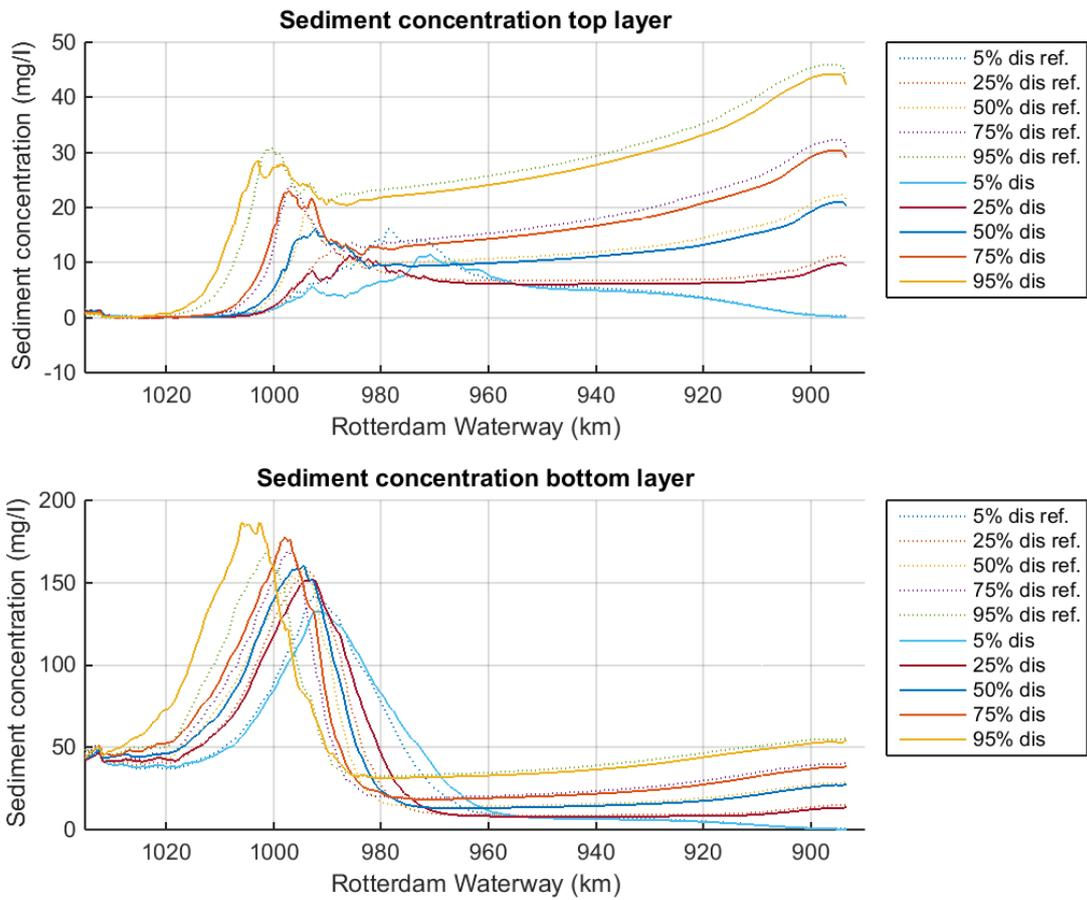
Figure 71 Concentration suspended sediment for the top layer (upper panel) and the bottom layer (lower panel) due to changing discharge for the reference scenario (dashed line) and the step deepening scenario
