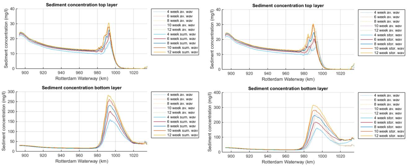
Figure 129 Fine sediment concentration for summer waves (left panel) and storm waves (right panel)
