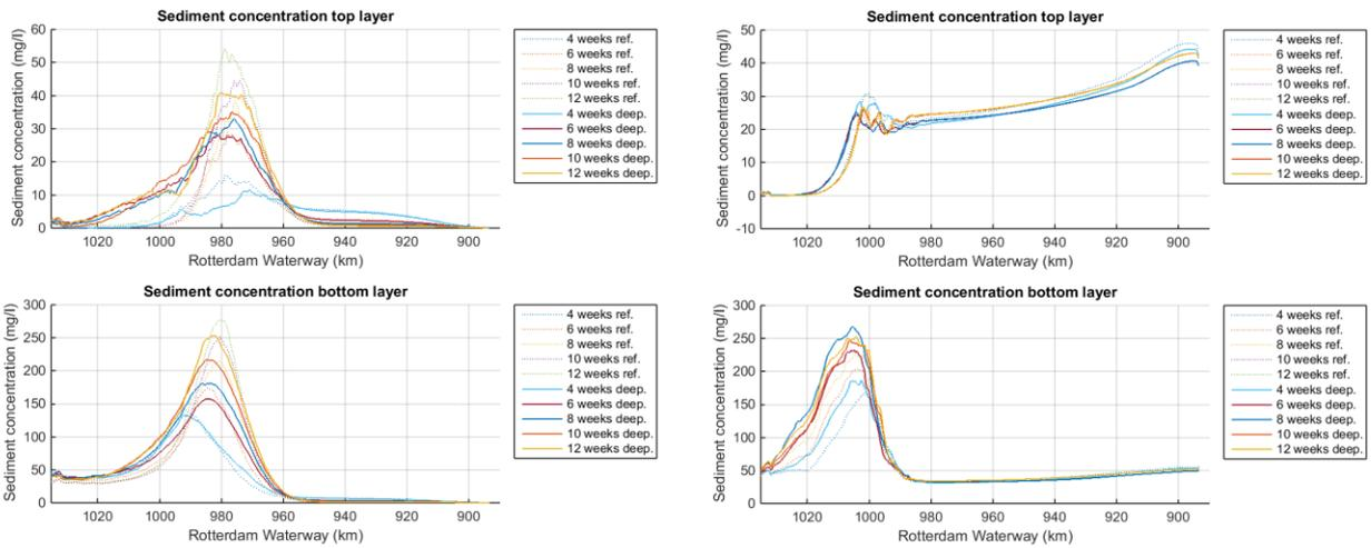
Figure 84 Medium term growth of the ETM for the 5% discharge (left) and for the 95% discharge right
