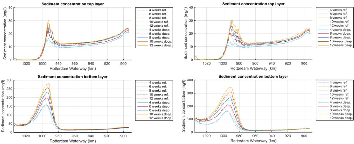
Figure 86 Medium term growth of the ETM for the summer waves (left) and for the storm waves right
