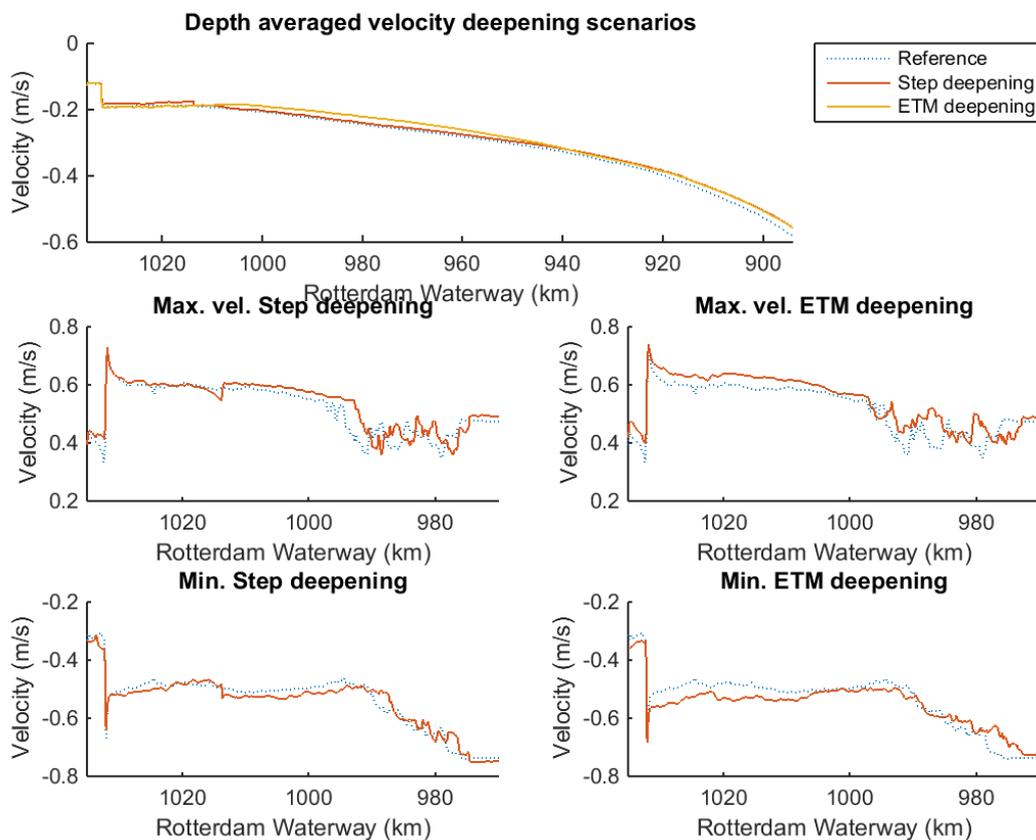
Figure 55 Left: change in minimum and maximum velocity due to deepening
