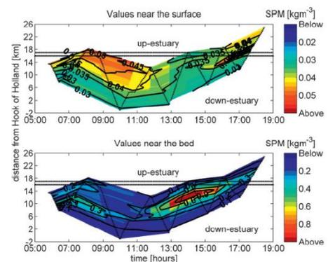
Figure 8 SPM concentration near the surface (upper panel) and near the bottom (lower panel) (De Nijs et al., 2011)
