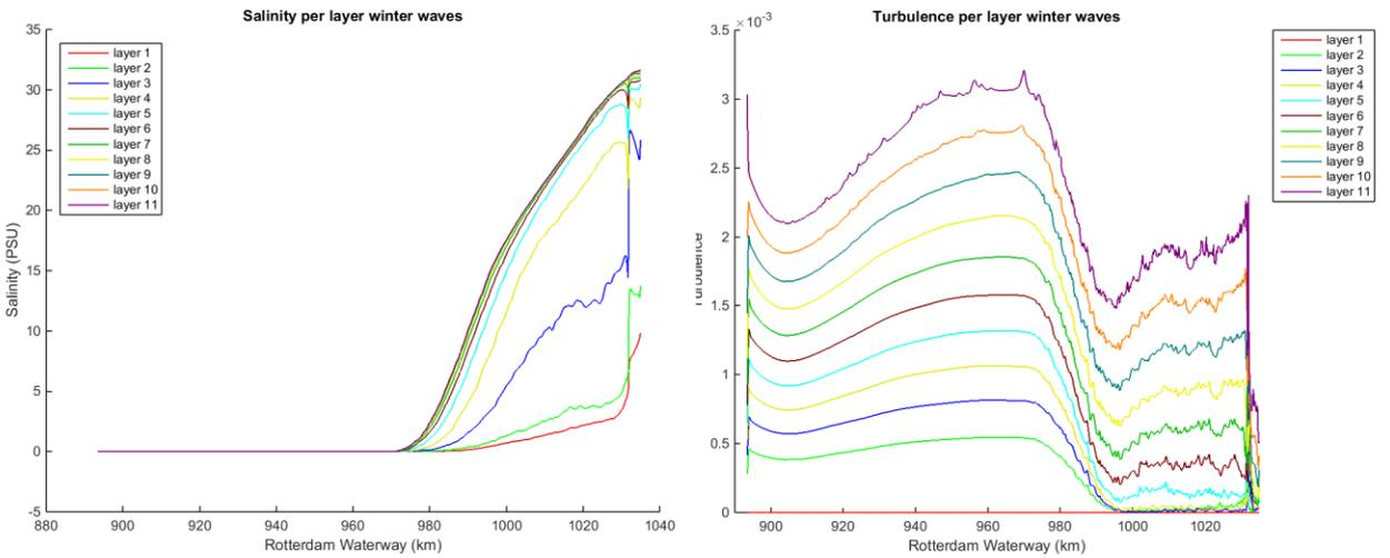
Figure 124 Salinity (left) and turbulence (right) for winter waves
