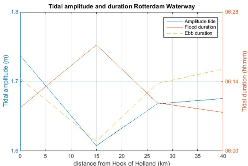
Figure 12 Tidal amplitude and duration in 2015 for Hook of Holland (km 0), Maassluis (km 15), Vlaardingen after bifurcation (km 27) and Rotterdam (km 40) (Rijkswaterstaat, 2016)
