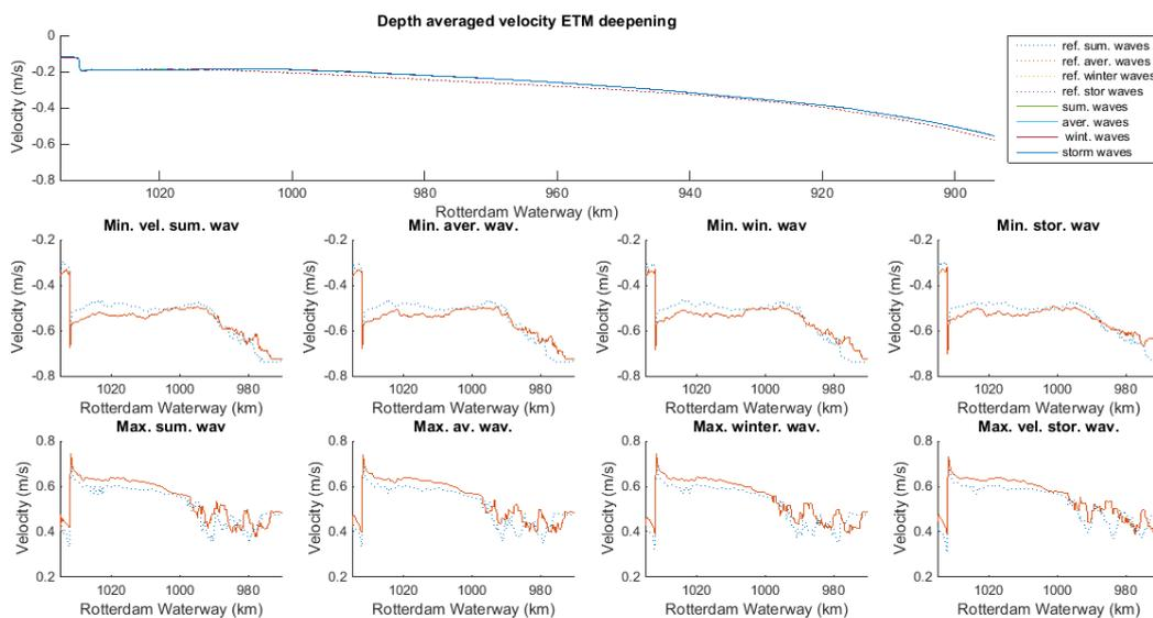
Figure 81 Depth average velocity for changing wave conditions (upper panel); Ebb and flood velocity for different wave conditions (lower panel)
