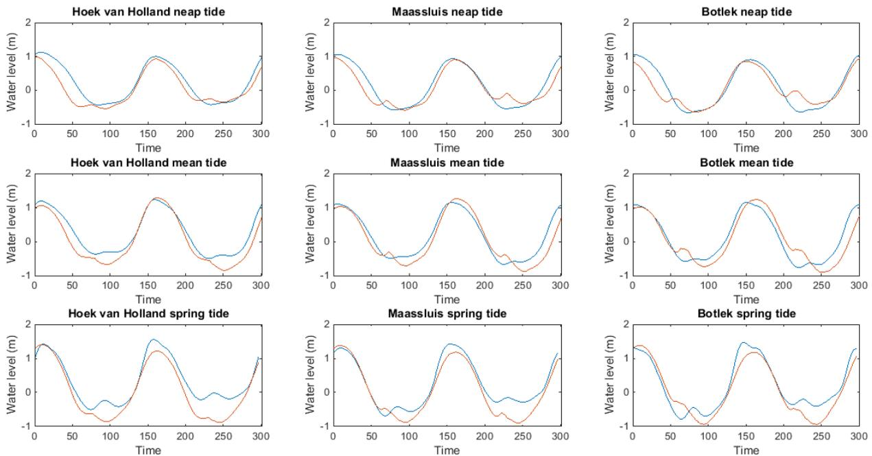
Figure 18 Water levels for Hook of Holland, Maassluis and the Botlek for three tides of the HBR model (in blue) and the calculated values (in orange).
