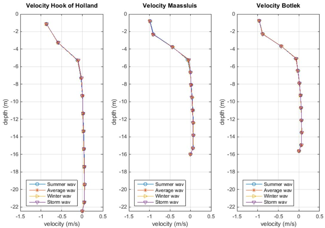
Figure 80 Average velocity for the ETM deepening for Hook of Holland, Maassluis and the Botlek due to changing wave conditions
