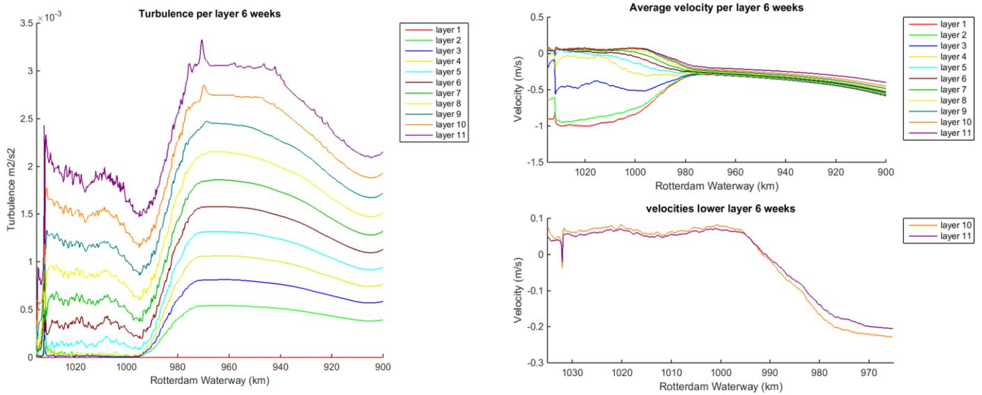
Figure 102 Turbulence in the Rotterdam Waterway on the left; Velocity per layer in the upper right figure; velocity profile of the near bed layers in the lower right panel. Positive velocity indicates flood, a negative velocity indicates ebb
