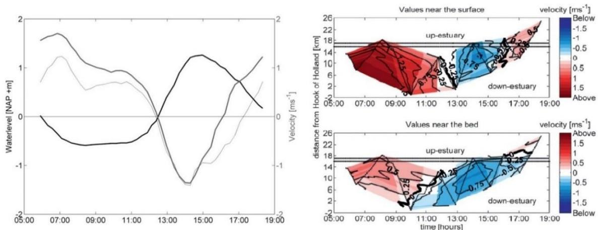
Figure 4 Left: Water level (black) velocity; velocity 2.5 m below surface (dark grey); velocity 12.5 m below surface (light grey) 15 km upstream of Hook of Holland. Right: velocities near the surface (upper panel); velocity near the bottom. Negative velocity indicates flood velocity (lower panel) (De Nijs *et al.*, 2011).
