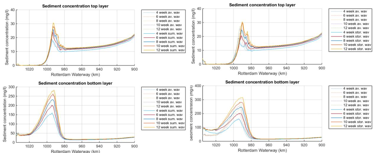
Figure 43 Sediment concentration along the Rotterdam Waterway in the left panel during summer waves; in the right panel for the long term storm waves
