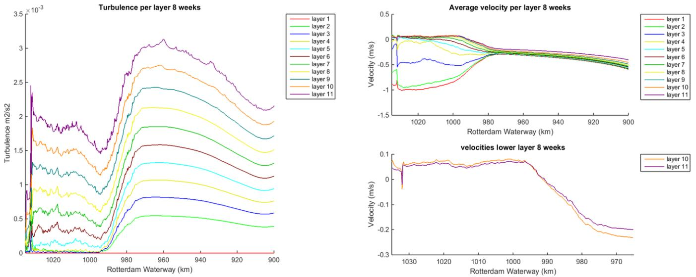
Figure 104 Turbulence in the Rotterdam Waterway on the left; Velocity per layer in the upper right figure; velocity profile of the near bed layers in the lower right panel. Positive velocity indicates flood, a negative velocity indicates ebb
