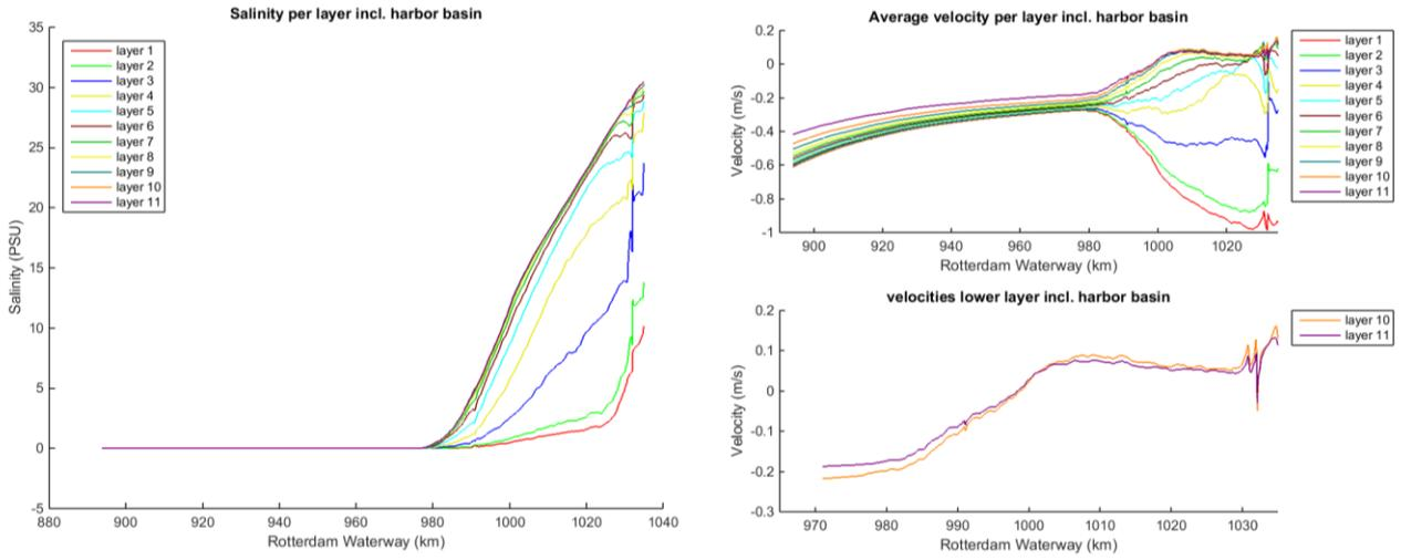
Figure 130 Salinity of the Rotterdam Waterway (left); averaged velocity (right)
