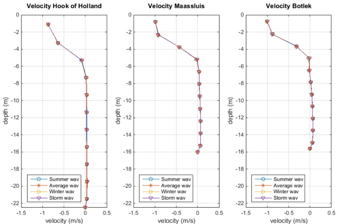
Figure 69 Average velocity for Hook of Holland, Maassluis and the Botlek for the changing wave conditions
