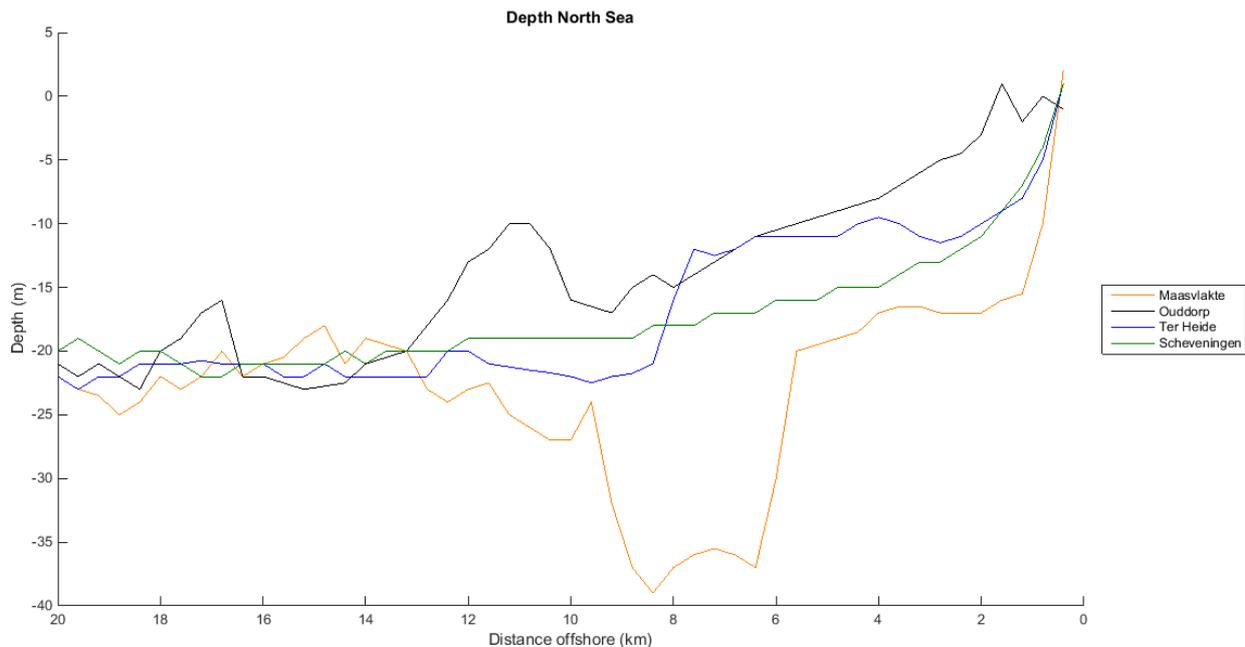
Figure 10 Bathymetry North Sea for four locations
