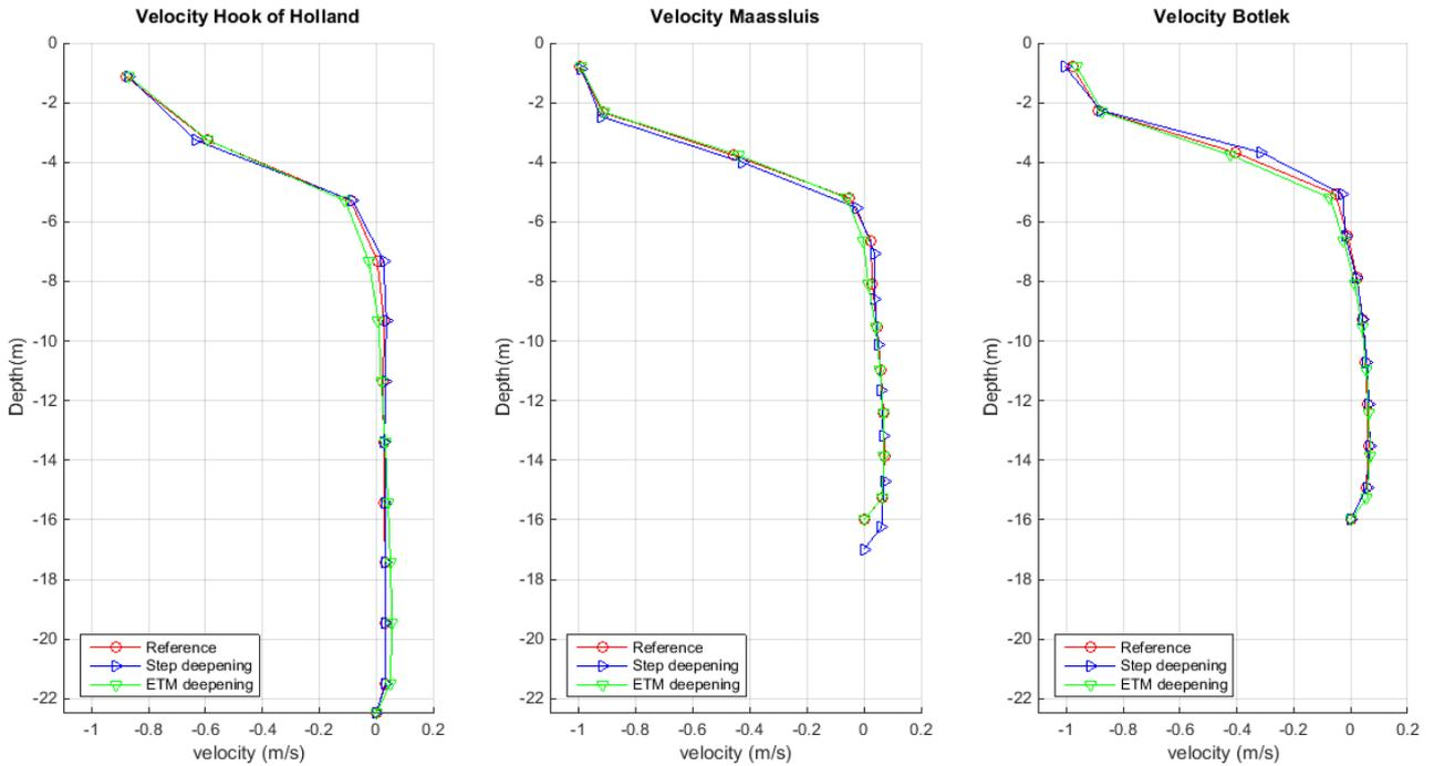
Figure 51 Average velocity for Hook of Holland (km 1034.6), Maassluis (km 1021.8) and the Botlek (km 1009.4) for the reference and deepening scenarios. Negative velocity means ebb velocity, and the positive velocity means flood velocity.
