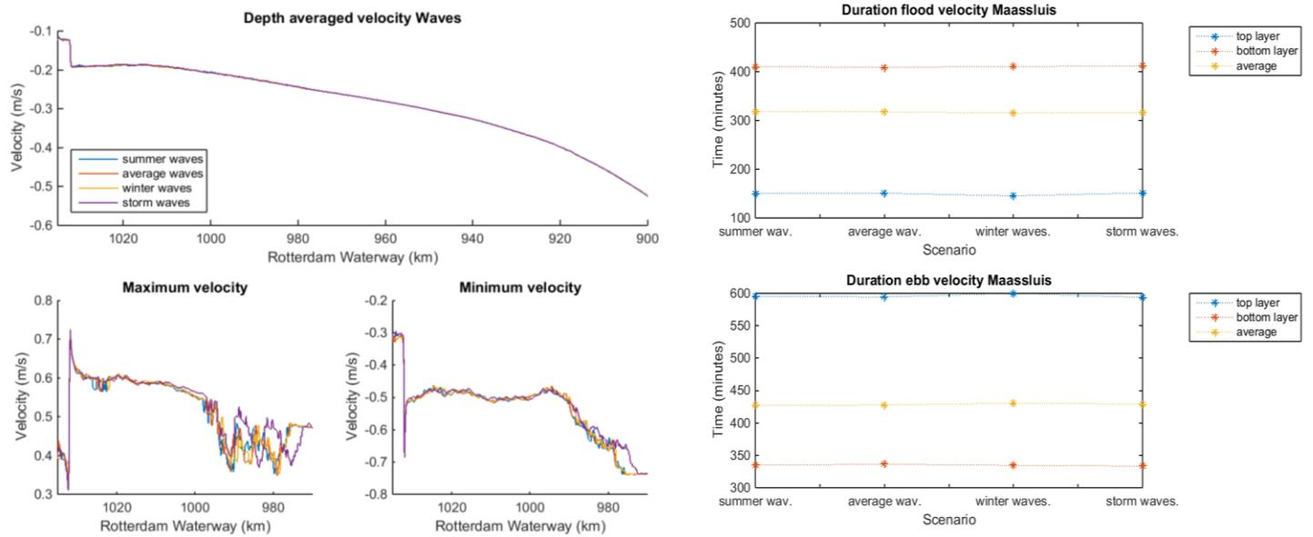
Figure 40 Top: Depth averaged velocity for the different scenarios; Lower left panel: Maximum (flood) velocity; Lower right panel minimum (ebb) velocity
