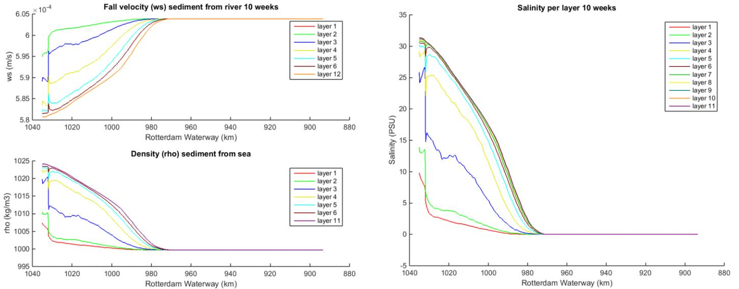
Figure 105 Fall velocity, density and salinity per layer for average discharge
