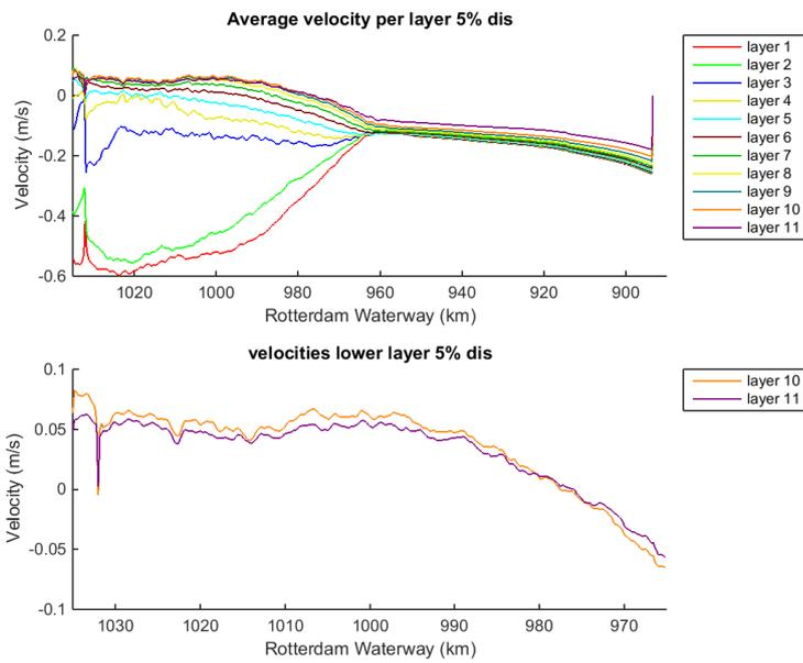
F.2.1.2. *Figure 153 Average velocity for all layers (upper panel) and for the lowest two layers for the 5% discharge* 25% discharge
