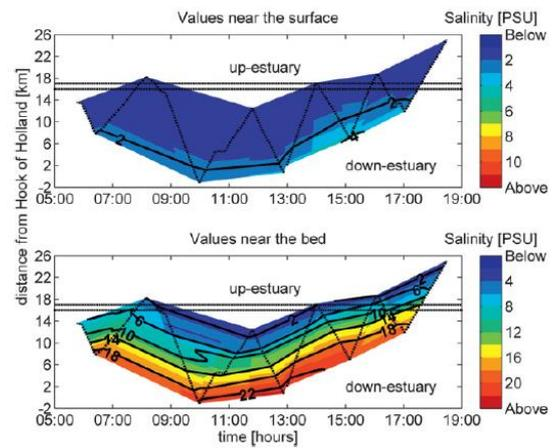
Figure 3 Along channel salinity distribution in at the surface in the upper panel and the salinity at the bottom at the lower panel (de Nijs *et al.*, 2011)
