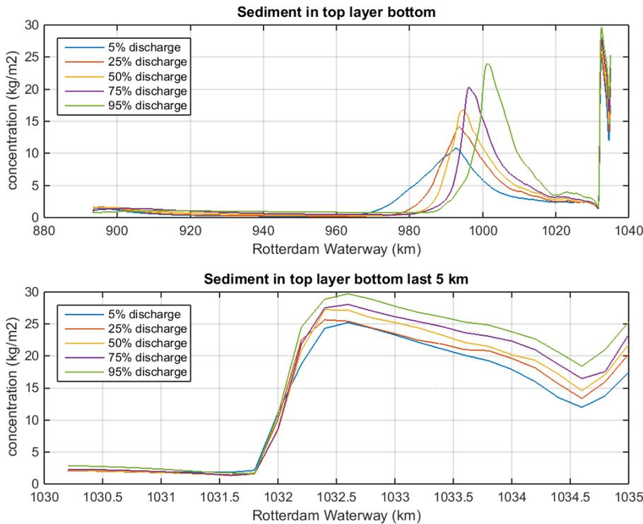
Figure 126 Available sediment in top layer of the bottom after 4 weeks
