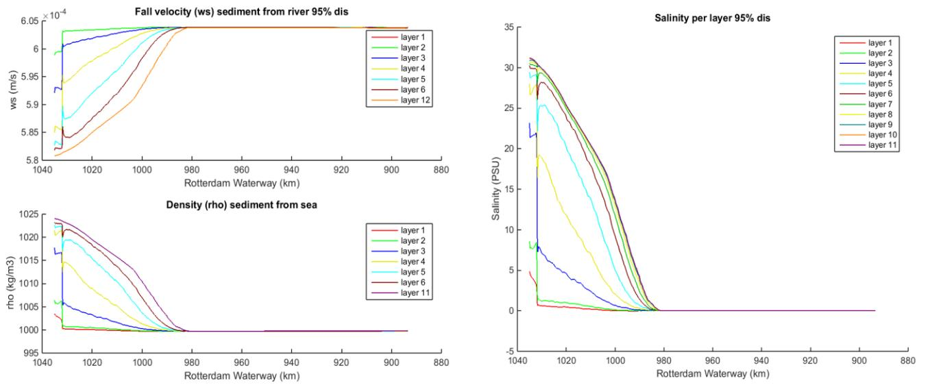
Figure 121 Fall velocity and density (left panels) and salinity for 95% discharge (right)
