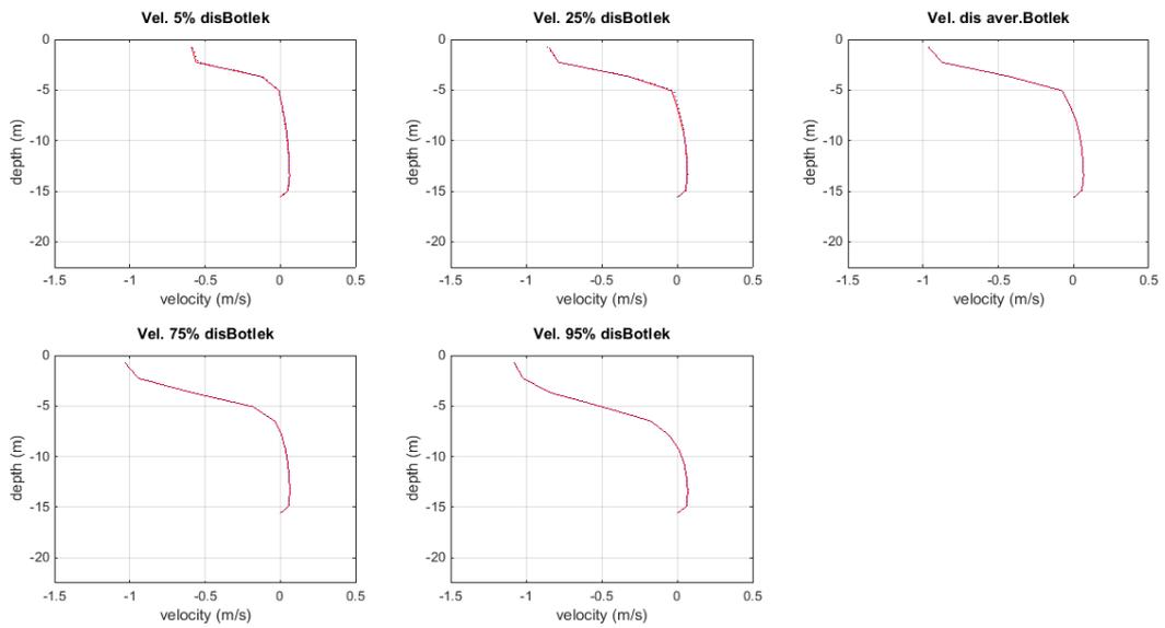
Figure 150 Changing average discharge for changing discharge near Botlek due to ETM deepening
