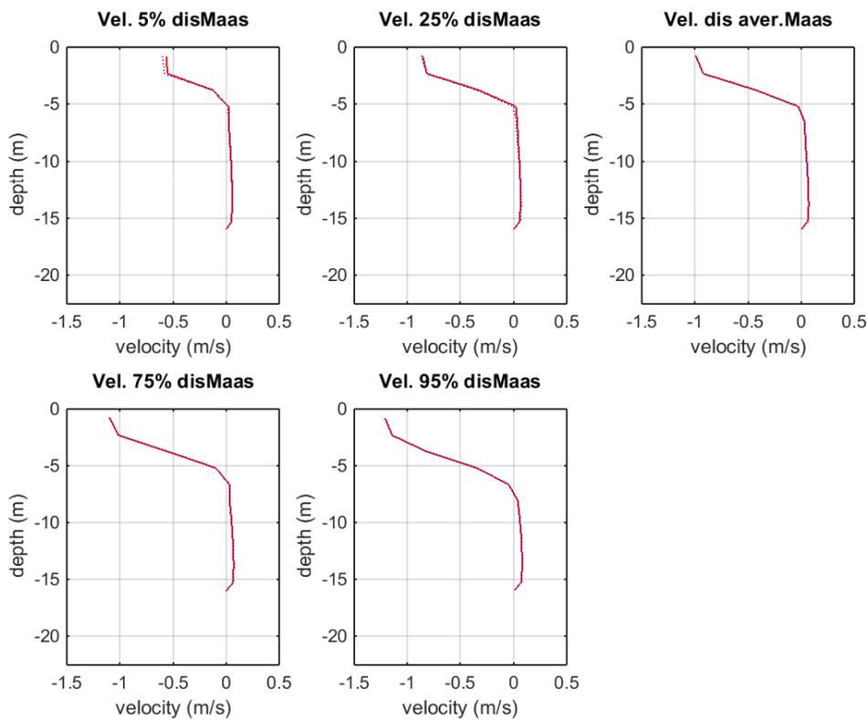
Figure 135 Change in velocity due to changing discharge for the reference scenario (dashed blue line) with the step deepening scenario (in red)
