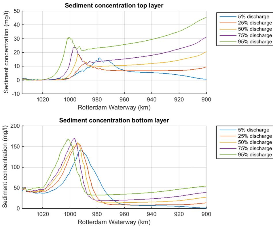
Figure 36 Tide integrated sediment concentration with varying discharge for the top layer (upper panel) and near bottom layer (lower panel)
