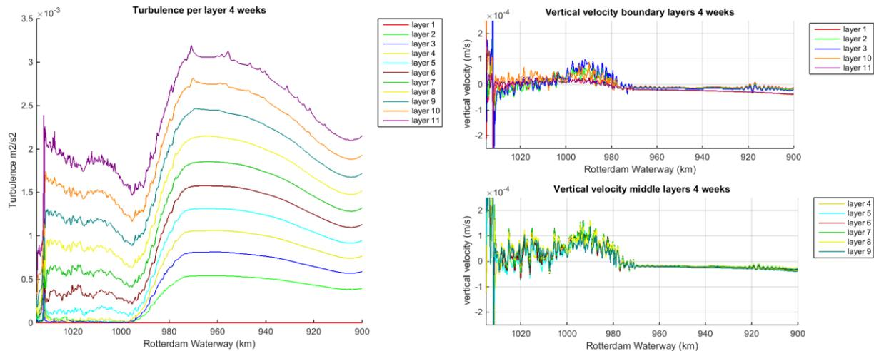
Figure 27 Left panel: turbulence per layer; Righter panel: vertical velocity of the boundary layers (upper panel) and of the middle layers (lower panel)
