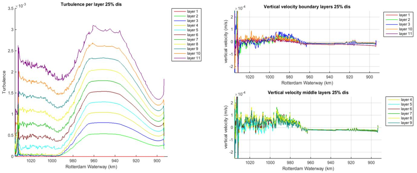
Figure 155 Turbulence (left) and vertical velocity for boundary layers and middle layers for 25% discharge
