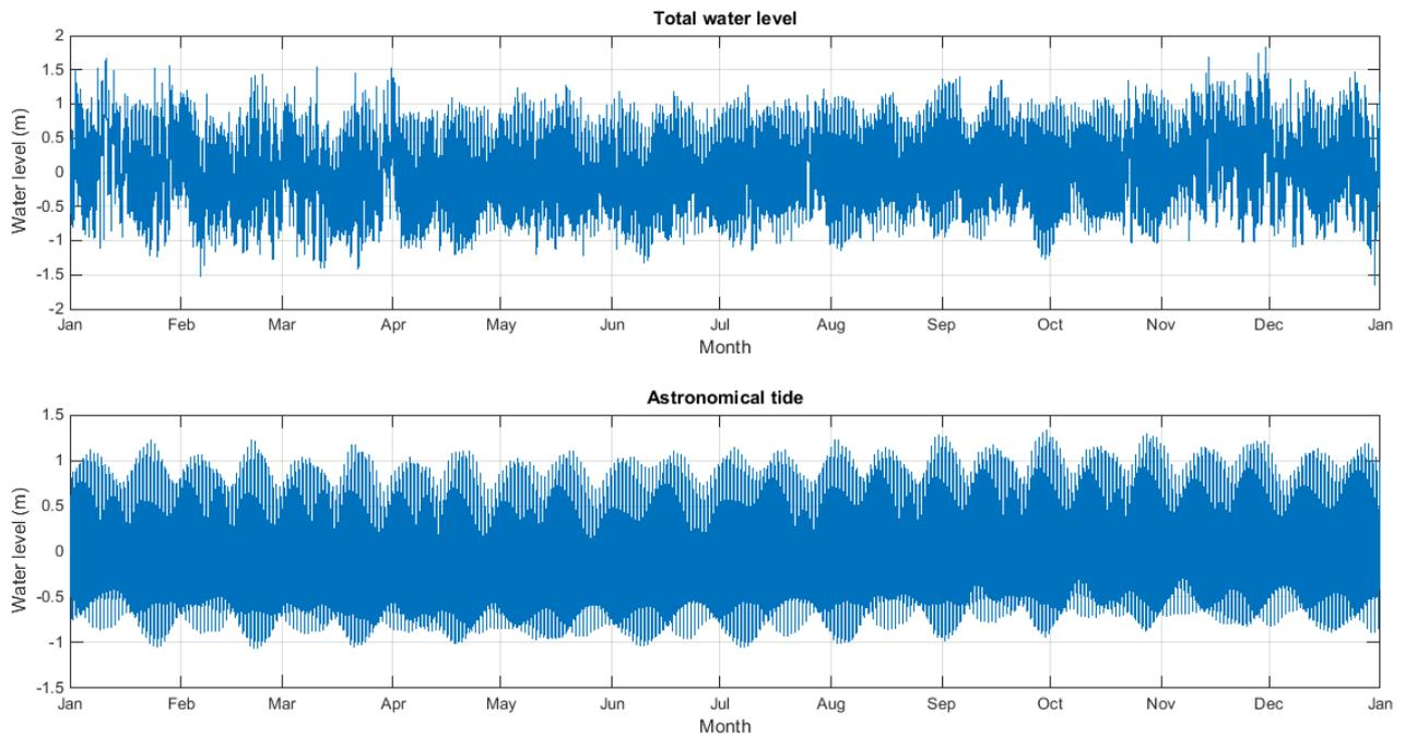
Figure 11 Tidal characteristics Europlatform in 2015 (Rijkswaterstaat, 2016)
