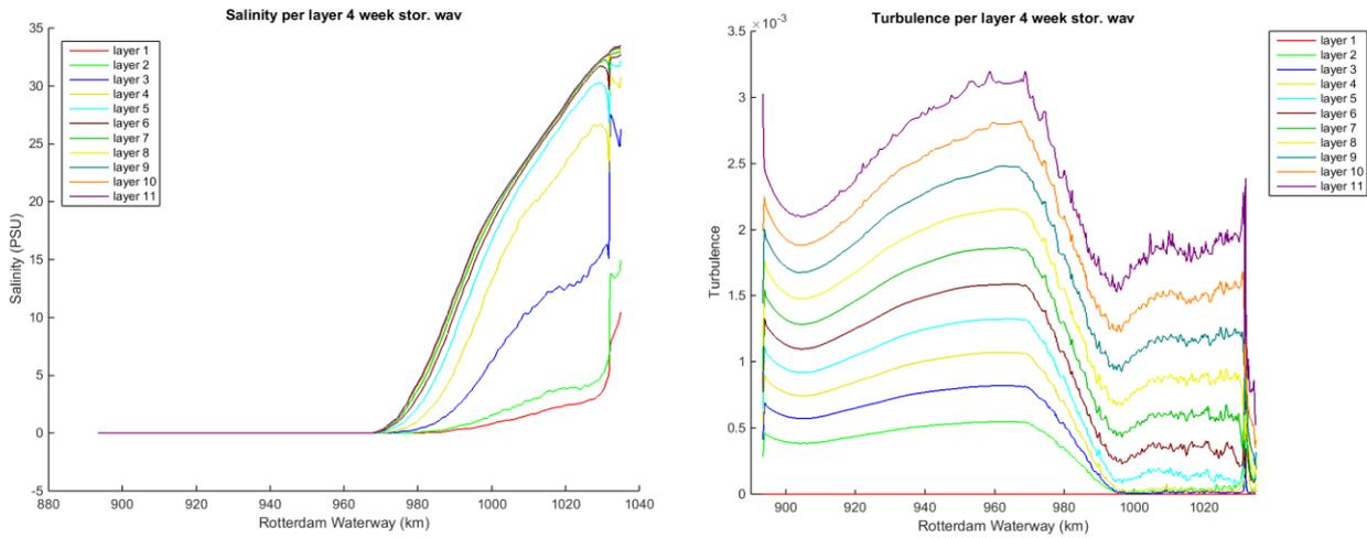
Figure 125 Salinity (left) and turbulence (right) for storm
