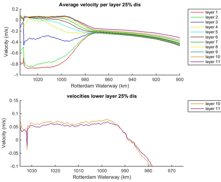
Figure 116 Average velocity per layer for 25% discharge (upper panel) and lowest two layers (lower panel)
