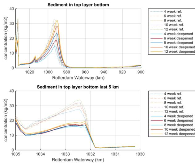
Figure 63 Available sediment in bottom layer for ETM deepening scenario
