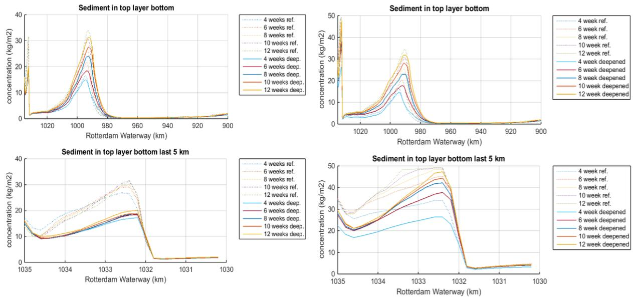
Figure 87 Available sediment in bottom layer for summer waves (left) and storm waves (right) for the ETM deepening scenario, compared with the reference scenario
