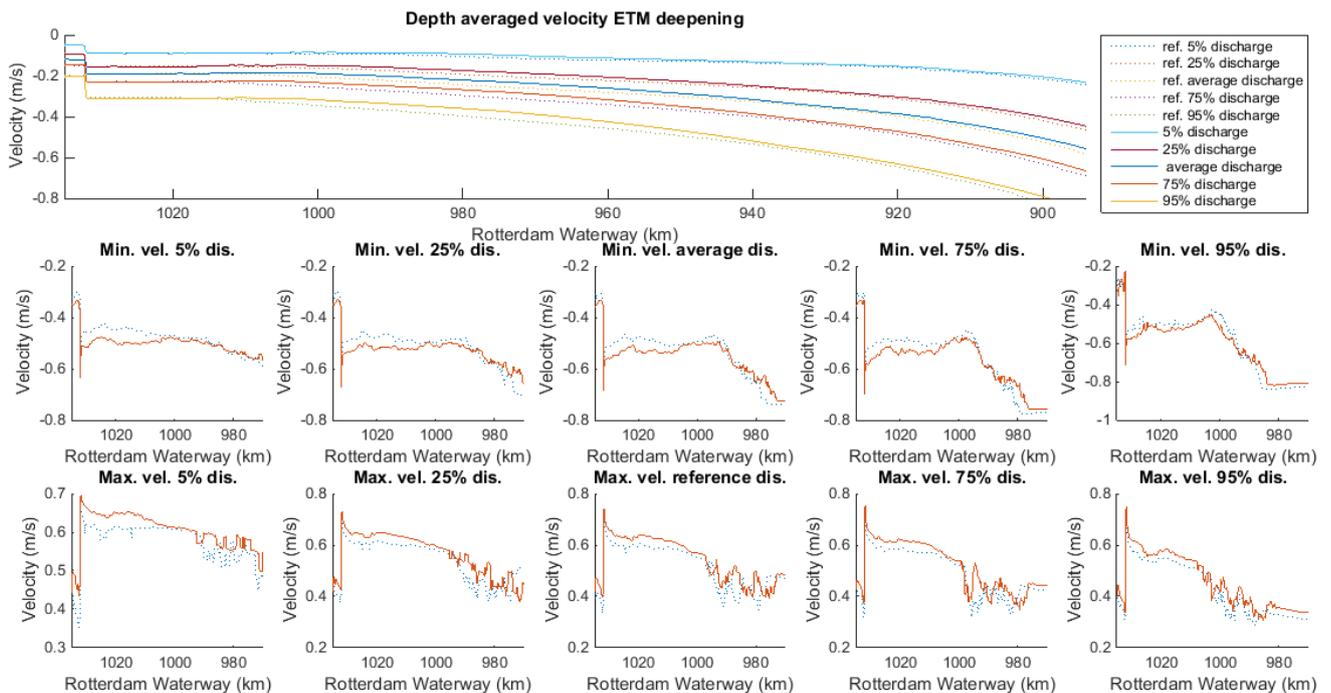
Figure 79 Depth average velocity for discharge sensitivity (upper panel); Flood (maximum) and ebb (minimum) velocity due compared (orange line) with reference depth (dashed line) for discharge sensitivity
