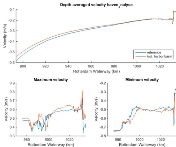
Figure 132 Depth averaged velocity (upper panel); average flood and ebb velocity (lower panel)
