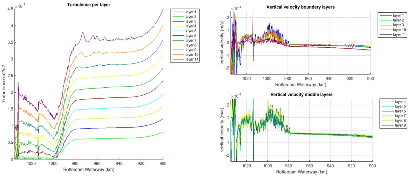
Figure 145 Turbulence, average velocity for all layers and specific for the two lowest layers
