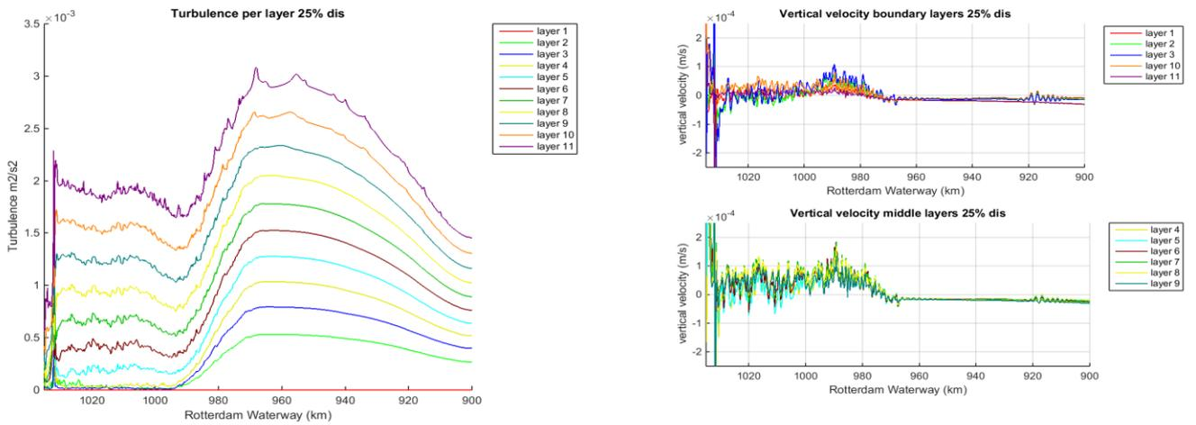
Figure 115 Turbulence (left) and vertical velocity for boundary layers and middle layers for 25% discharge
