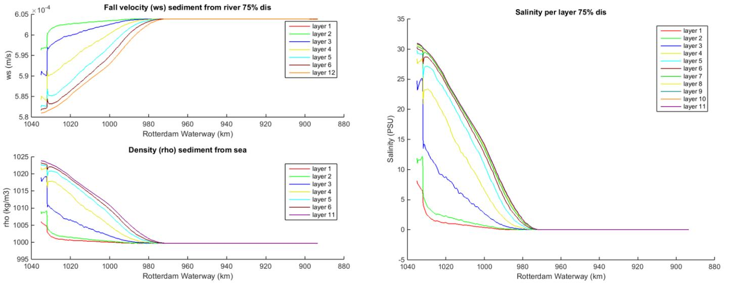
Figure 157 Fall velocity and density (left) and salinity (right) for the ETM deepening scenario 75% discharge
