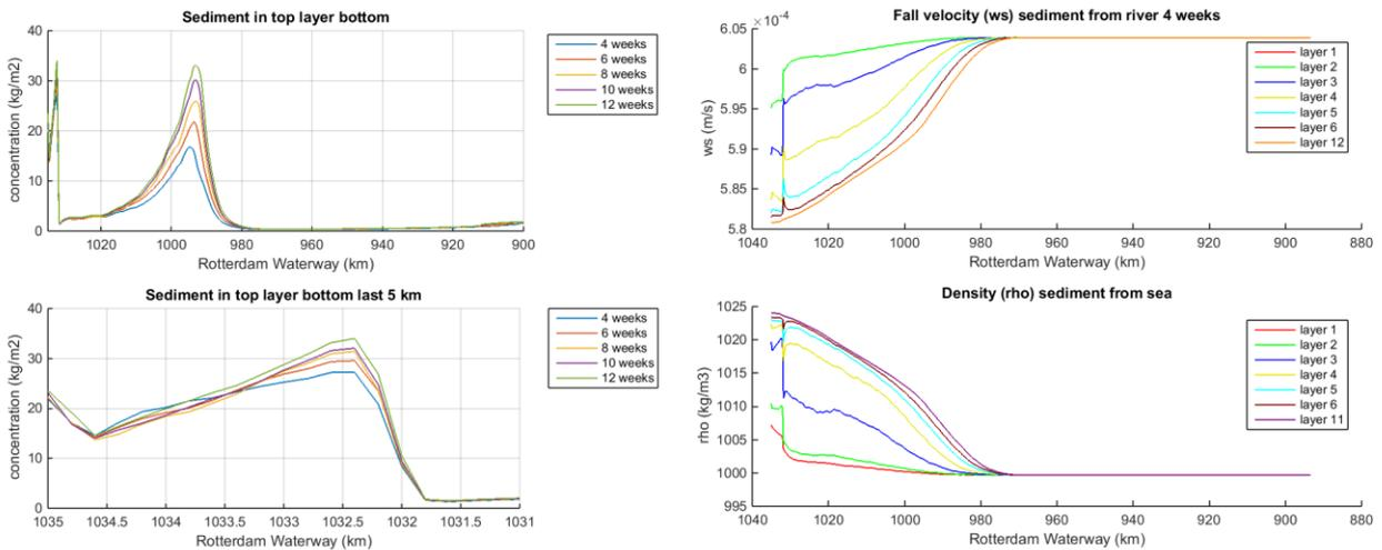
Figure 29 Left: Available fine sediment in top layer; Right upper panel: fall velocity righter lower panel density water column
