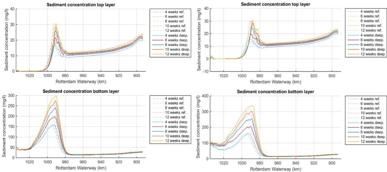
Figure 75 ETM in time for summer waves (left panel) and storm waves (right panel) for the reference depth (dotted line) and the deepened scenario
