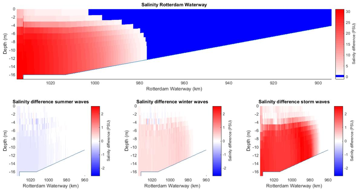
Figure 39 Salinity for the reference case (upper panel); Salinity difference between reference case and summer waves (lower left panel); Salinity difference reference case and storm waves (lower right panel)
