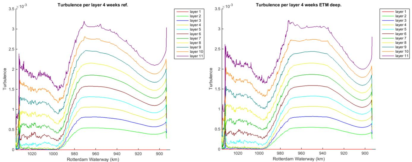
Figure 57 Turbulence for the reference scenario (left panel) and the deepened scenario (right panel)
