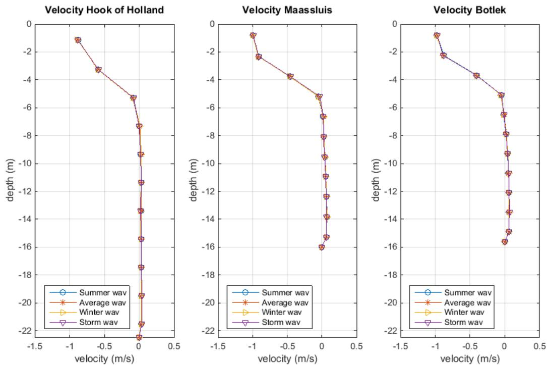
Figure 41 Velocity profiles due to changing wave conditions
