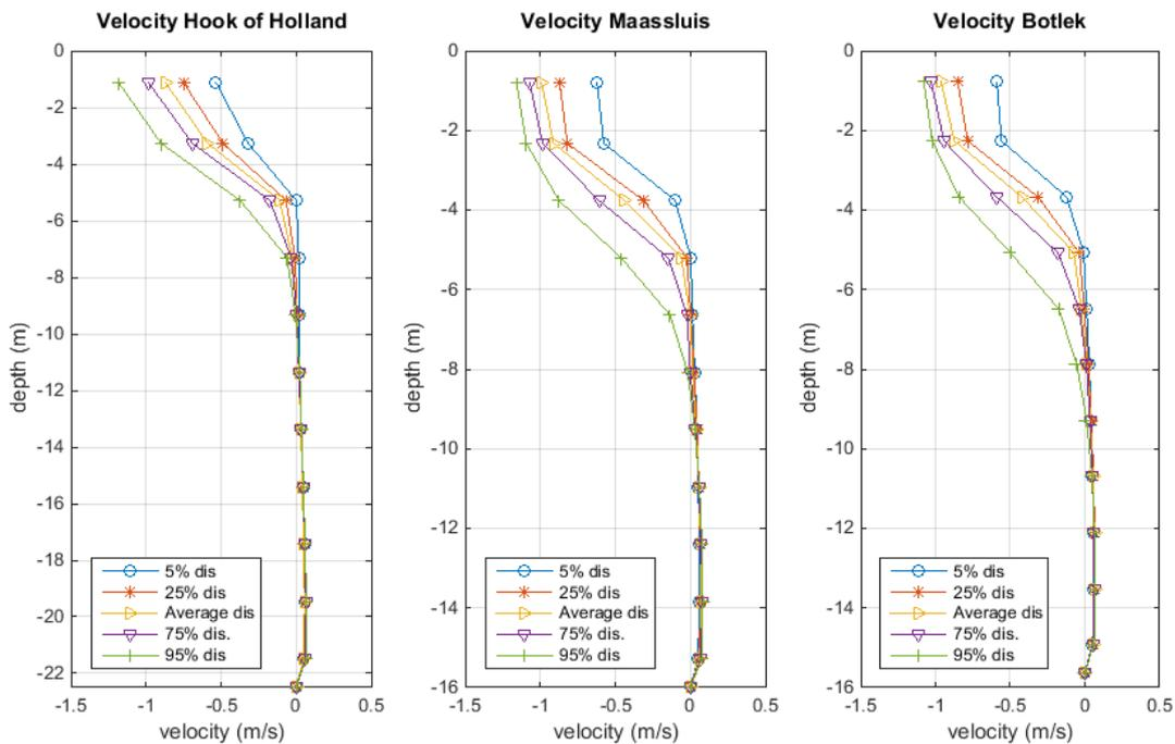
Figure 78 Average velocity for Hook of Holland (km 1034.6), Maassluis (km 1024) and the Botlek (km 1009)
