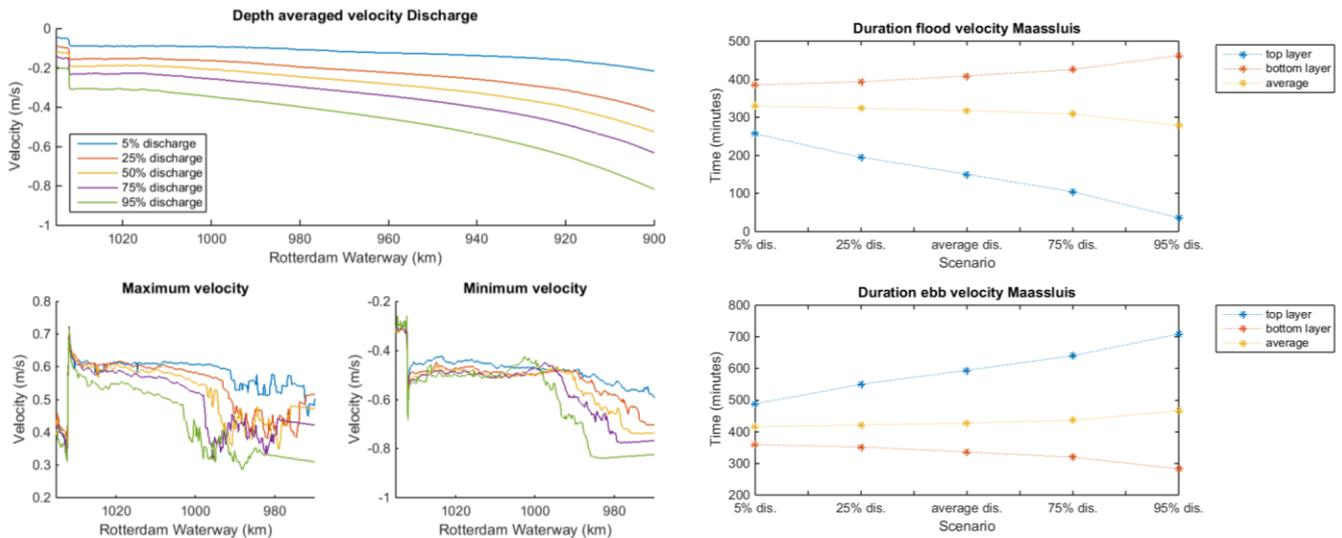
Figure 33 Left upper panel: depth average discharge; Lower left panel maximum (flood) velocity; Lower right panel minimum (ebb) velocity
