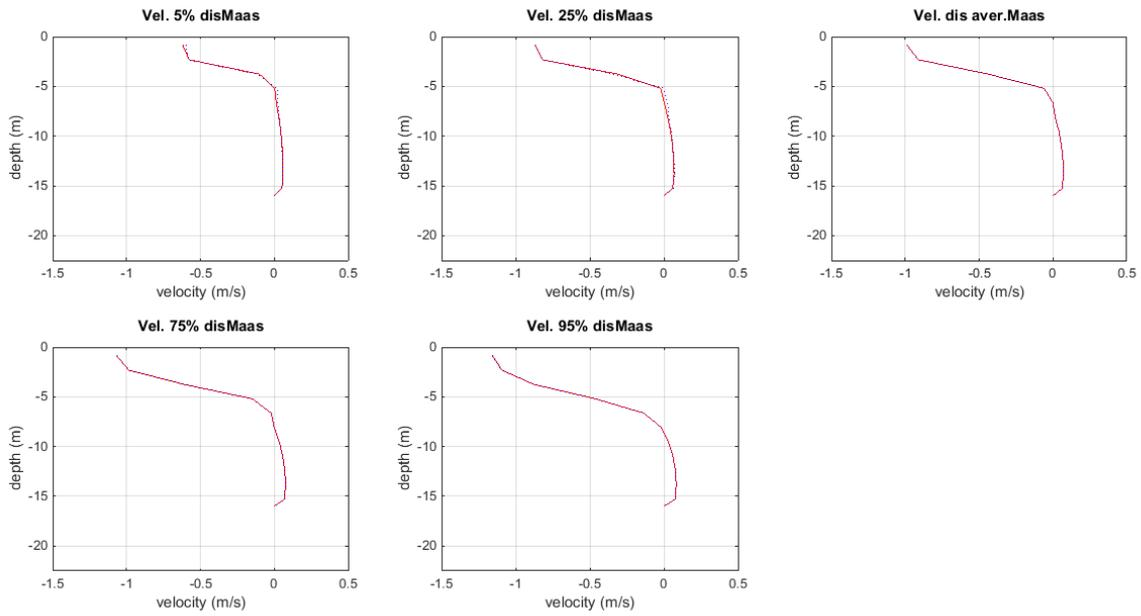
Figure 149 Changing average discharge for changing discharge near Maassluis due to ETM deepening
