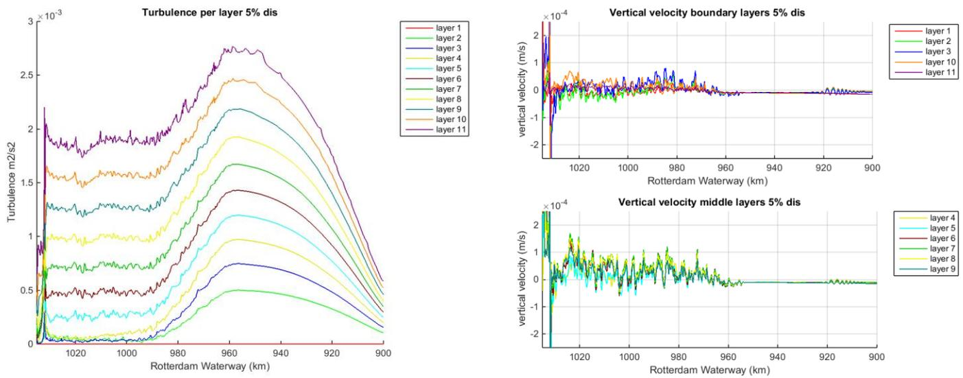
Figure 112 Turbulence (left) and vertical velocity for boundary layers and middle layers for 5% discharge
