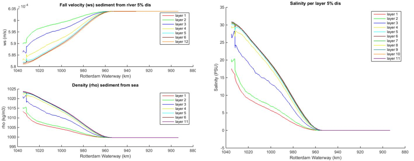
Figure 151 Fall velocity and density (left) and salinity (right) for the ETM deepening scenarion 5% discharge
