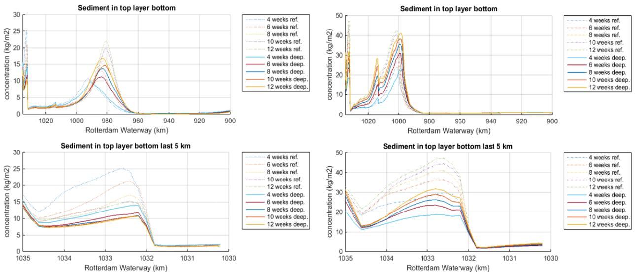
Figure 74 Bottom sediment active top layer for the 5% discharge (left) and 95% discharge (right)
