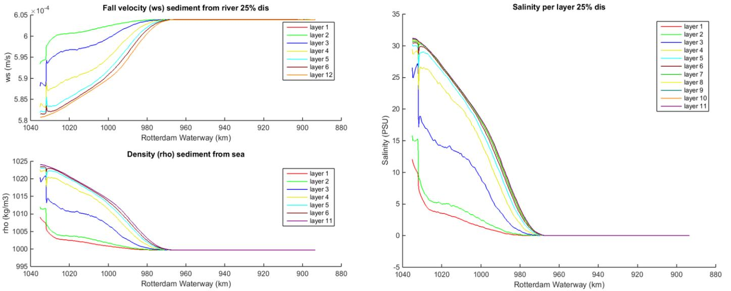
Figure 114 Fall velocity and density (left panels) and salinity for 25% discharge (right)
