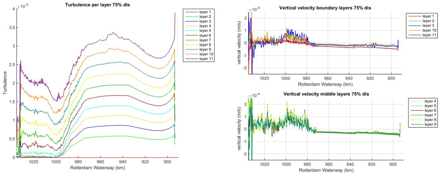
Figure 158 Turbulence (left) and vertical velocity for boundary layers and middle layers for 75% discharge
