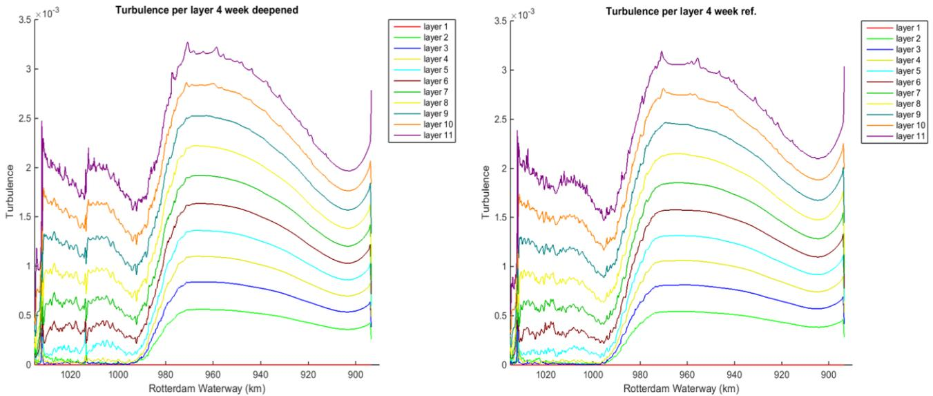
Figure 56 Turbulence for the step deepening scenario (left) and the reference scenario
