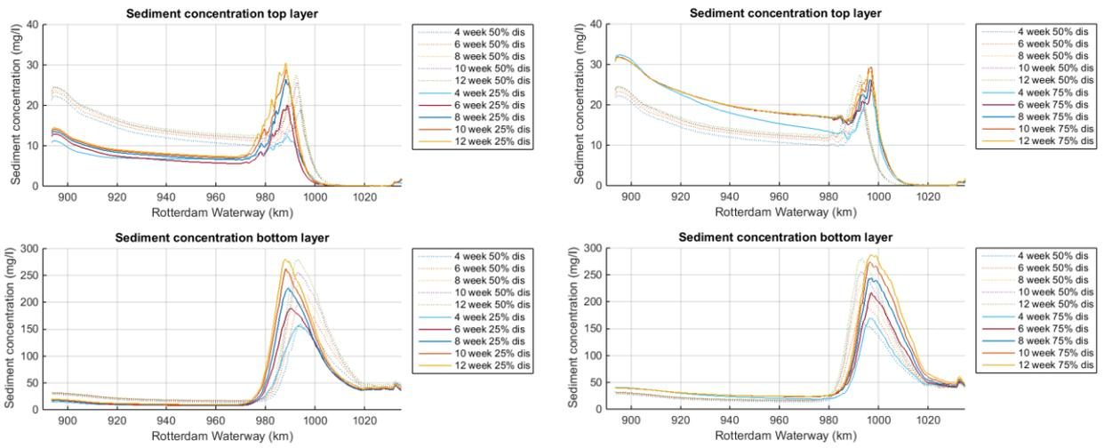
Figure 110 Bottom sediment in time for 25% discharge left and 75% discharge right
