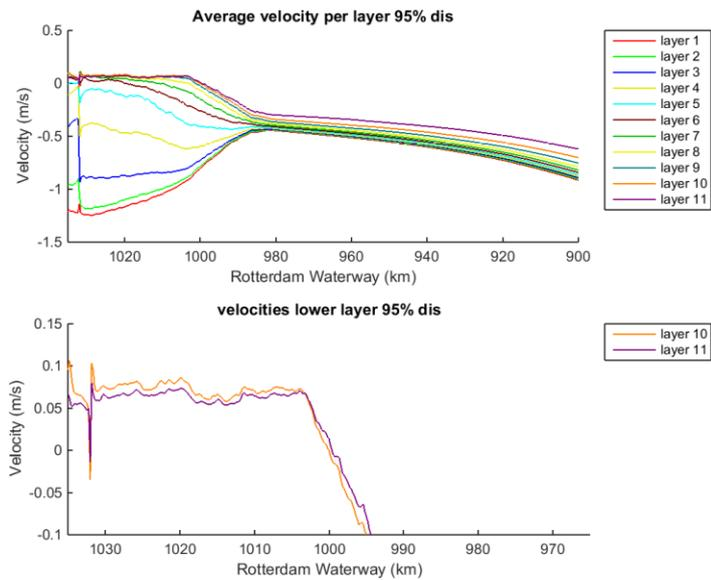
Figure 122 Average velocity per layer for 95% discharge (upper panel) and lowest two layers (lower panel)
