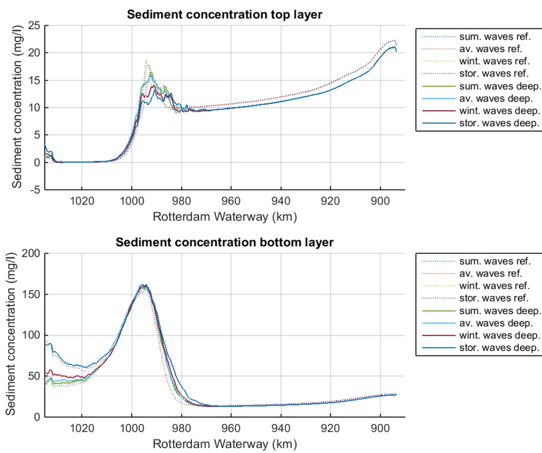
Figure 83 Sensitivity ETM due to changing waves for the ETM deepening, compared with the reference scenario (dashed lines)
