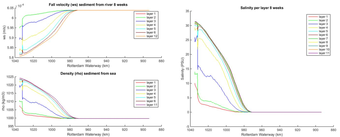
Figure 103 Fall velocity, density and salinity per layer for average discharge
