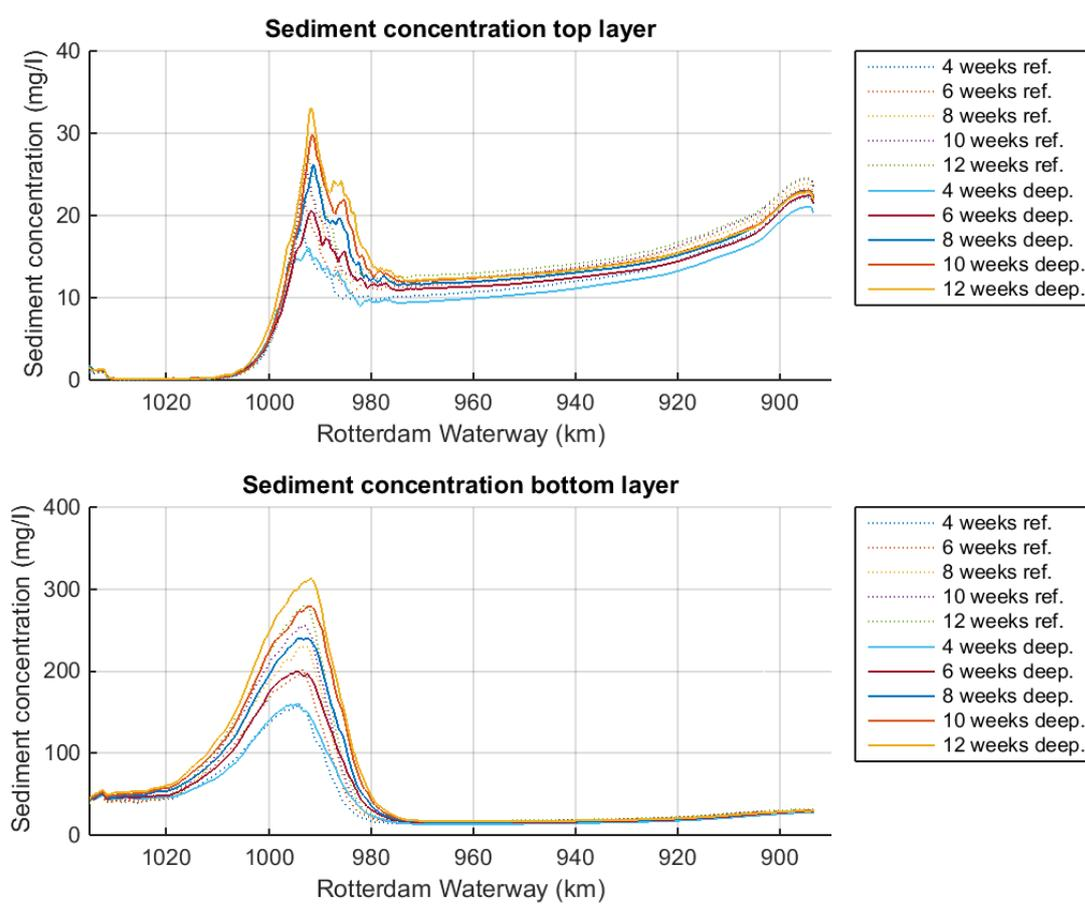
Figure 64 Suspended sediment concentration near the bottom and in the top layer for the deepened scenario compared with the reference scenario
