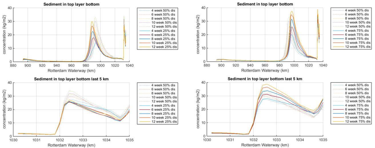
Figure 128 Fine sediment concentration in top layer bottom for 25% discharge (left panel) and 75% discharge (right panel)
