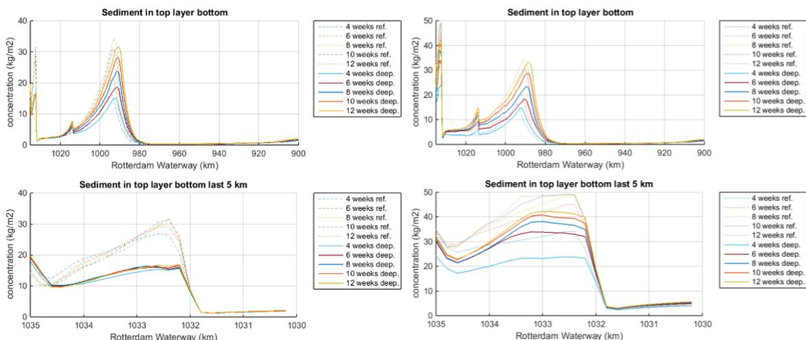
Figure 76 Available sediment bottom layer for summer waves (left) and storm waves (right)
