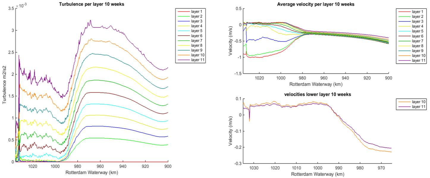
Figure 106 Turbulence in the Rotterdam Waterway on the left; Velocity per layer in the upper right figure; velocity profile of the near bed layers in the lower right panel. Positive velocity indicates flood, a negative velocity indicates ebb
