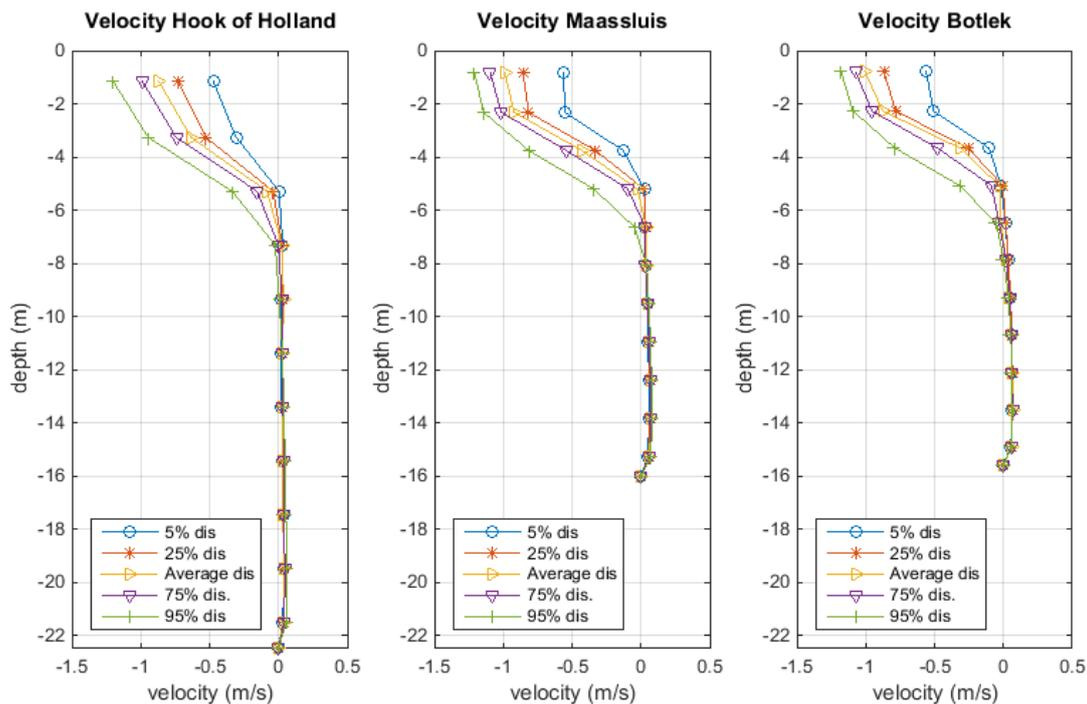
Figure 67 Average velocity for Hook of Holland, Maassluis and the Botlek for the changing discharge
