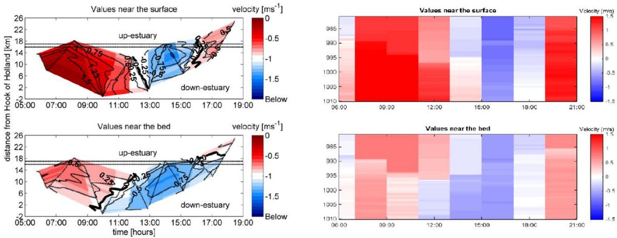
Figure 20 Left panel: Velocity measured by de Nijs et al. (2010). Right panel: calculated velocity with 4 weeks run up time
