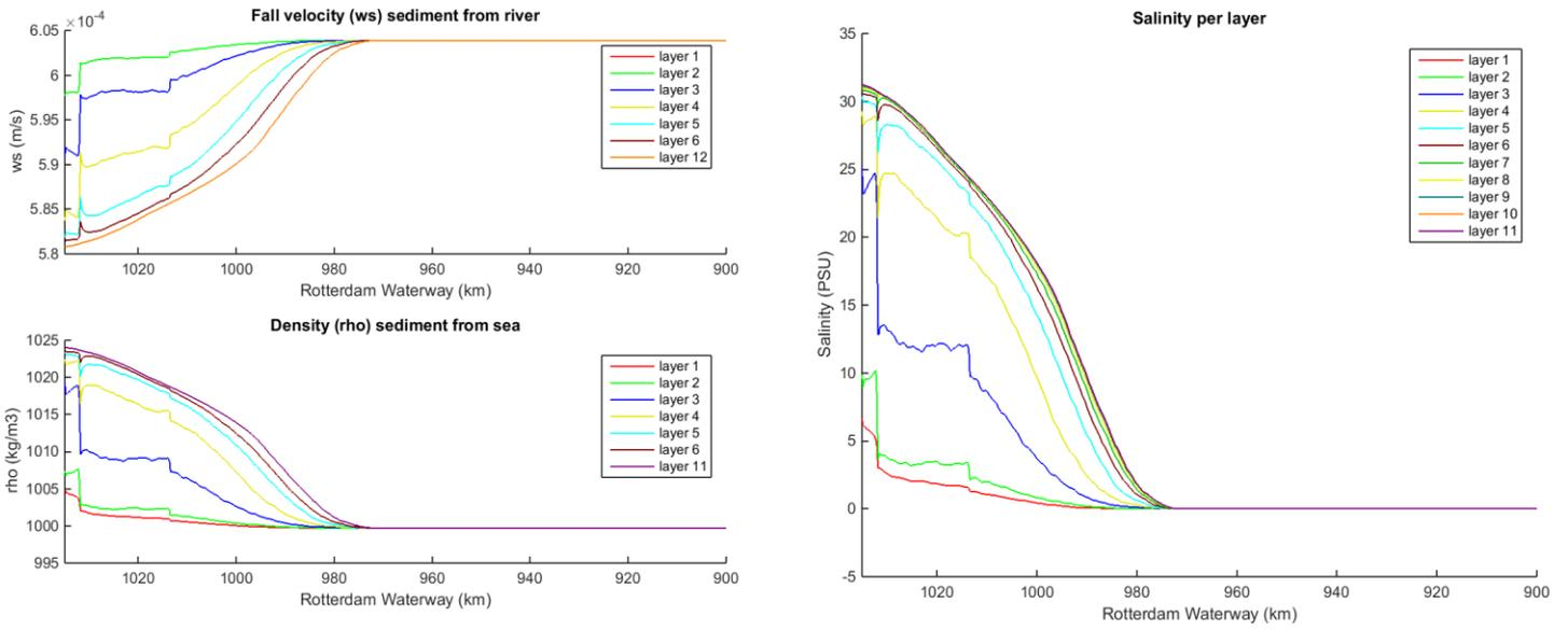
Figure 143 Fall velocity, density and salinity per layer for the deepened scenario
