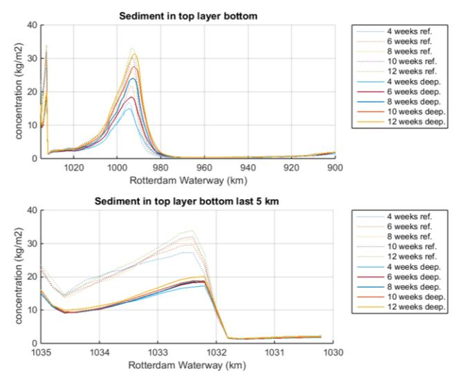
Figure 65 Available sediment in active top layer bottom for step deepening scenario (left) and ETM deepening scenario (right)
