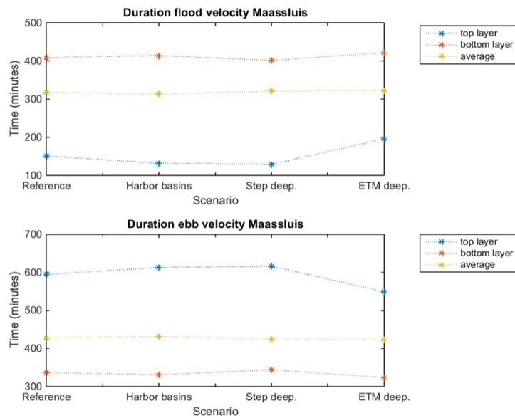
Figure 52 Ebb and flood velocity duration for different scenarios near Maassluis (km 1021.8)
