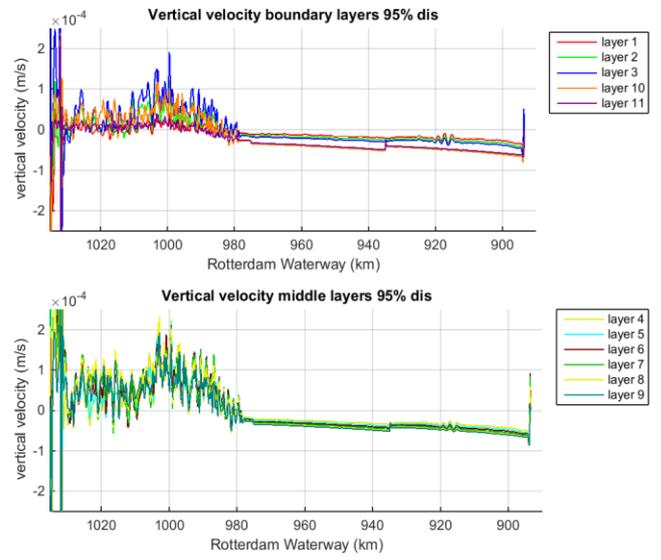
Figure 161 Turbulence (left) and vertical velocity for boundary layers and middle layers for 95% discharge
