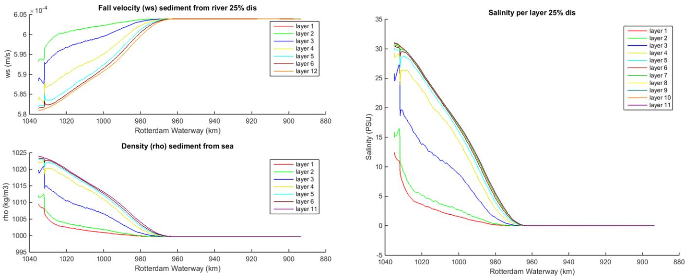
*Figure 154 Fall velocity and density (left) and salinity (right) for the ETM deepening scenario 25% discharge*
