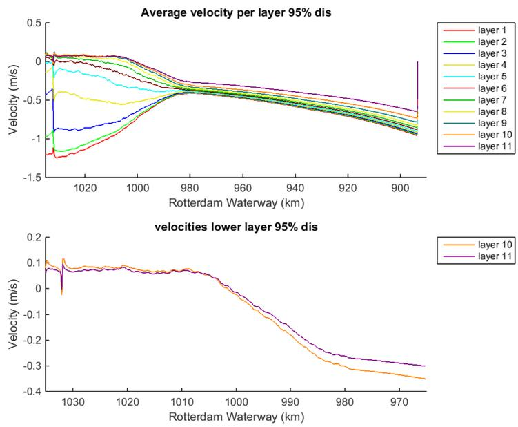
Figure 162 Average velocity for all layers (upper panel) and for the lowest two layers for the 95% discharge
