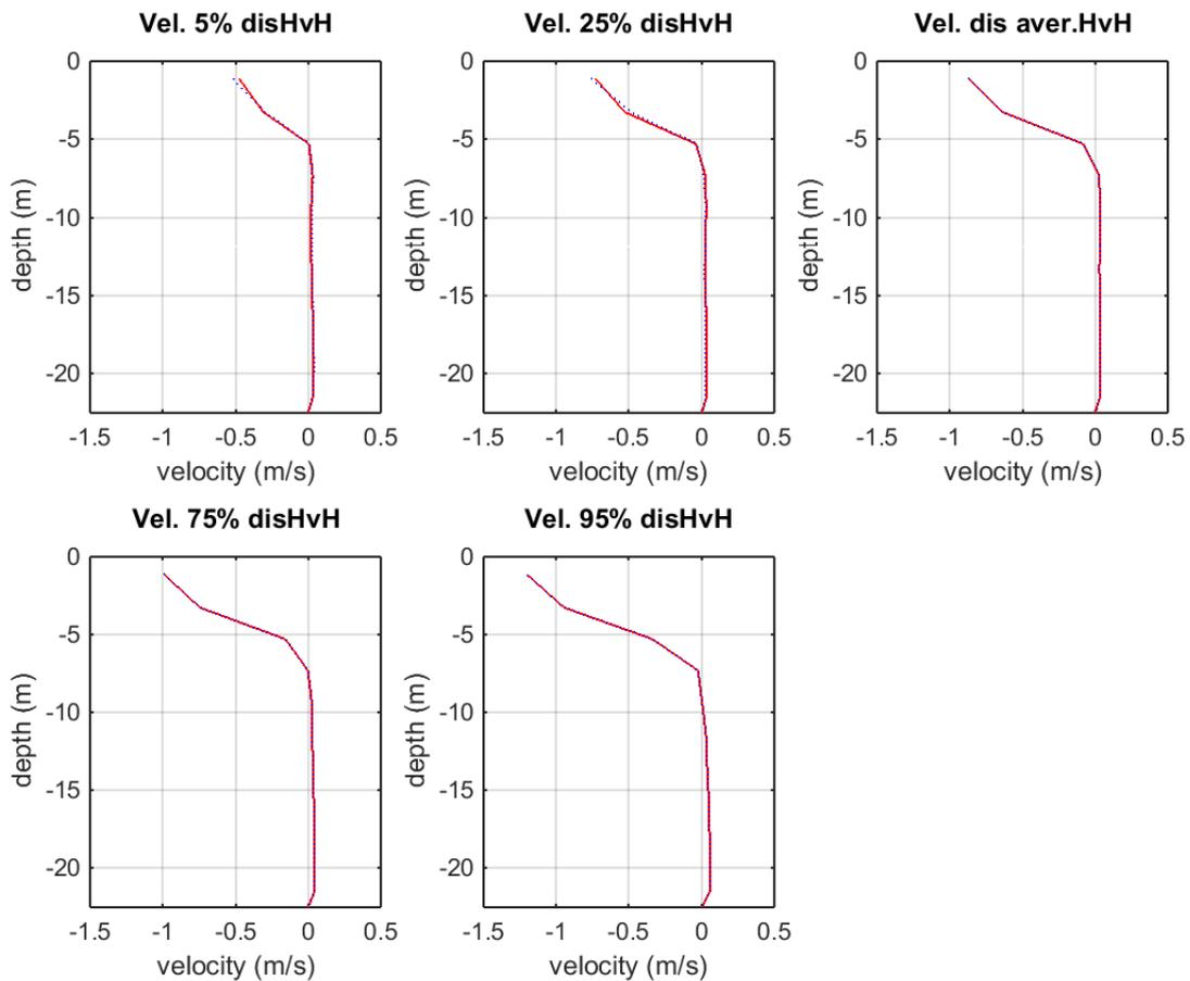
Figure 133 Change in velocity due to changing discharge for the reference scenario (dashed blue line) with the step deepening scenario (in red)
