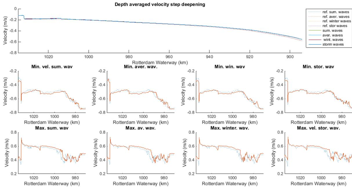
Figure 70 Depth average velocity (upper panel); Average ebb and flood velocities near the bed (lower panels) due to changing waves for the reference scenario (dashed blue) and the step deepening scenario (orange)
