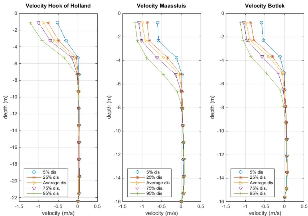
Figure 32 Average velocity for the discharge sensitivity for Hook of Holland (km 134.6), Maassluis (km 121.8) and Botlek (km 1009.6)
