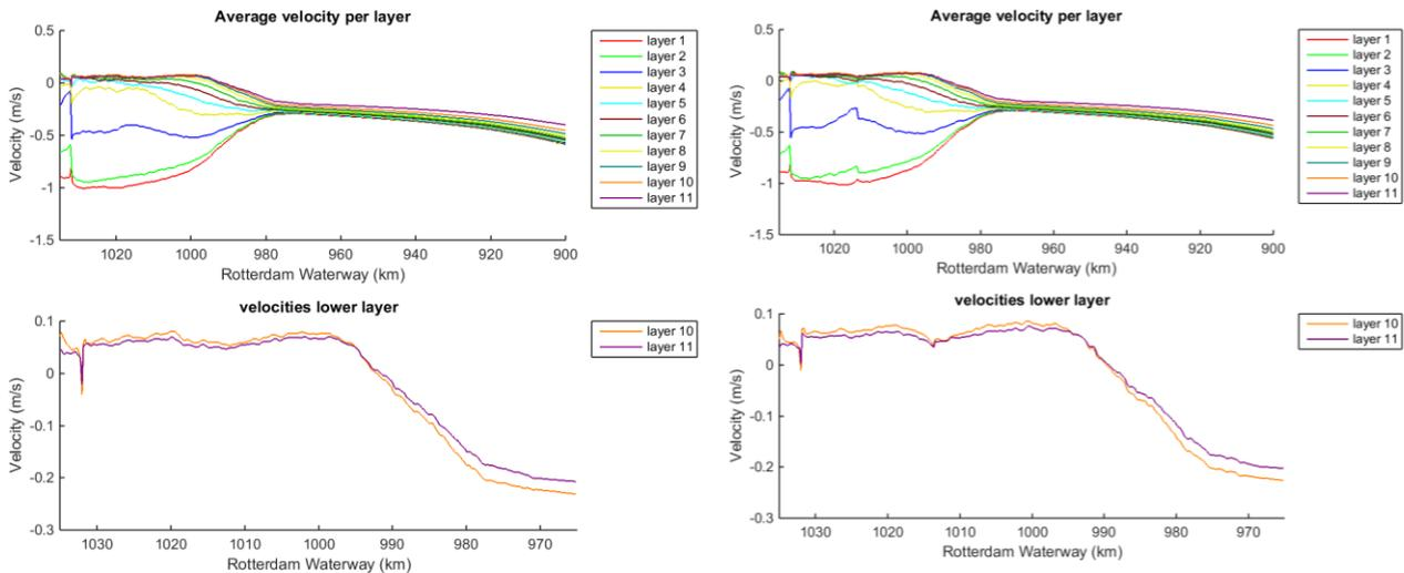
Figure 53 Average velocity for the reference scenario (left) and the step deepening scenario (right)
