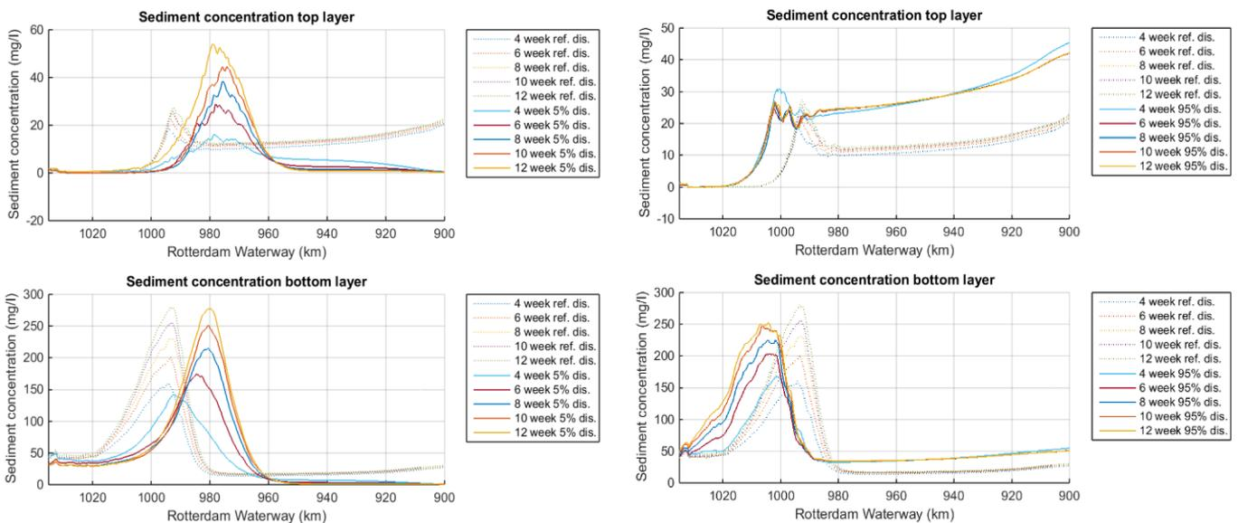
Figure 37 Long term response of the sediment in the ETM for 5% discharge in the left panel and 95% discharge for the right
