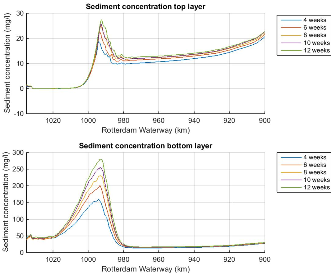
Figure 28 Tide averaged concentration SPM in time near the surface (top panel) and near the bottom (lower panel)
