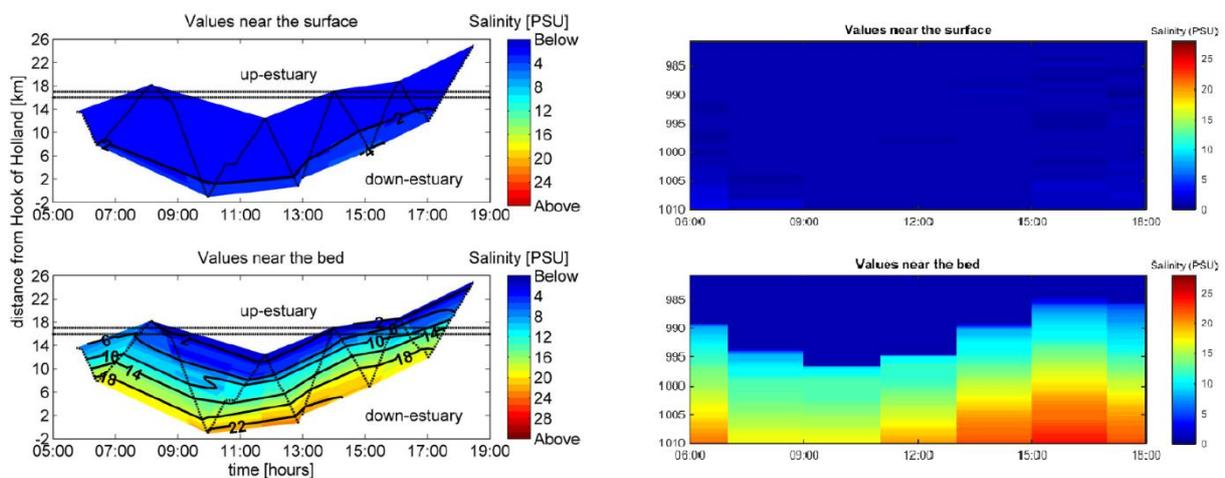
Figure 19 Left panel: Salinity measured by de Nijs *et al.* (2010). Right panel: calculated salinity with 4 weeks run up time
