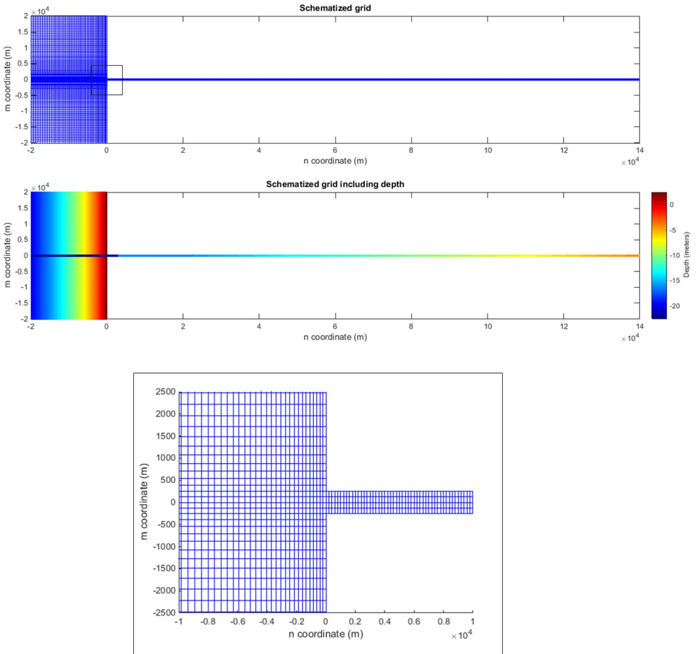
Figure 15 Schematized grid Rotterdam Waterway
