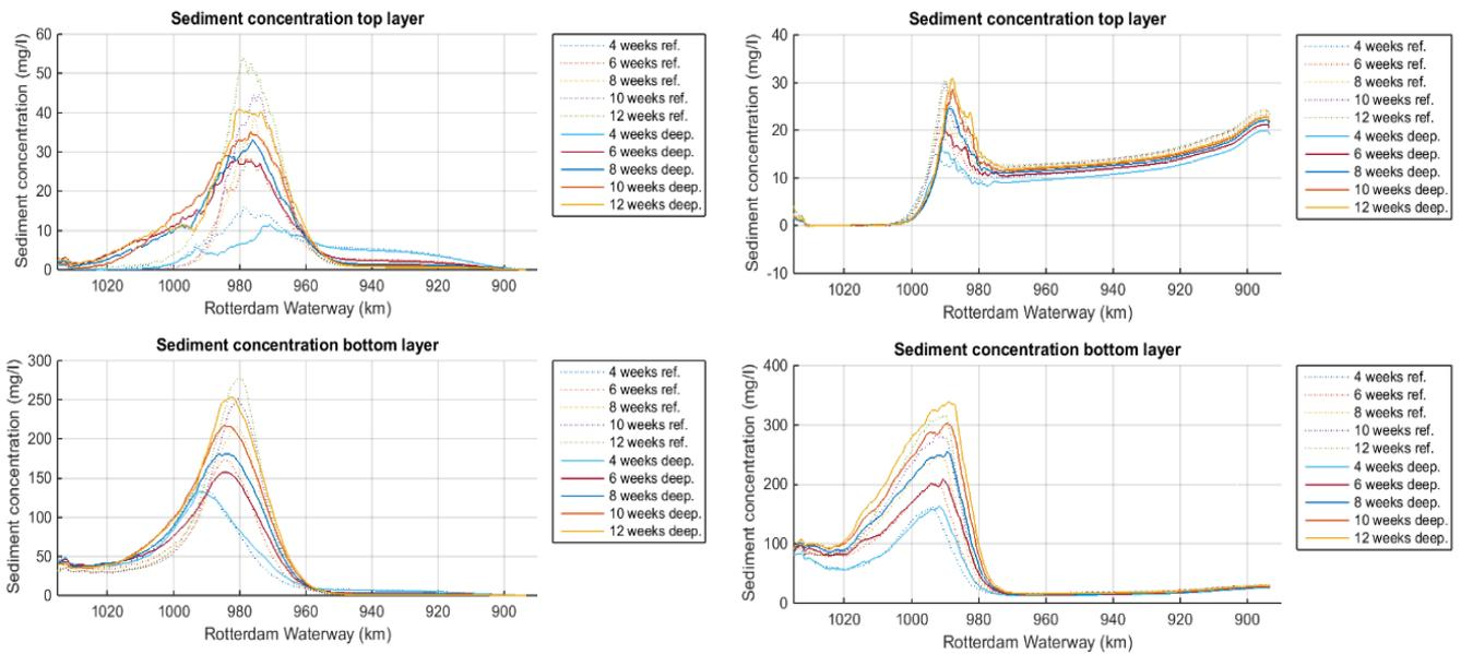
Figure 73 Medium term change due to 5% discharge (left) and 95% discharge (right) for the top layer (upper panels) and the near bed layer (lower panels) for the reference scenario (dashed line) and the step deepening scenario
