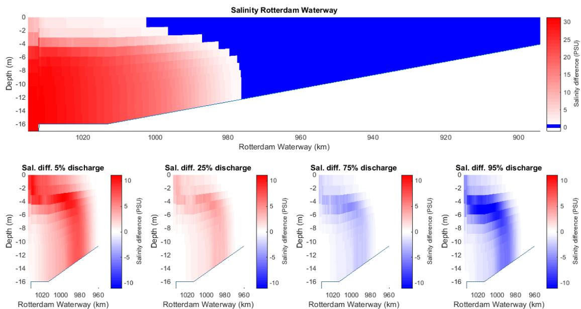
Figure 31 Salinity of the reference case (upper panel); Salinity difference for the 5% discharge (lower left panel); Salinity difference between reference case and 95% discharge (lower right panel)
