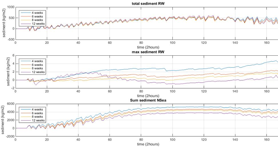
Figure 109 Growth of the sediment in bottom layer (upper panel); The growth of the peak of the ETM (middle panel); Growth of sediment at North Sea (bottom panel)
