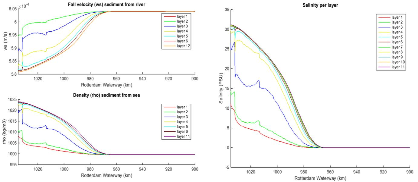
Figure 139 Fall velocity, density and salinity per layer for the deepened scenario
