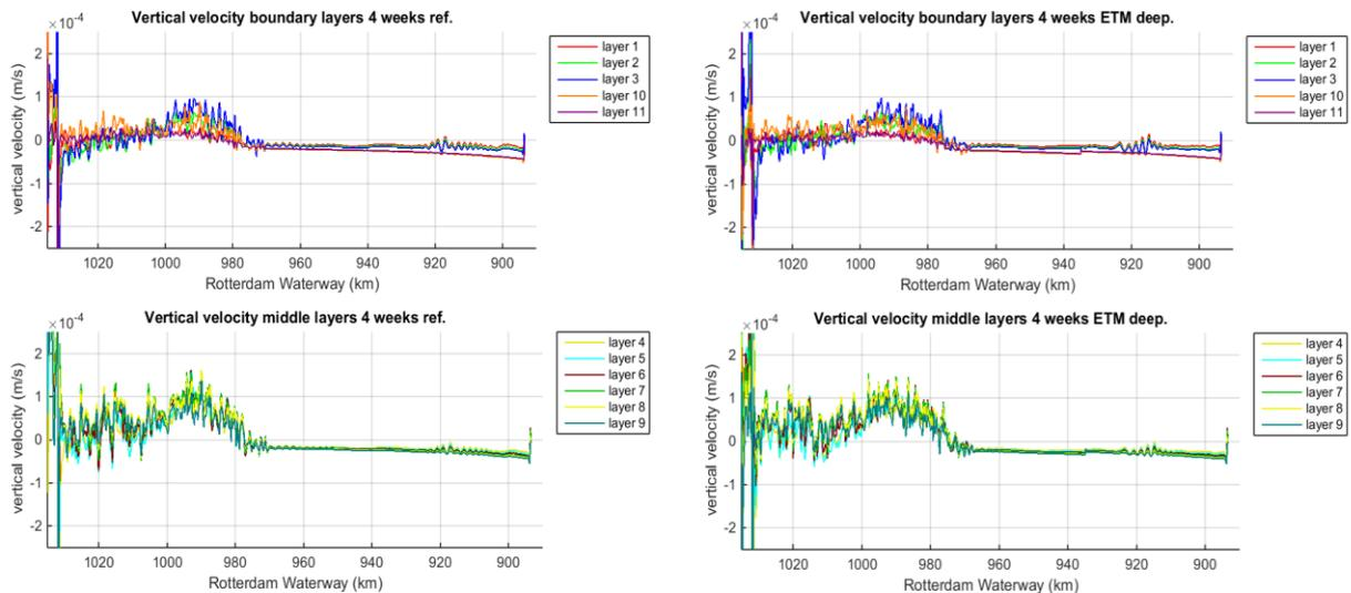
Figure 59 Gravitational circulation for the reference situation (left) and the ETM deepening scenario (right)
