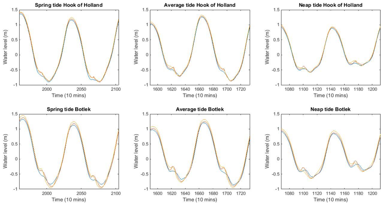
Figure 94 Water levels Hook of Holland and Maassluis for discharge sensitivity with 5% discharge in blue, average discharge in orange and 95% discharge in yellow for the step deepening scenario
