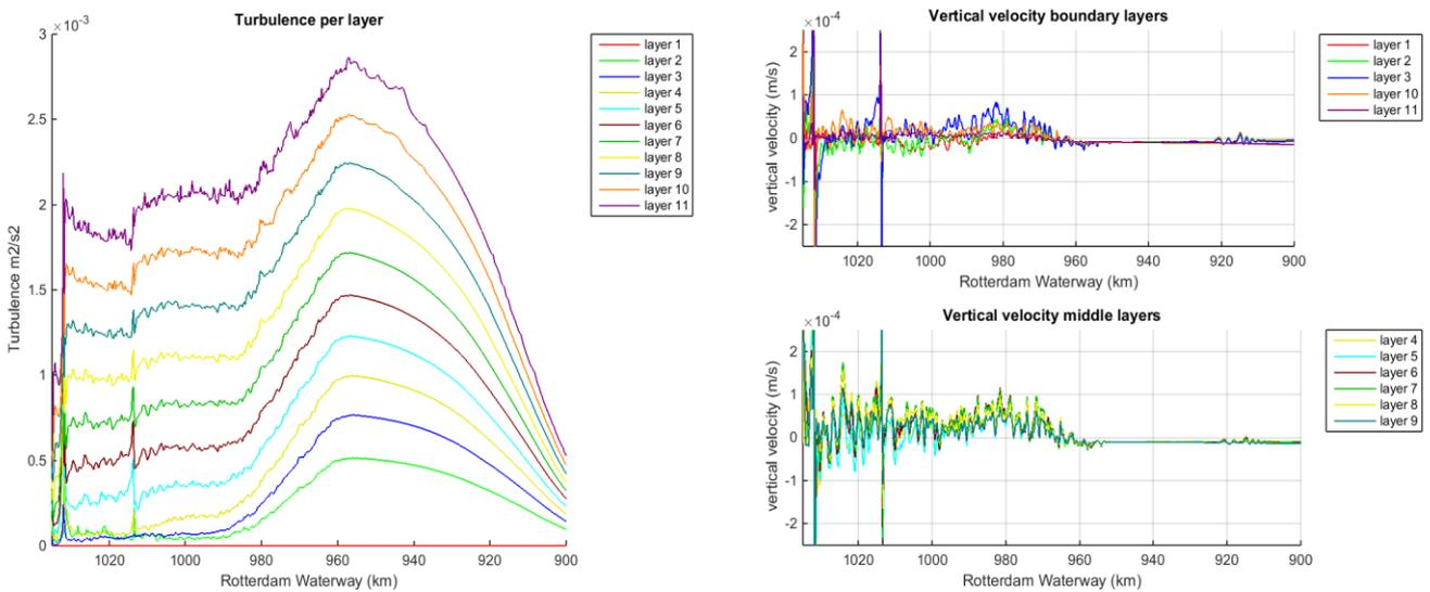
Figure 137 Turbulence, average velocity for all layers and specific for the two lowest layers
