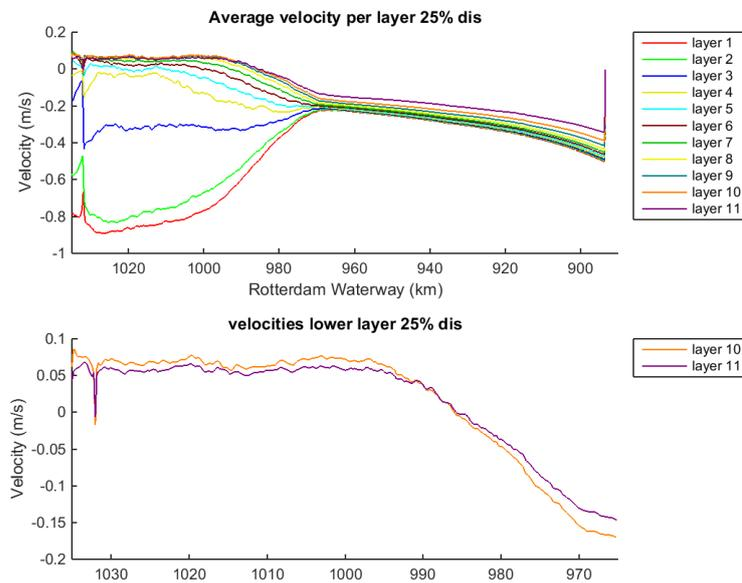
Figure 156 Average velocity for all layers (upper panel) and for the lowest two layers for the 25% discharge
