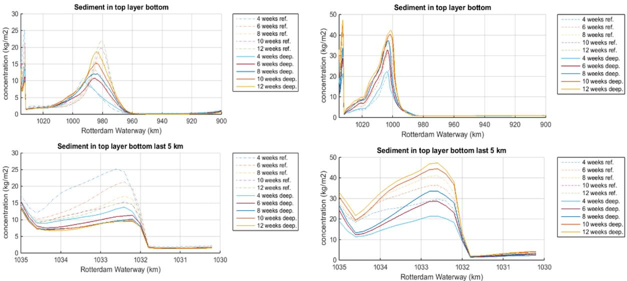
Figure 85 Available sediment in bottom layer for 5% discharge (left) and 95% discharge (right) for the ETM deepening scenario and the reference scenario (dashed lines)
