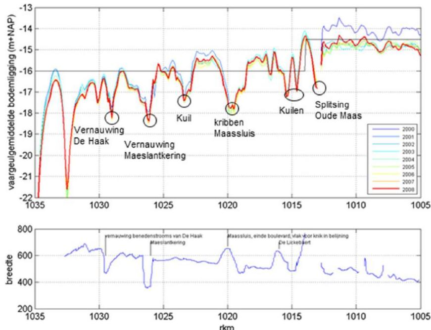
Figure 9 Bathymetry (upper panel) and the width (lower panel) of the Rotterdam Waterway (van Dreumel *et al.*, 2010)
