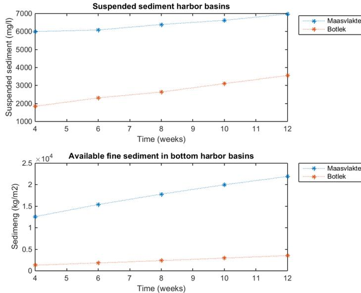
Figure 49 Total suspended sediment (upper panel) in the harbor basins; Total average fine sediment in top layer bottom (lower panel)
