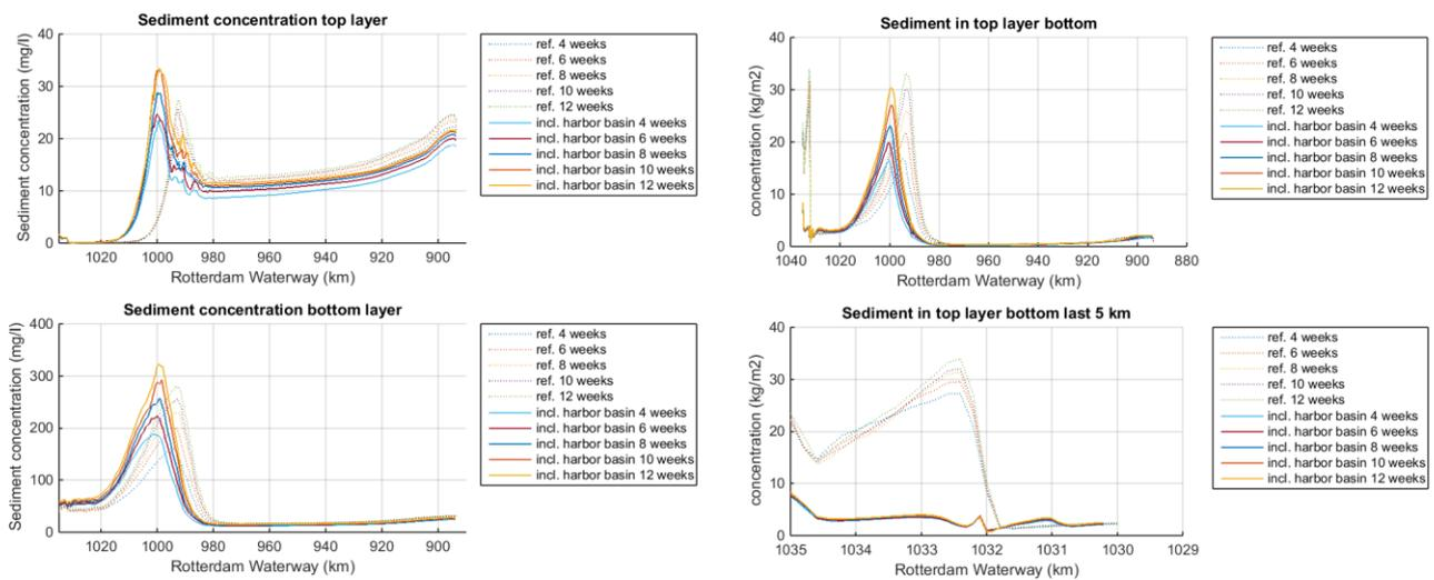
Figure 48 Sediment in the top and near bottom layer for the water column (left); Sediment in top layer bottom (right)
