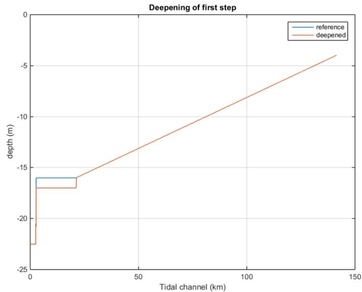
Figure 23 Deepened depth vs. original depth
