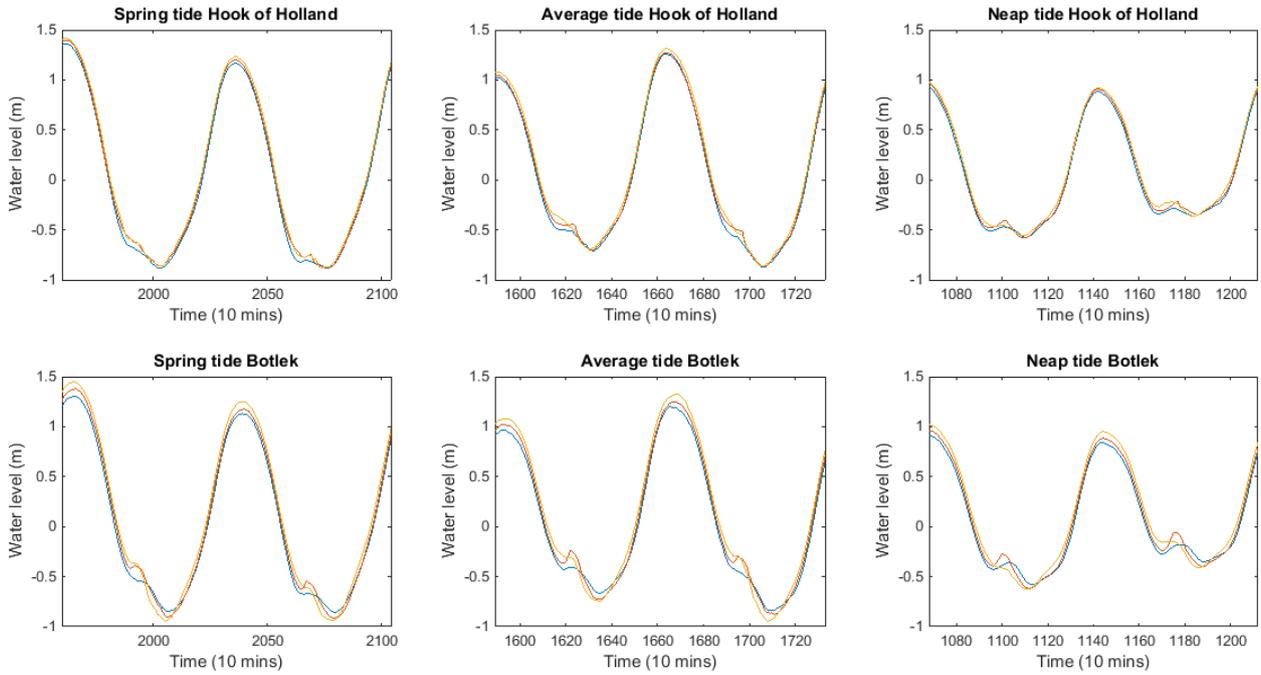
Figure 90 Water levels Hook of Holland and Maassluis discharge sensitivity with 5% discharge in blue, average discharge in orange and 95% discharge in yellow
