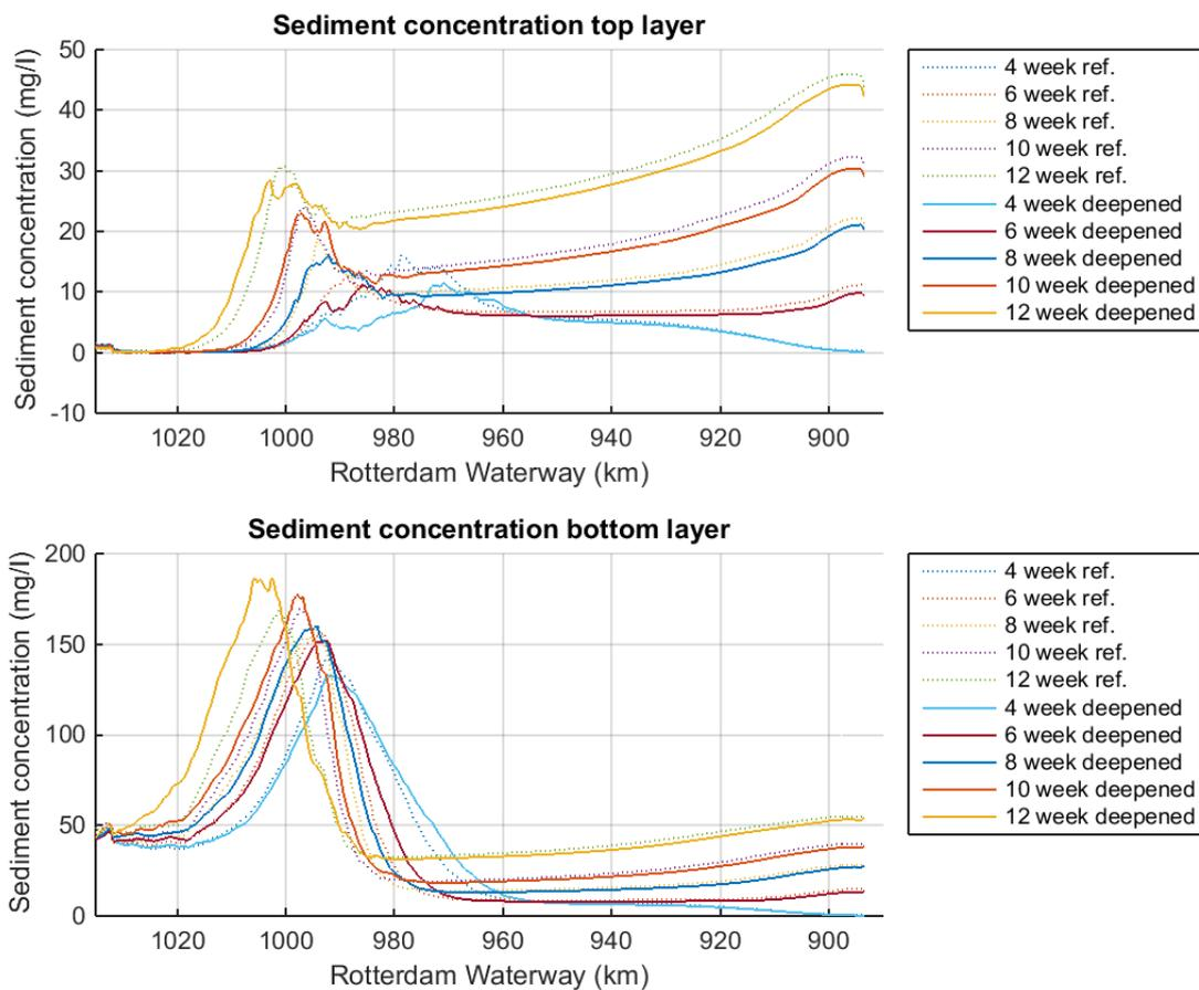
Figure 82 Sensitivity ETM deepening for changing discharge for the ETM deepening scenario, compared with the reference scenario (dashed lines)
