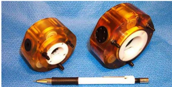
**Figure 2.3:** The “PneuStep” actuator comes in two sizes
