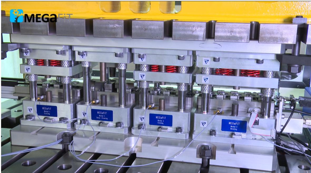
**Figure 2.1:** Test setup for production of the demonstrator product as used in the MEGaFit project.
