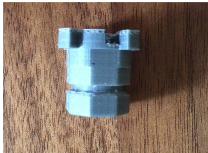
Figure 76: Printed container with visible excess material in the groove
