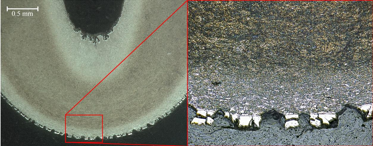
**Figure 3.16** *Micrograph of unetched buckling bending test specimen n1\_03 at a displacement of 36 mm with inset.*
