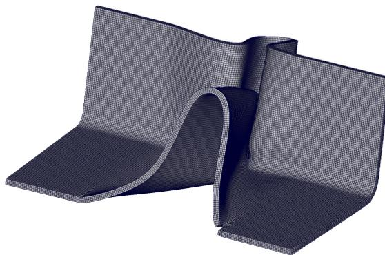
**Figure 5.8** *The 0.5 mm mesh with SRI and rotated base plate FE model with shear fracture above the clamped section.*
