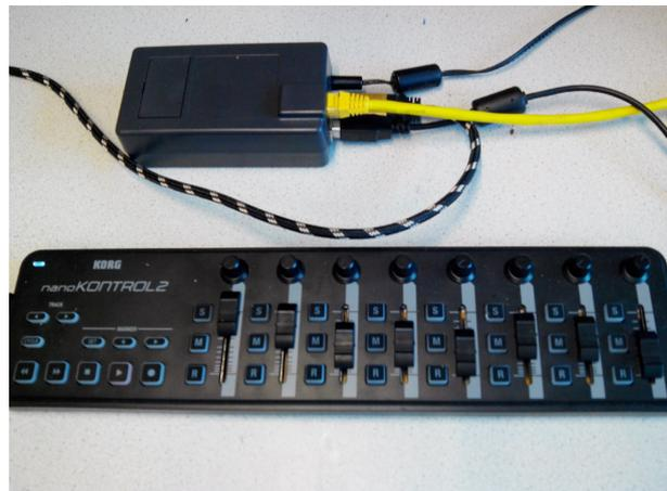
**Figure 3.3:** This image shows the KORG control board connected to a casing containing an Arduino ATmega, this is connected to the sensor vessel with the yellow Ethernet cable and to the laptop using usb.
