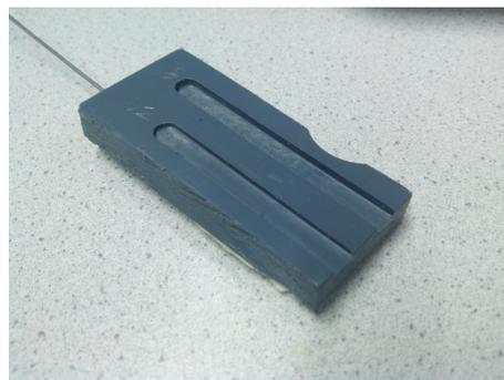
**Figure 4.2:** A picture of the used obstacle, showing two cuts one of 1.8 and 1.2 mm depth
