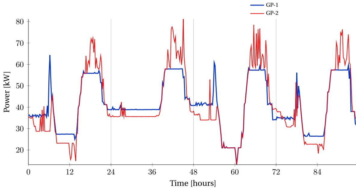
Figure 6.3: Ex1 - Transformer power profile to compare strategies with different prices for the device-off option
