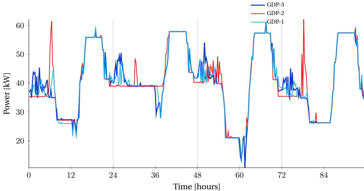
Figure 6.5: Ex2 - Transformer power profile of the bidding strategies with the device-off option on different prices.
