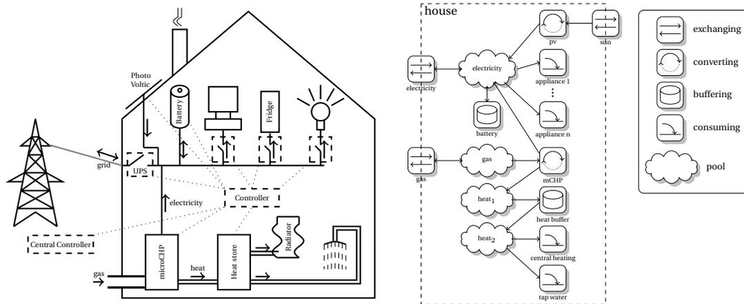
Figure 3.5: Left: drawing of a typical household. Right: its corresponding Triana model
