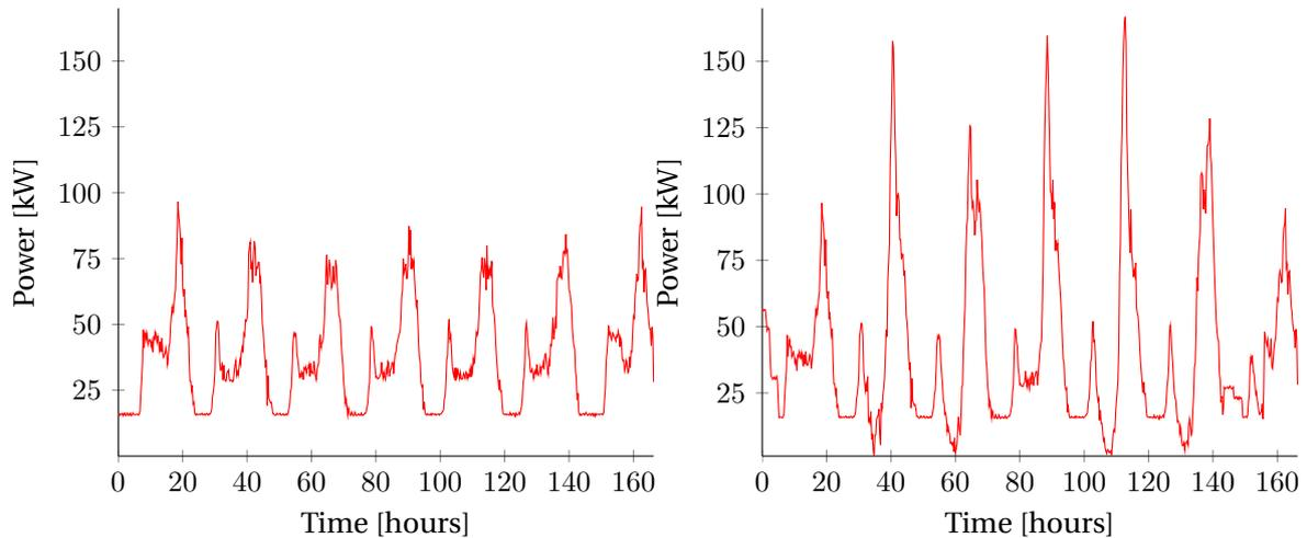
(a) Transformer power levels in the present situation. No EV, PV, batteries and control.
