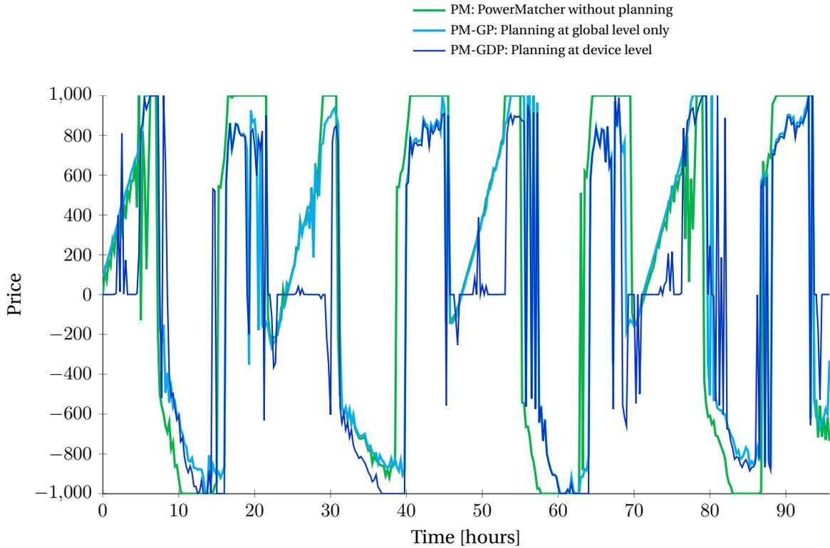
Figure 6.12: MCP/OSP of the three best simulation results from Experiment 1 and Experiment 2, together with The PowerMatcher results.
