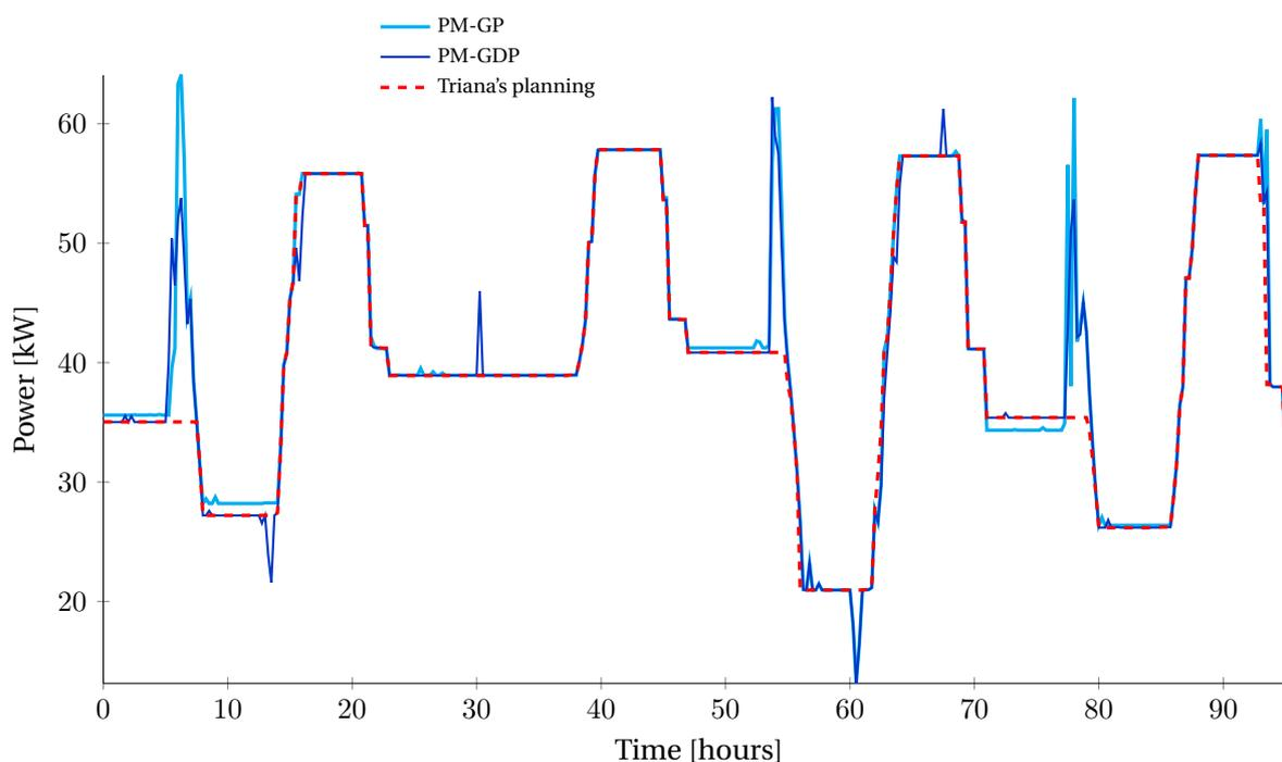
Figure 6.9: Ex3 - Transformer power profile of two bidding strategies, using a continuous MCP/OSP
