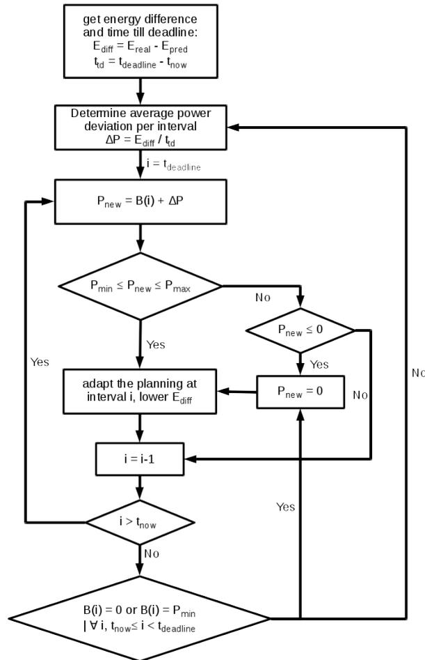
Figure 4.4: Flowchart of algorithm EP1: the deviations with respect to the planning are spread out over all time intervals till the deadline
