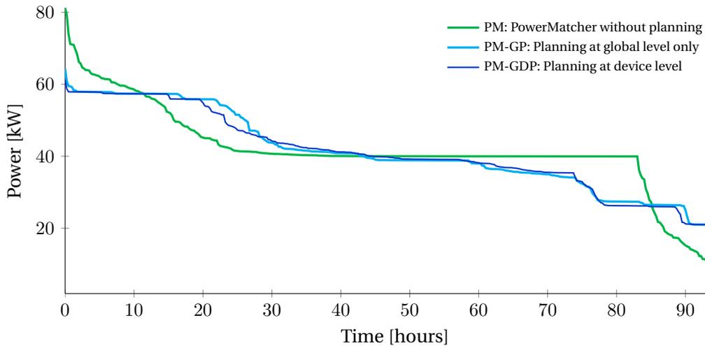
Figure 6.13: Load duration curve the of transformer power profile.
