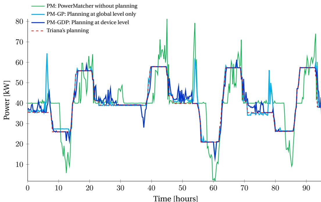
Figure 6.11: Transformer power profile of the three best simulation results from Experiment 1 and Experiment 2, together with The PowerMatcher results.
