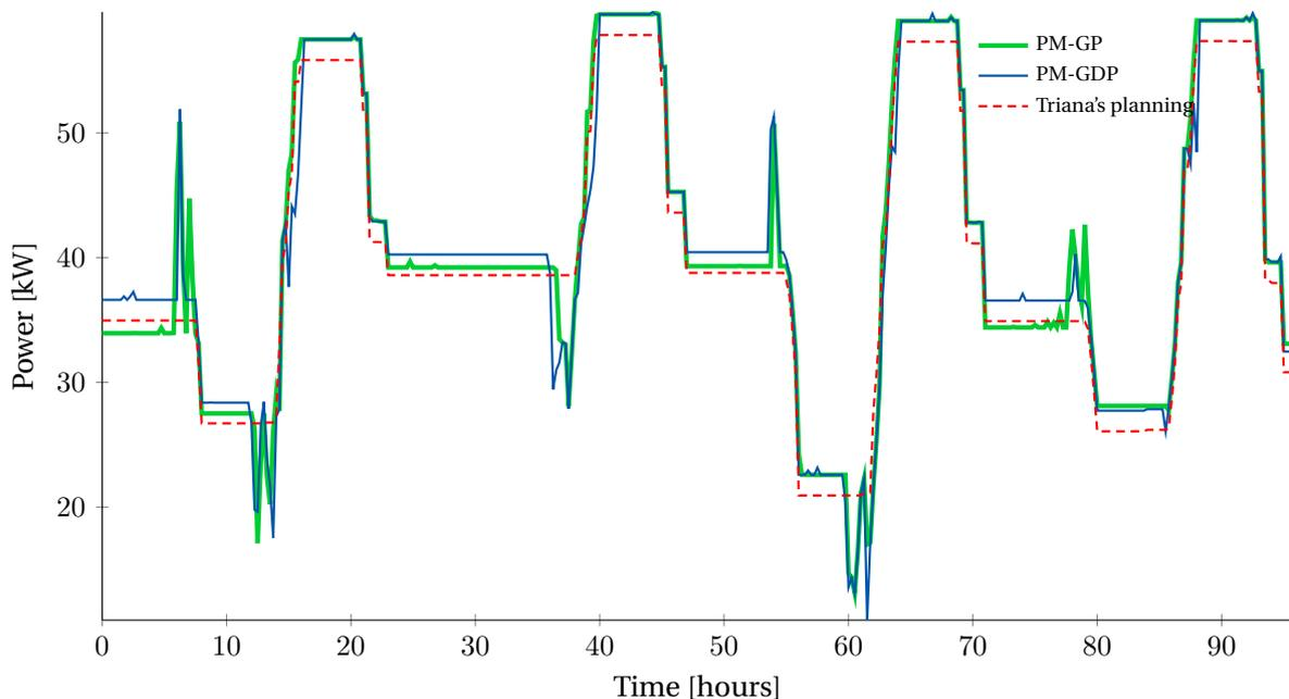
Figure 6.10: Ex5 - Transformer power profiles of the experiment with a continuous clearing price and energy compensation at the auctioneer.
