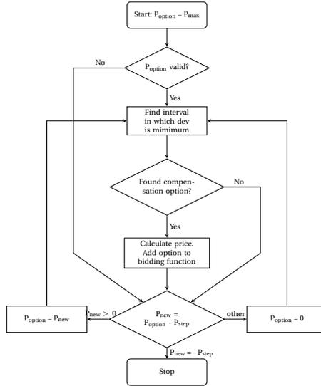
Figure 4.5: Flowchart of algorithm API: compose a bidding functions with options that lead to minimum deviation from the original planning
