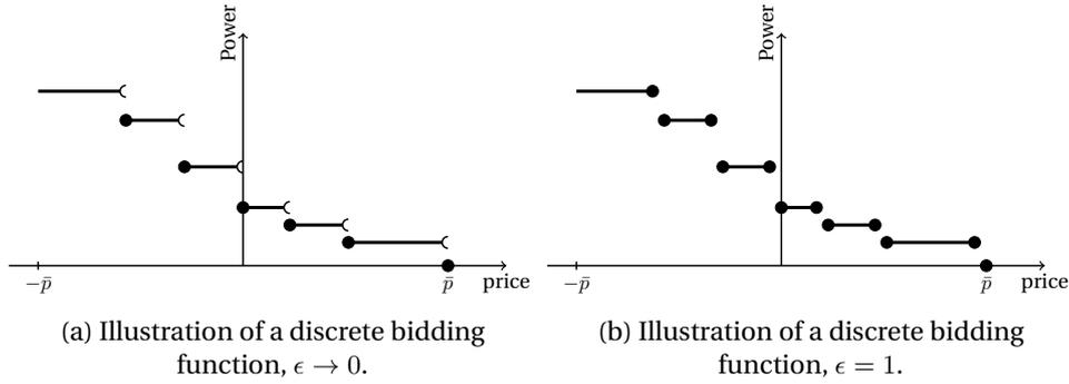
Figure 4.2: Discrete bidding function.
