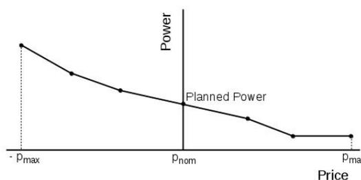
Figure 4.1: Basic illustration of a bidding function in the combined DSM approach
