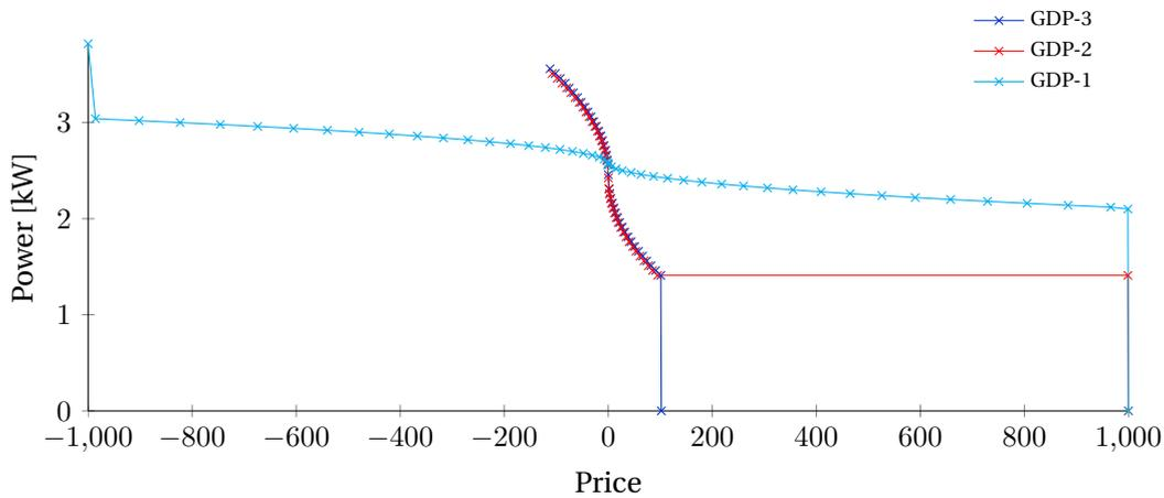
Figure 6.8: Ex2 - Comparing bidding functions of one EV on interval 192 (start of day 3).
