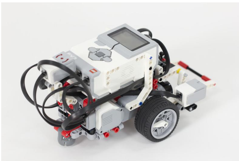
Figure 1. LEGO Mindstorms EV3 car.
