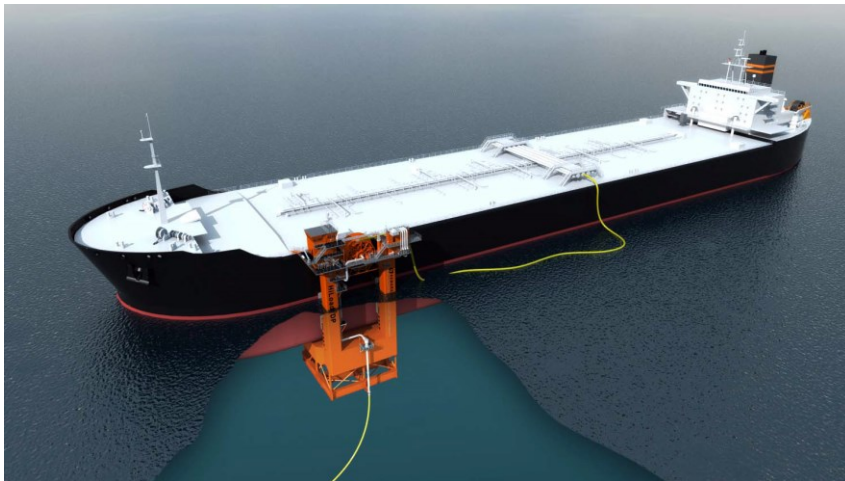
Figure 24 - Tanker docking system based on the remora adhesion mechanism.
