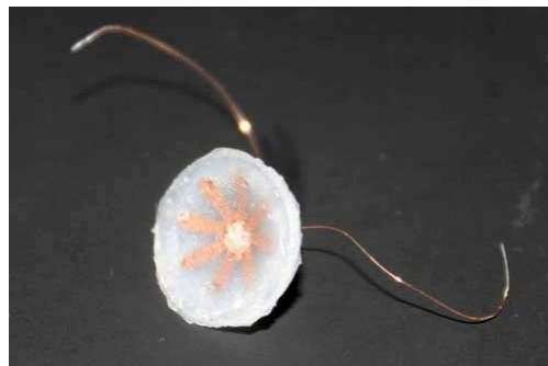
Figure 30 - Bionic leech sucker with ionic polymer–metal composites actuator Feng et al., 2014).
