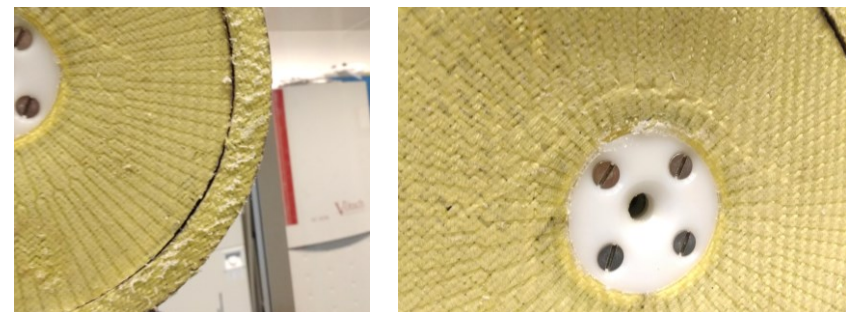
Figure 149 - Visual wear effects on the suction cup.
