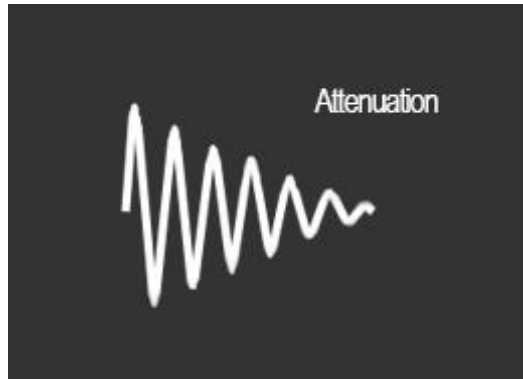
Figure 6: Schematic of the attenuation principle. The amplitude of a signal decreases over time.
