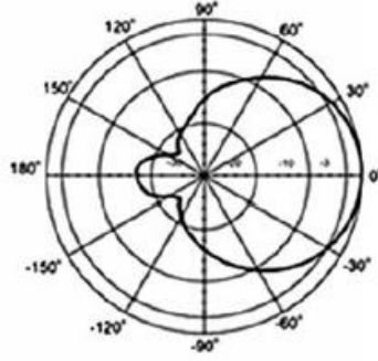
Figure 3: Schematic of the propagation of a signal from a directional antenna [3].
