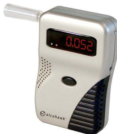
IMAGE 9: BREATHALYZER WITH SEMI-CONDUCTOR FROM 'ALCOHAWK'.
