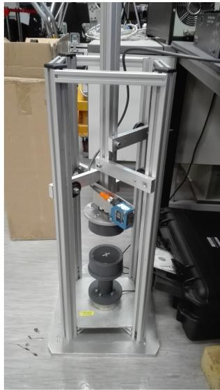
(a) Measurement rig to determine force between a pair of magnets
