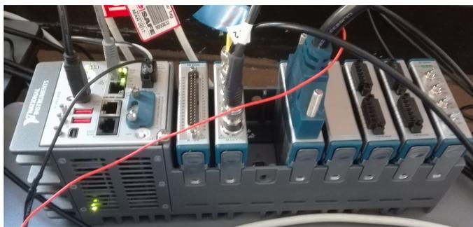
Figure 3.1: NI-cRIO 9035 with different modules
