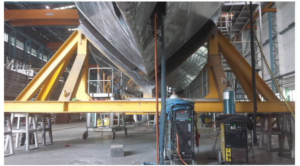
Figure 1: Traditional ship cradle used by DAMEN
