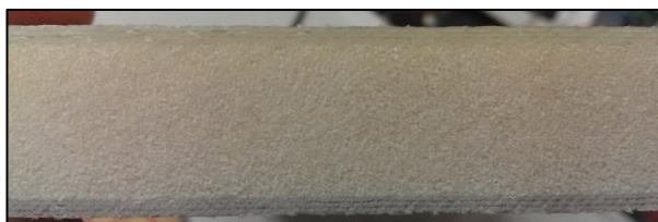
Figure 13: Sandwich specimen: two glass fibre skin and foam core
