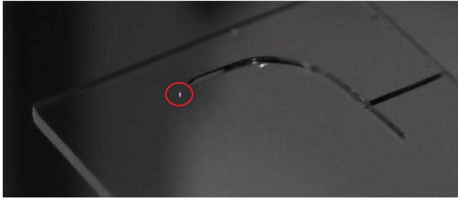
Figure 4.2: Visible white cylindrical spot when focusing the laser in the middle of a soda-lime glass sample. Laser parameters: Repetition rate=300 kHz, power=2.64 W, scanning speed=1 mm/s.
