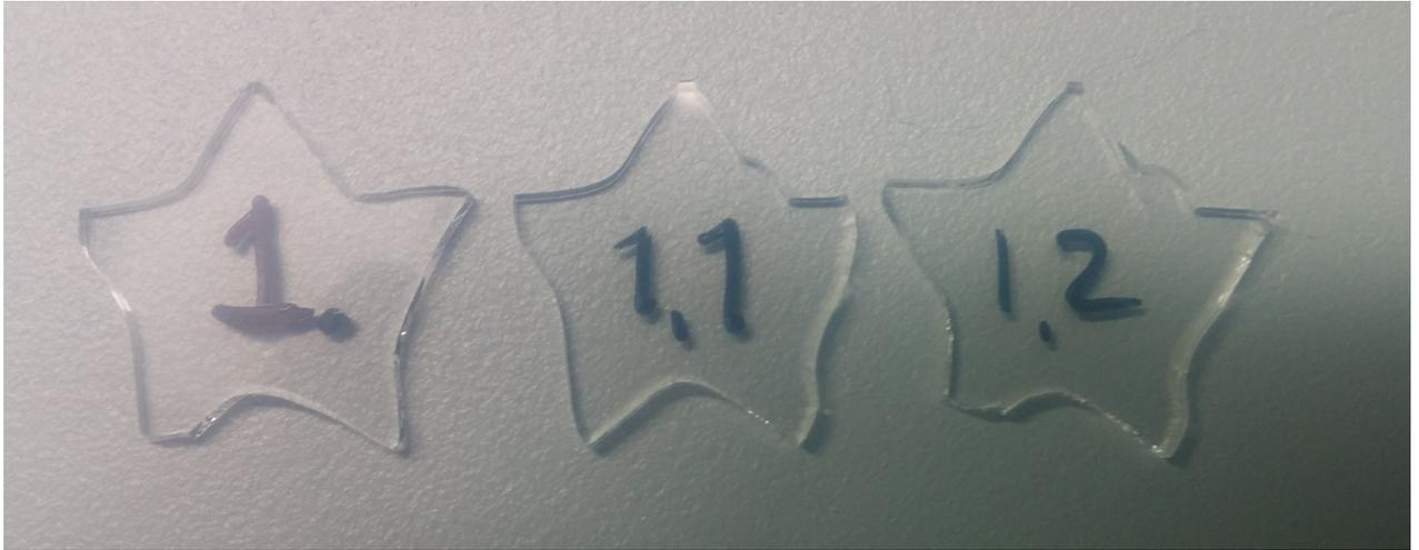
Figure 4.7: Soda-lime glass star shapes objects cut with the laser. Laser parameters: Repetition rate = 300 kHz, power=2.65 W, scanning speed = 0.5-1 mm/s, NA=0.04.
