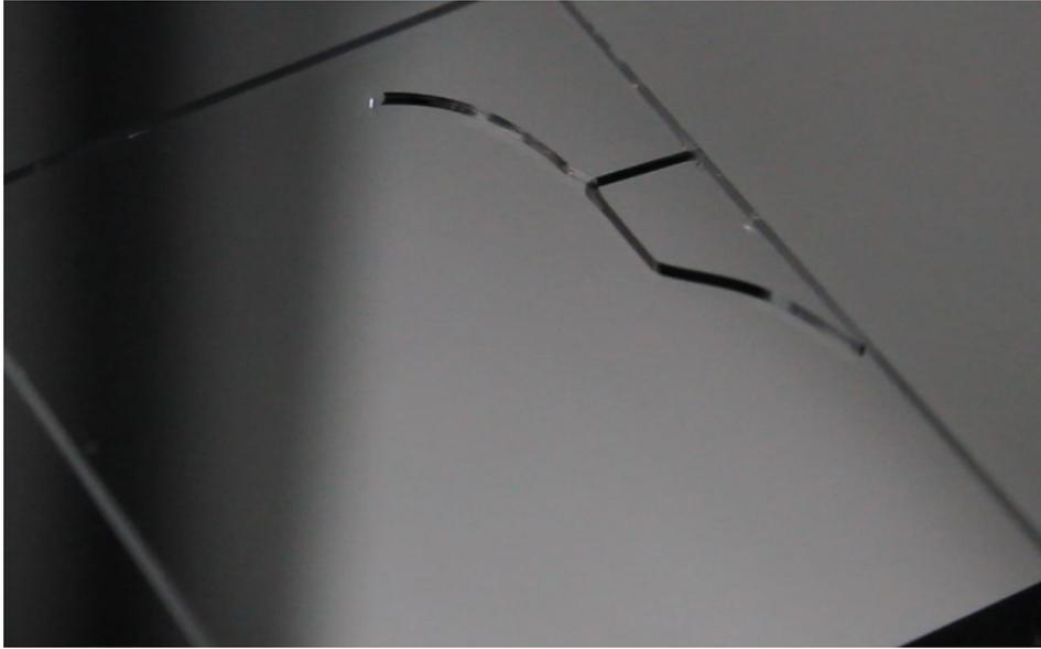
Figure 4.5: An initial cut in the glass is further cracked in the wrong direction by induced material stress. Laser parameters: Repetition rate = 300 kHz, power=2.65 W, scanning speed = 1 mm/s.
