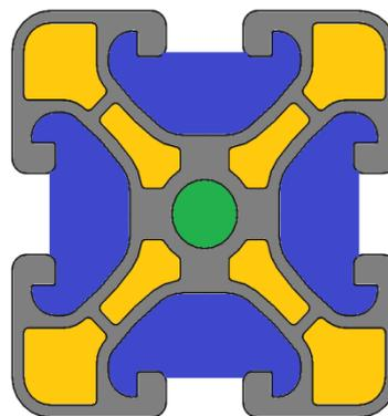
Figure 19: Cross section of aluminum profile "Profil 8 40x40 leicht natur"
