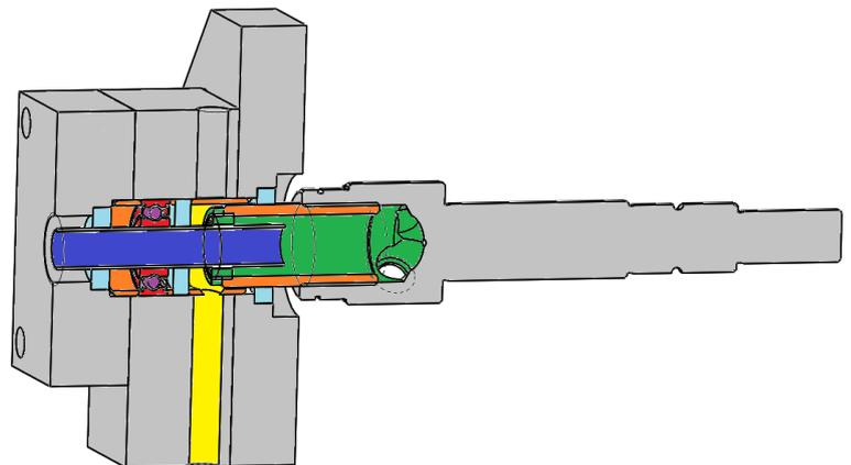
Figure 4: Schematic representation of old water supply system. inflow (dark blue), mix of in- and outflow (green) and outflow (yellow)
