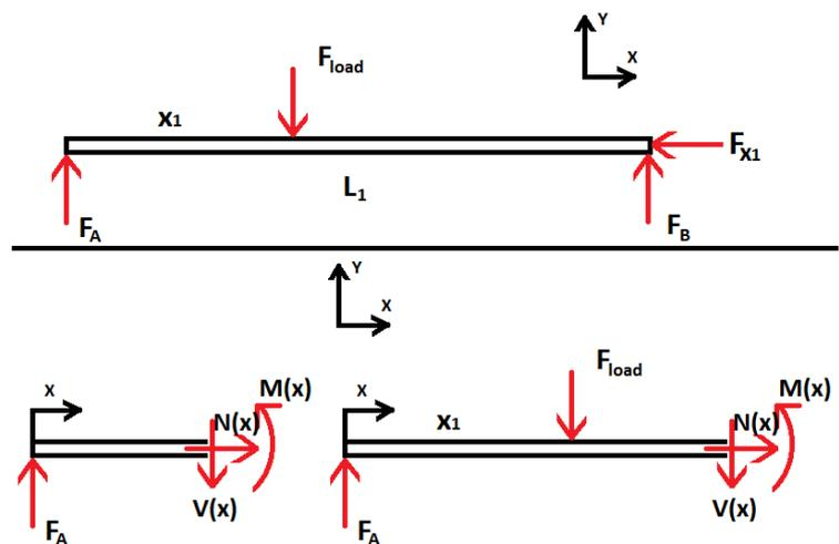
Figure 6: Free Body Diagram shaft
