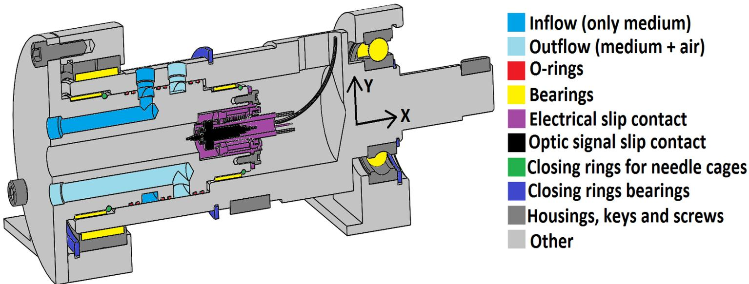
Figure 12: CAD designs of the power, medium and optical signal supply systems
