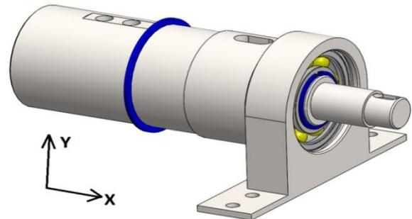
Figure 14: Mounting the simple ball bearing and wheel (wheel not displayed)
