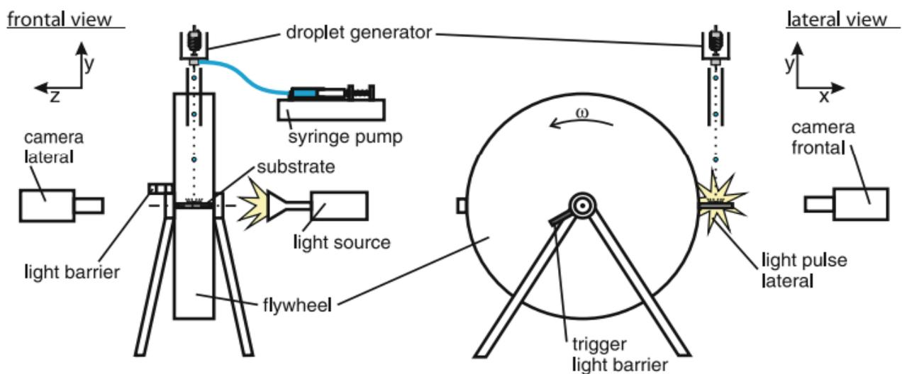
Figure 1: Experimental set-up by W.B. Faßmann (2013)
