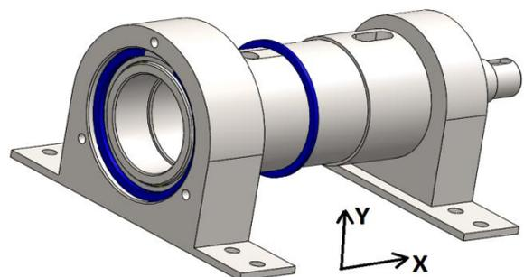
Figure 15: Mounting needle bearing in its casing and shaft
