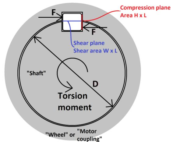
Figure 10: Free body diagram of keys
