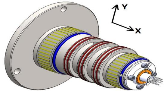
Figure 13: Mounting medium and optical signal supply system
