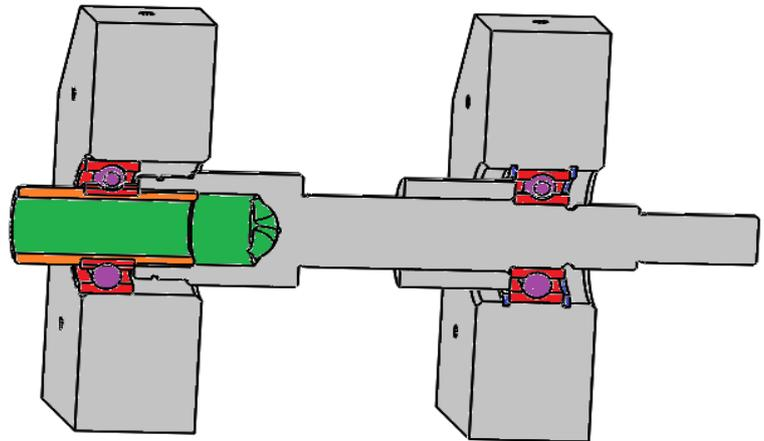
Figure 3: Schematic representation of the old power system. Bearings (red), supporting frame (gray), mix of in- and outflow (green) and closing rings (blue).
