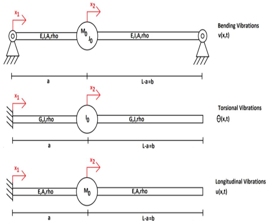
Figure 8: Vibrational model for the power system
