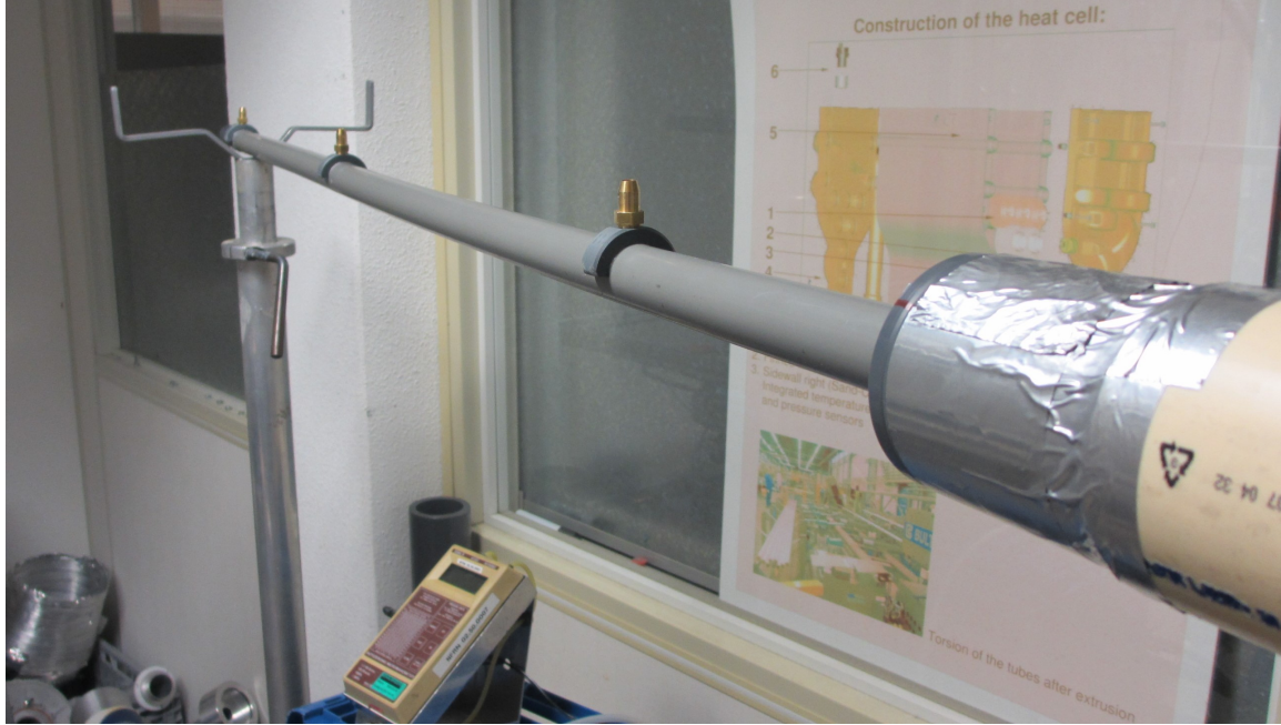
Figure 3.11: PVC pipe with pressure taps connected to the main set-up.
