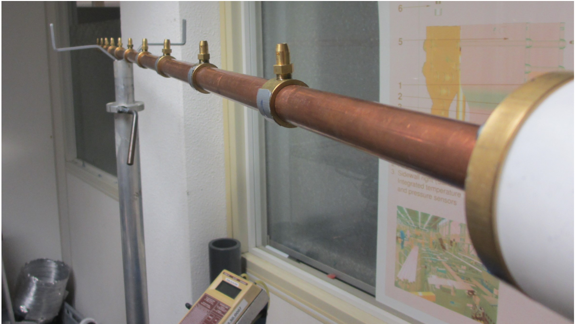
Figure 3.13: Copper pipe with pressure taps connected to the main set-up.
