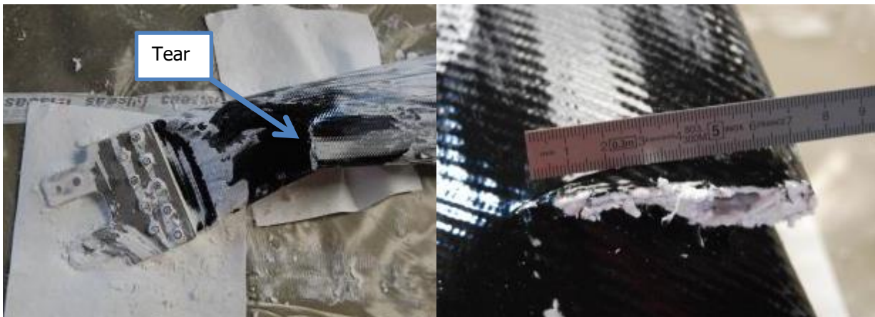
Figure 3.3 Left, overview of the tear in buoyancy hose one. Right, details of the tear in buoyancy hose one
