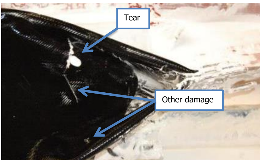
Figure 3.4 Overview of the tear and other damage in buoyancy hose two
