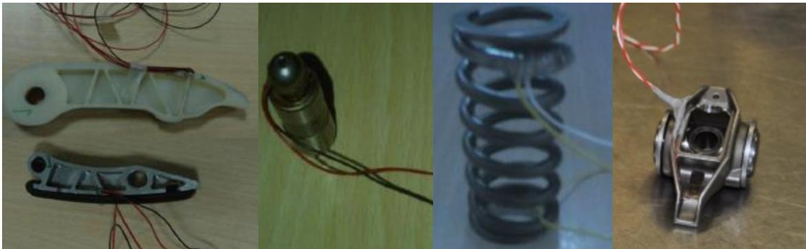
Fig.9-1 Strain gauges 1. Timing chain guides, 2. Lash adjuster, 3. Valve spring, 4. Follower (Mulik, 2015)
