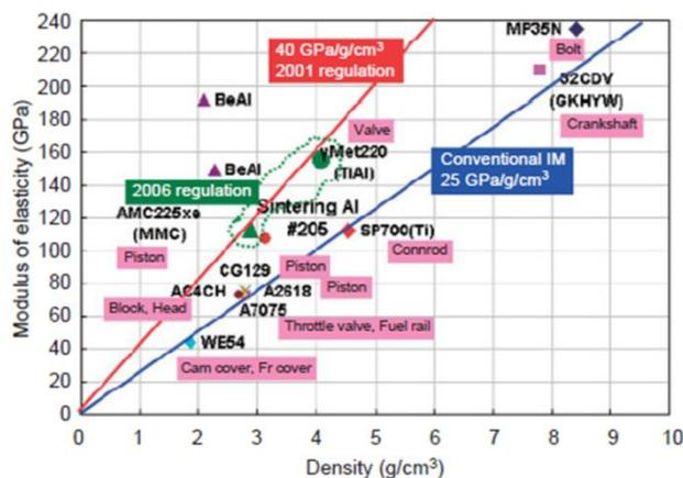
Fig. 3-3 Comparison of multiple materials used in the F1 (Kondo, 2009)
