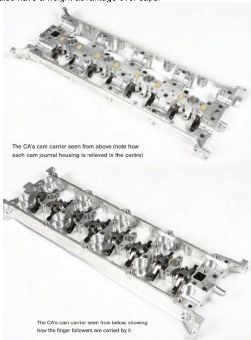
Fig.8-1 The CA's cam carrier (Bamsez, 2013)
