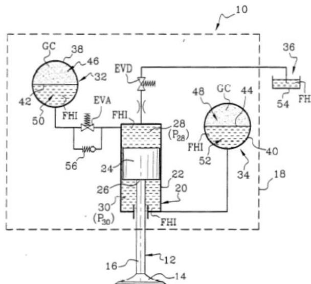
5-3 Renault's hydraulic valve system (Scarborough, 2016)
