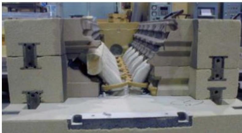
Fig. 8-2 Honda's cylinder head sand mold with PVRS (Kondo, 2009)
