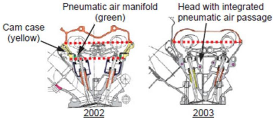
Fig. 5-2 Honda's two and one piece cylinder heads
