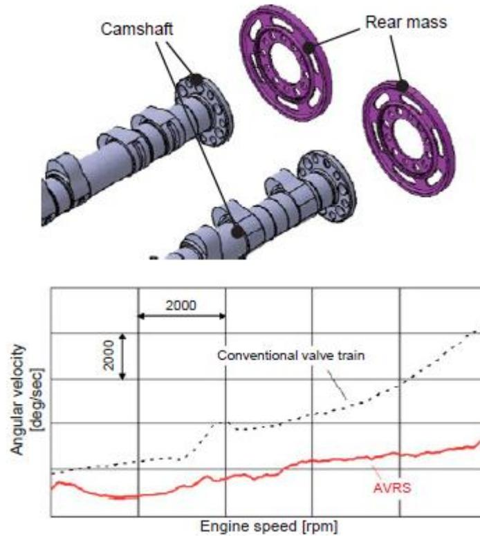
Fig. 4.3 Reduction of the fluctuation of the angular velocity using AVRS (Hayakawa, 2009)
