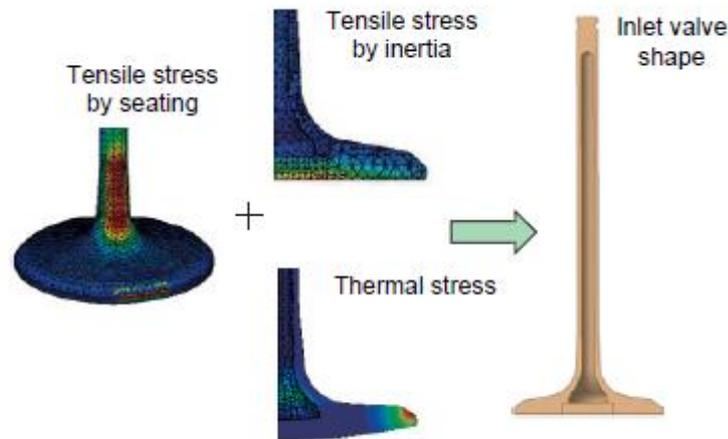
Fig.9-2 Computer aided design of a F1 racing valve (Mulik, 2015)
