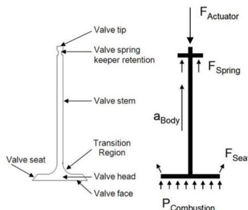
Fig. 3-2 Poppet valve and its free body diagram (Black, 2009)
