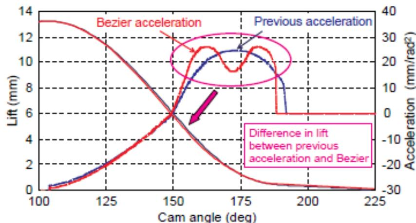
Fig. 4.2 Bezier lift curve of the 2008 Honda F1 engine (Hayakawa, 2009)
