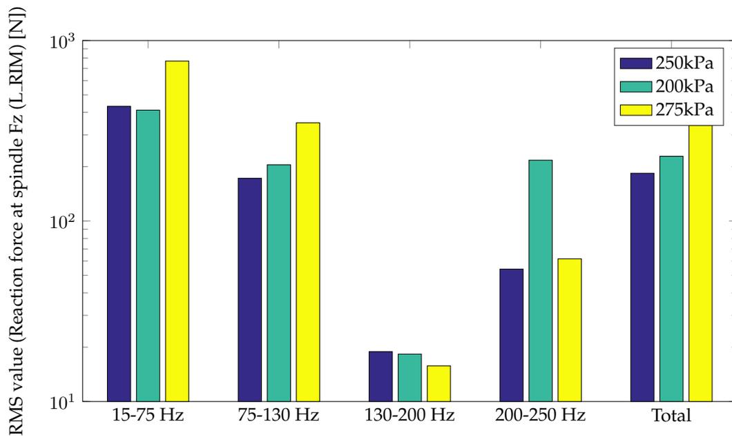
Figure 6.3: Root mean square values of the generic tyre inflation pressure variants.
