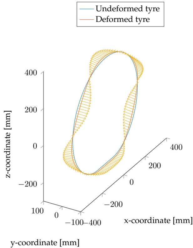
**Figure 5.3:** Visual representation of the coordinate and displacement data of a lateral (3,1) mode shape, which is in this case mode number 14 of a generic tyre. The yellow arrow indicate the direction of the displacements.
