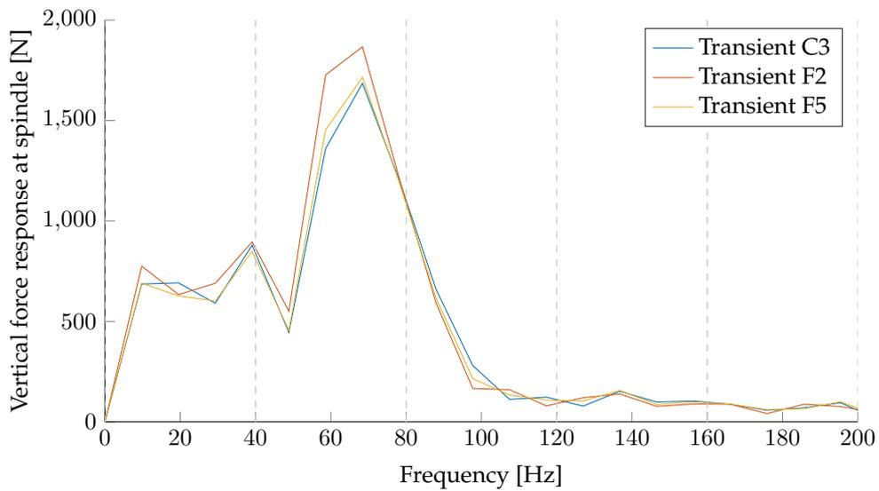
**Figure A.8:** The force frequency response (FRF) data of the three Apollo Alnac 4Gs tyre variants, obtained by transforming the IRF-data using a fast Fourier transform.
