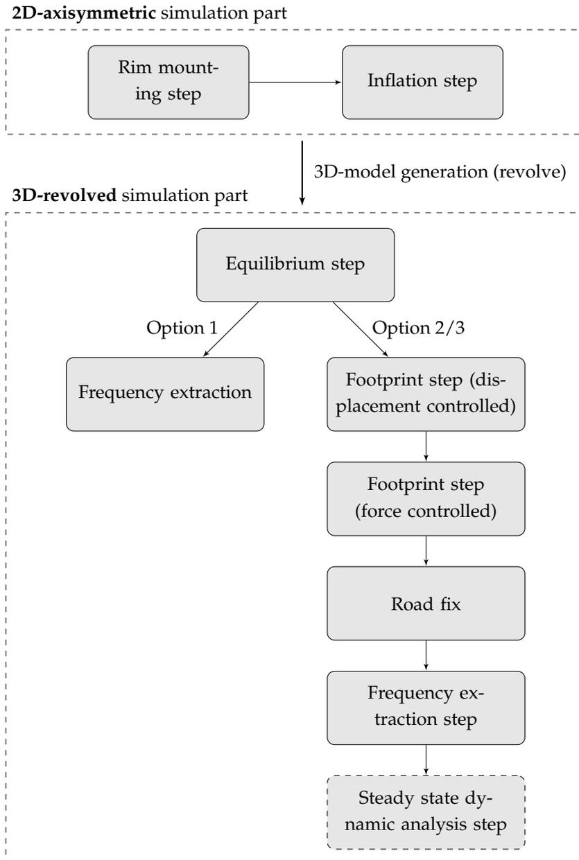
**Figure 4.2:** Overview of low frequency analysis procedure of a tyre with the different options visualized.
