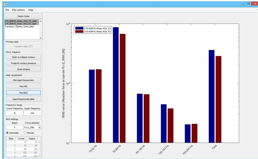
Figure 5.1: Tyre Vibration Toolbox with the RMS plot active.
