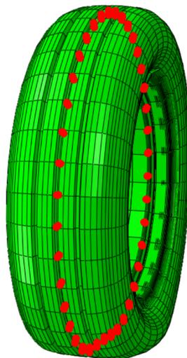
**Figure 5.2:** Symmetry nodes location on a 3D tyre model.
