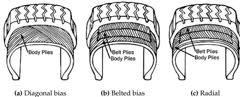
Figure 2.1: Different types of tyre construction.
