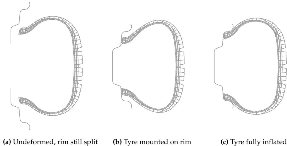
**Figure B.2:** The three 2D simulation steps, with the rim cross-sections on the left.
