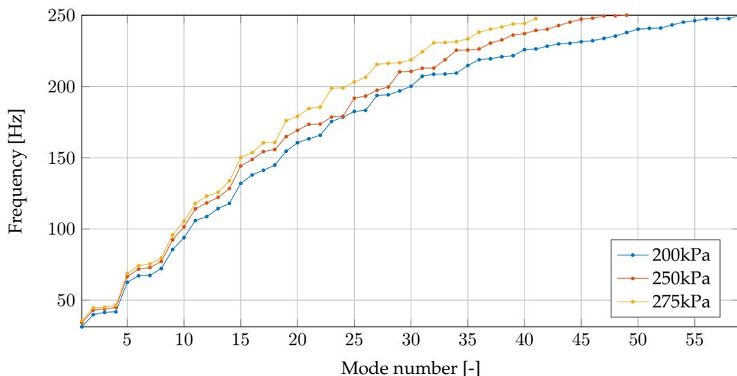
Figure 6.1: Mode numbers vs eigenfrequencies of the generic tyre inflation pressure variants.
