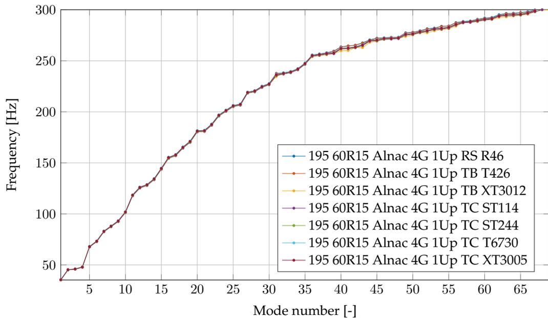
Figure A.1: Mode numbers vs eigenfrequencies of the Apollo Alnac 4G 1 Up tyre variants.
