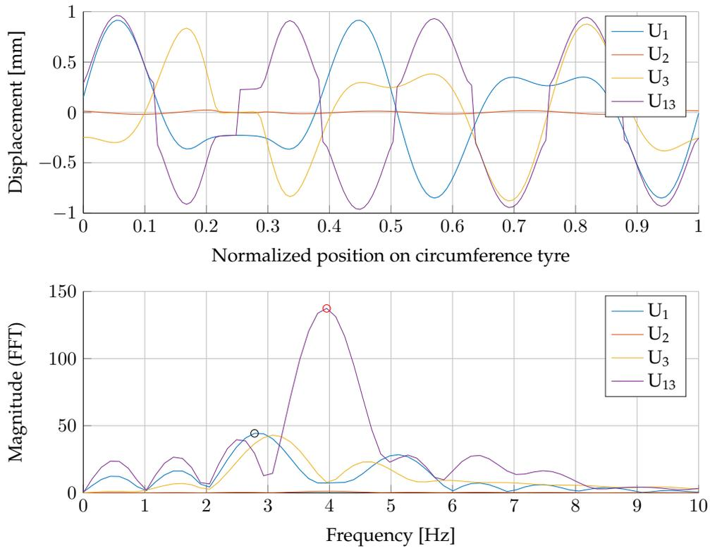
**Figure 5.6:** Raw and processed data from mode number 15. Upper graph displays all the displacements plotted against the normalized position on the tyre's circumference. The lower graph shows the results from the FFT of every displacement data set, where the peak marked with the red circle is the highest apparent peak ( $P_1$ ) and the black circle the second highest peak ( $P_2$ ).
