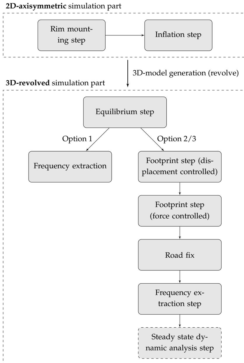
**Figure B.1:** Overview of low frequency analysis procedure of a tyre with the different options visualized.
