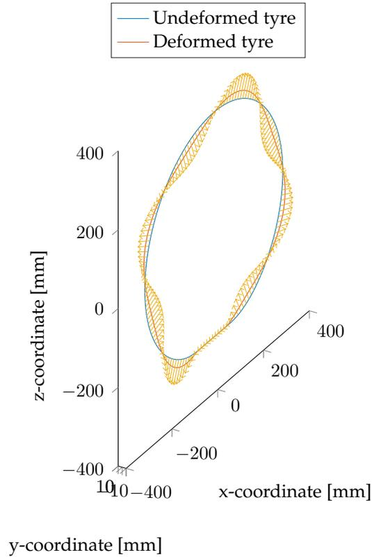
**Figure 5.4:** Visual representation of the coordinate and displacement data of radial (4,0) mode shape, which is in this case mode number 15 of a generic tyre. The yellow arrow indicate the direction of the displacements.
