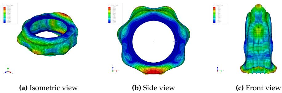
Figure 6.8: Mode shape 27 of the loaded PB12.046A tyre.
