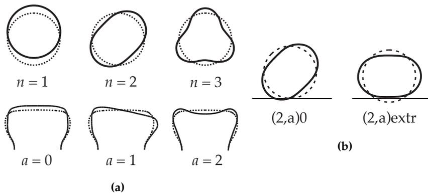
**Figure 4.7:** Visual representation of the mode shape labelling conventions indices (a) as proposed by Wheeler et al. and additions (b) as introduced by Kindt (illustration courtesy of Peter Kindt, obtained from his doctoral dissertation [5].).
