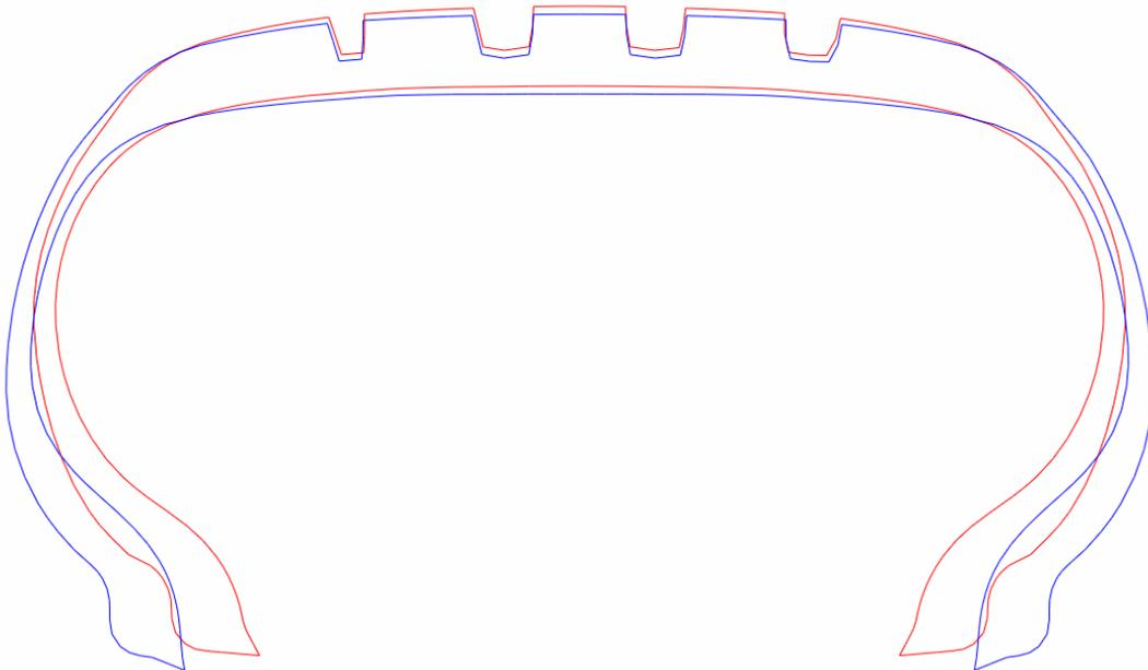
**Figure 4.4:** Mold vs inflated contour (Apollo Alnac 4G 195/60R15).
