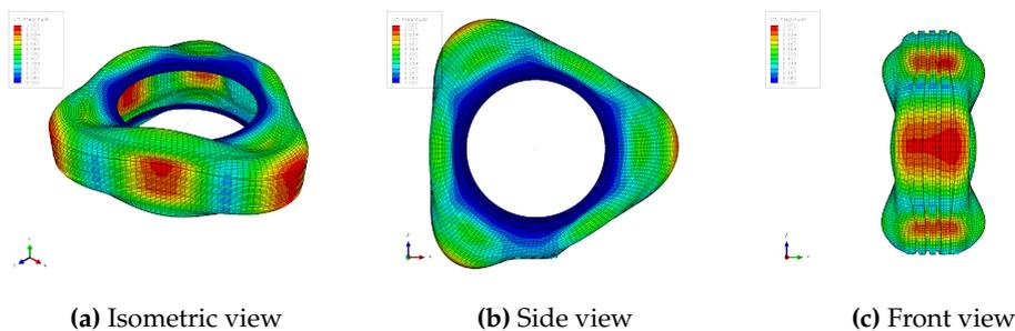
**Figure 4.6:** Mode shape 11 of the Apollo Alnac 4G 195/60R15 tyre, which is a radial mode shape with wavenumber 3.
