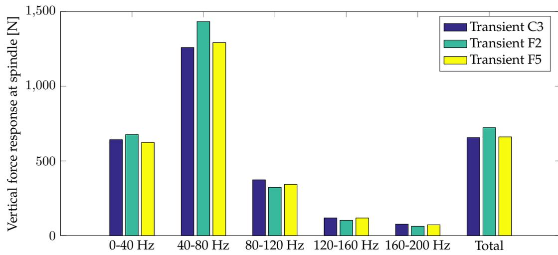
**Figure A.9:** Root mean square values of the FRF-data from figure A.8 of the three Apollo Alnac 4Gs tyre variants (F2, F5 and C3).
