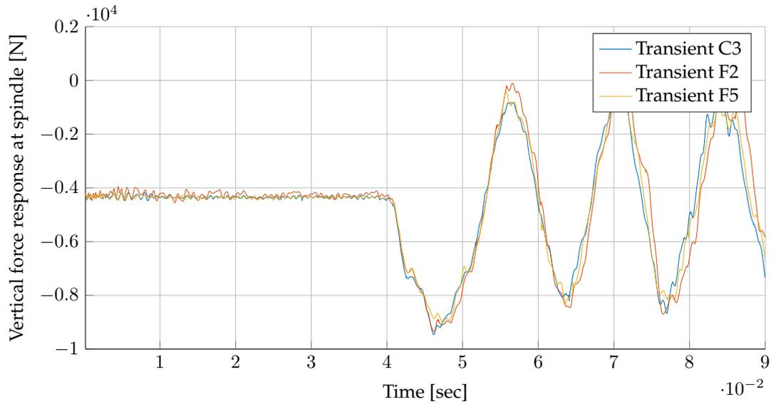
**Figure A.7:** Force impulse response function (IRF) in the time-domain of the three Apollo Alnac 4Gs tyre variants (F2, F5 and C3).
