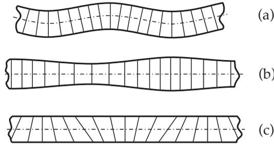
**Figure 3.2:** The three different wave types: bending wave (a), longitudinal wave (b) and rotational wave (c).
