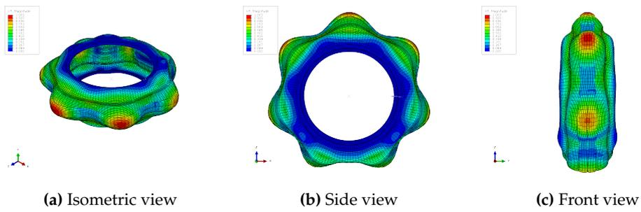
Figure 6.7: Mode shape 24 of the loaded PB12.046A tyre.
