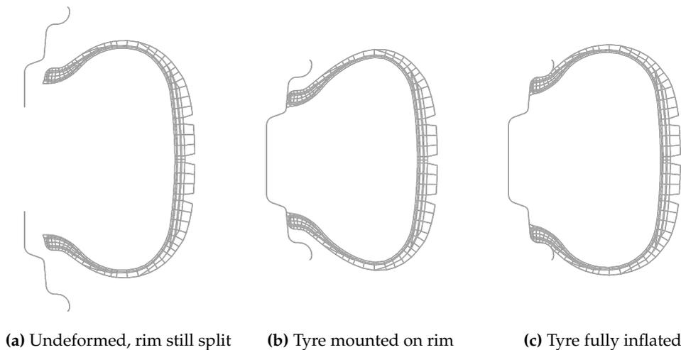
**Figure 4.1:** The three 2D-axisymmetric simulation steps, with the rim cross-sections on the left.
