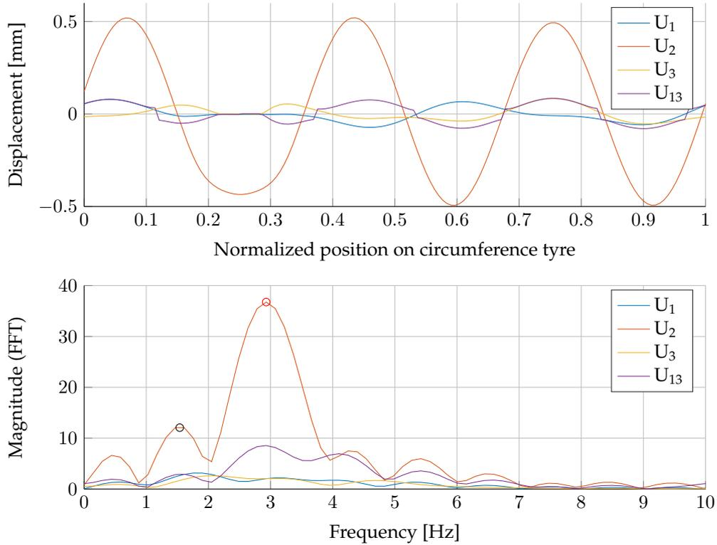
**Figure 5.5:** Raw and processed data from mode number 14. Upper graph displays all the displacements plotted against the normalized position on the tyre's circumference. The lower graph shows the results from the FFT of every displacement data set, where the peak marked with the red circle is the highest apparent peak ( $P_1$ ) and the black circle the second highest peak ( $P_2$ ).
