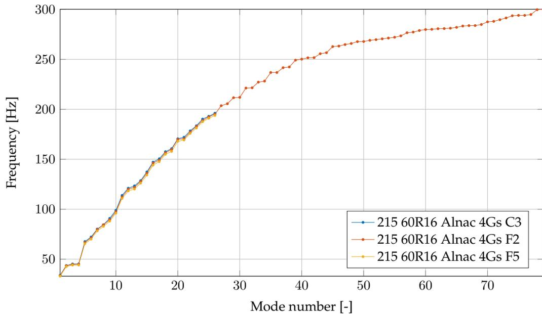
**Figure 6.4:** Mode numbers vs eigenfrequencies of the three Apollo Alnac 4Gs tyre variants.
