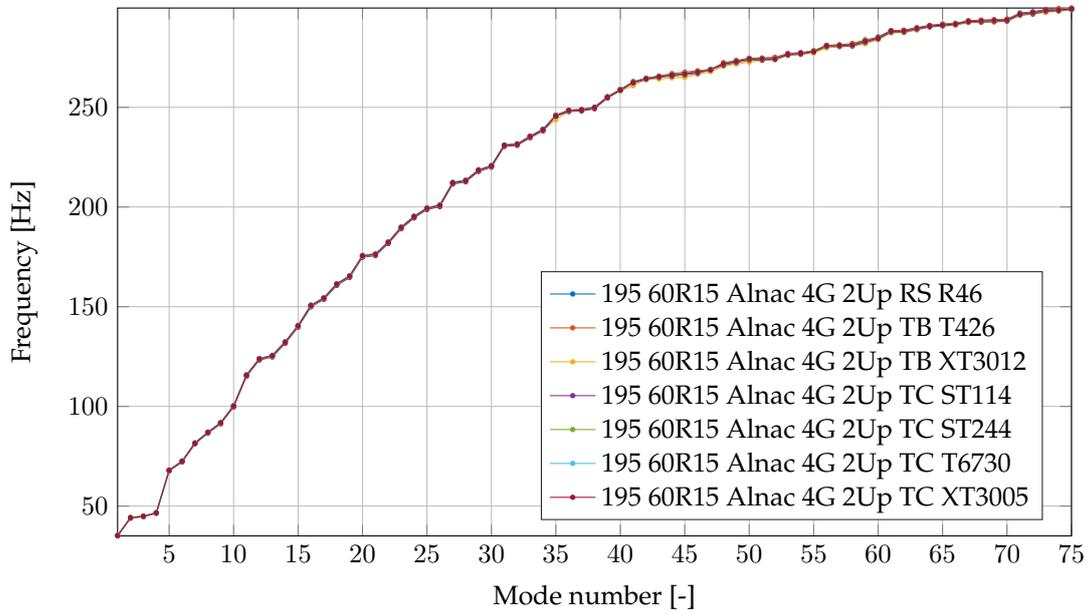
Figure A.4: Mode numbers vs eigenfrequencies of the Apollo Alnac 4G 2 Up tyre variants.
