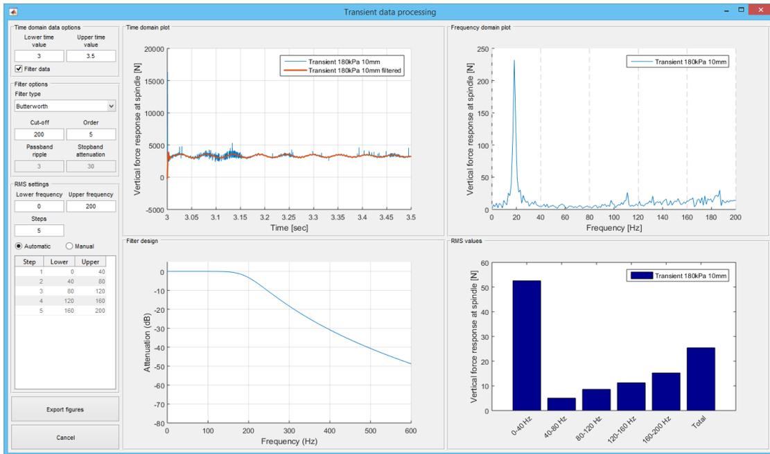
Figure B.11: Transient post-processing window.
