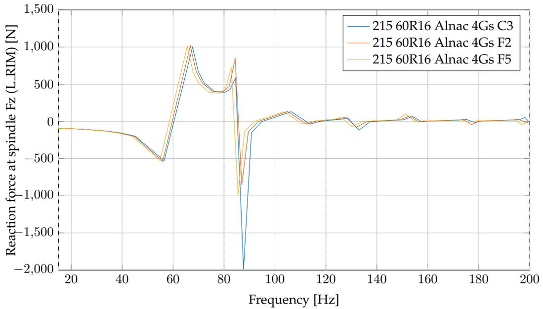
Figure 6.5: Force frequency response function plot of the three Apollo Alnac 4Gs tyre variants.
