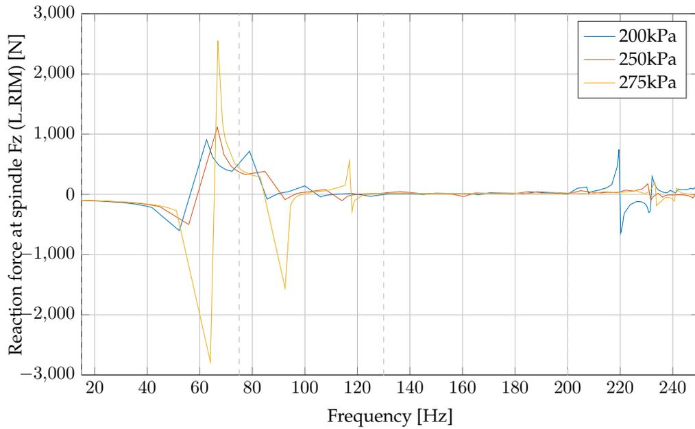
Figure 6.2: Force frequency response function plot of the generic tyre inflation pressure variants.
