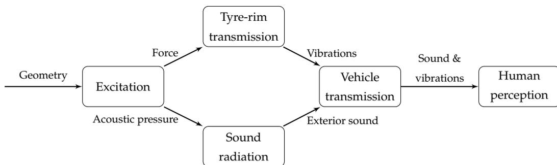
**Figure 3.1:** Basic function network of tyre-road noise as introduced by Bekke [1].
