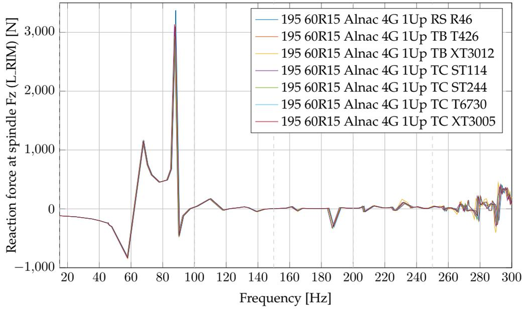
Figure A.2: Force frequency response function plot of the Apollo Alnac 4G 1 Up tyre variants.
