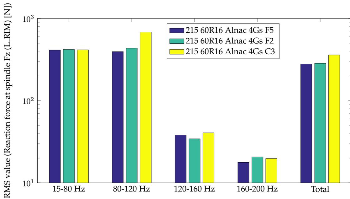
Figure 6.6: Root mean square values of the three Apollo Alnac 4Gs tyre variants.
