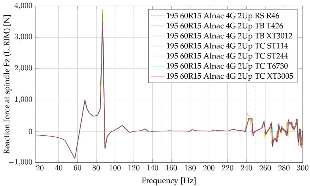
Figure A.5: Force frequency response function plot of the Apollo Alnac 4G 2 Up tyre variants.
