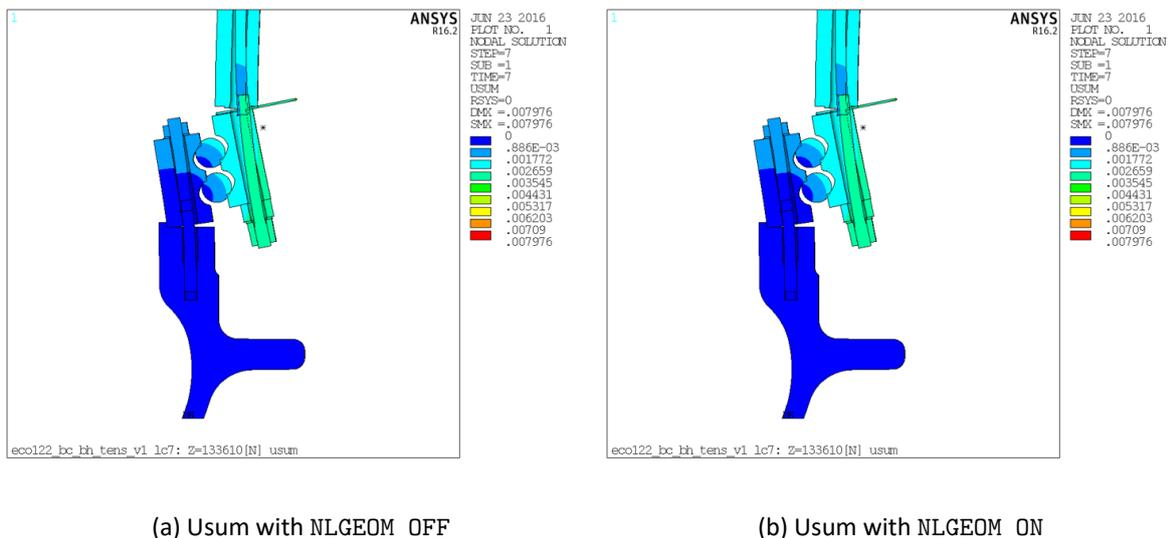
Figure 3.2: Displacements pitch bearing connection
