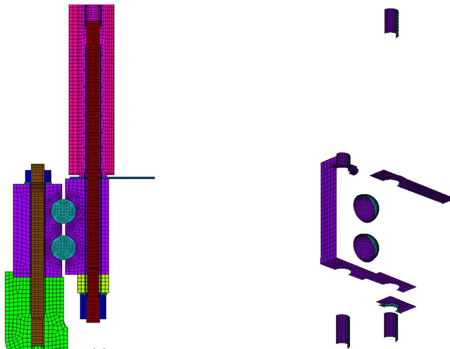
(a) Pitch bearing bolted connection, close up. Frontal view of plane of symmetry (b) Contact interfaces pitch bearing connection. Iso-metric view of plane of symmetry.
