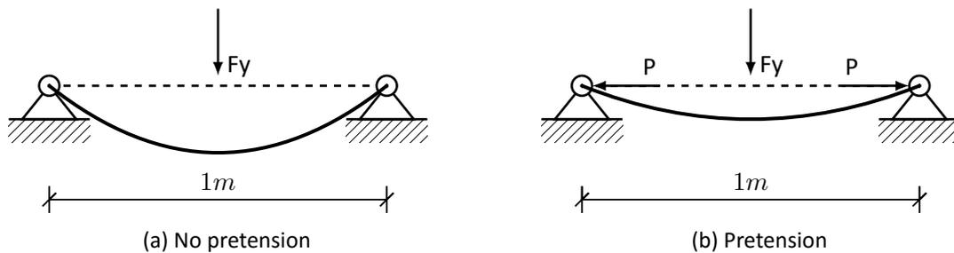
Figure 5.3: Load case 2 to obtain  $K_{flex}$
