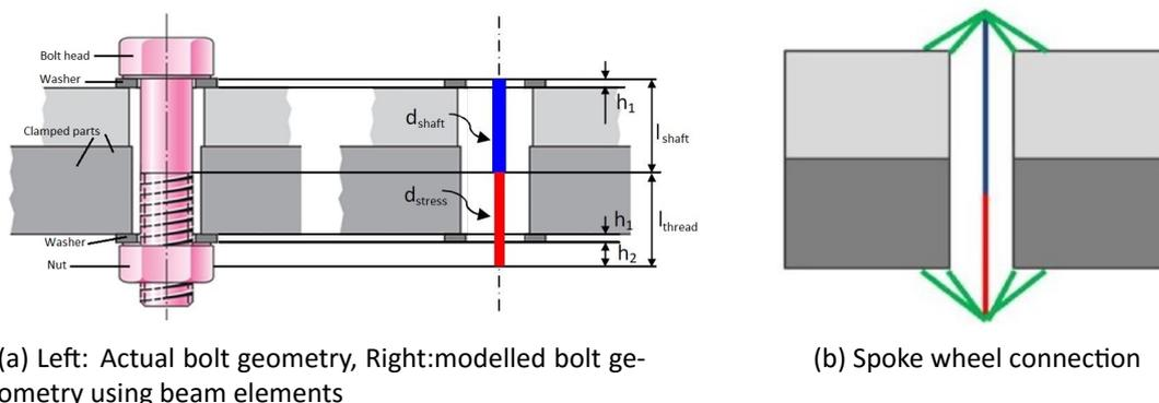
Figure 2.1: FE model of bolted connection
