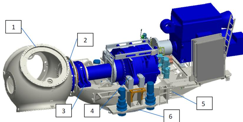
Figure 1.1: Typical bolted connections wind turbine [2]
