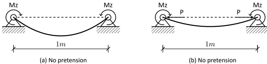
Figure 5.2: Load case 1 to obtain  $K_{rot}$
