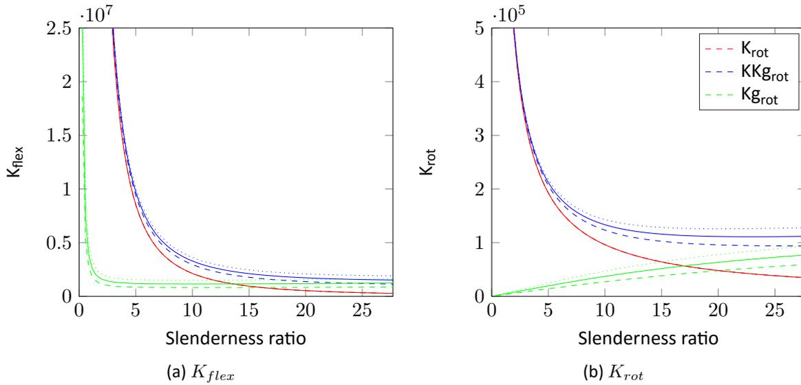
Figure 5.4: Bending stiffness dependent on slenderness ratio.
