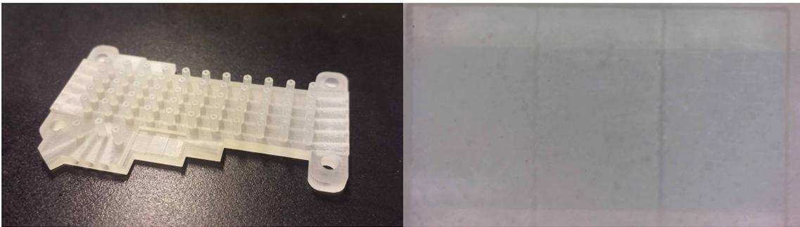
**Figure 6.3:** Overview of the printed part including the membrane (left) and a microscopic close-up of the membrane (right) with the three different thicknesses:  $50\ \mu\text{m}$  (left),  $100\ \mu\text{m}$  (middle), and  $150\ \mu\text{m}$ .
