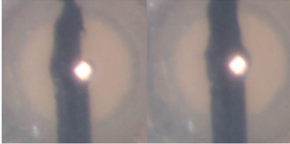
**Figure H.2:** Microscopic images of the channel filling process. The copper wires are not located in the middle of the channel. In the depicted situation the fluid goes around the left side first (left) while a moment later the right side follows (right).
